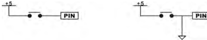
Figure 1-25 Incorrect circuits for button input
