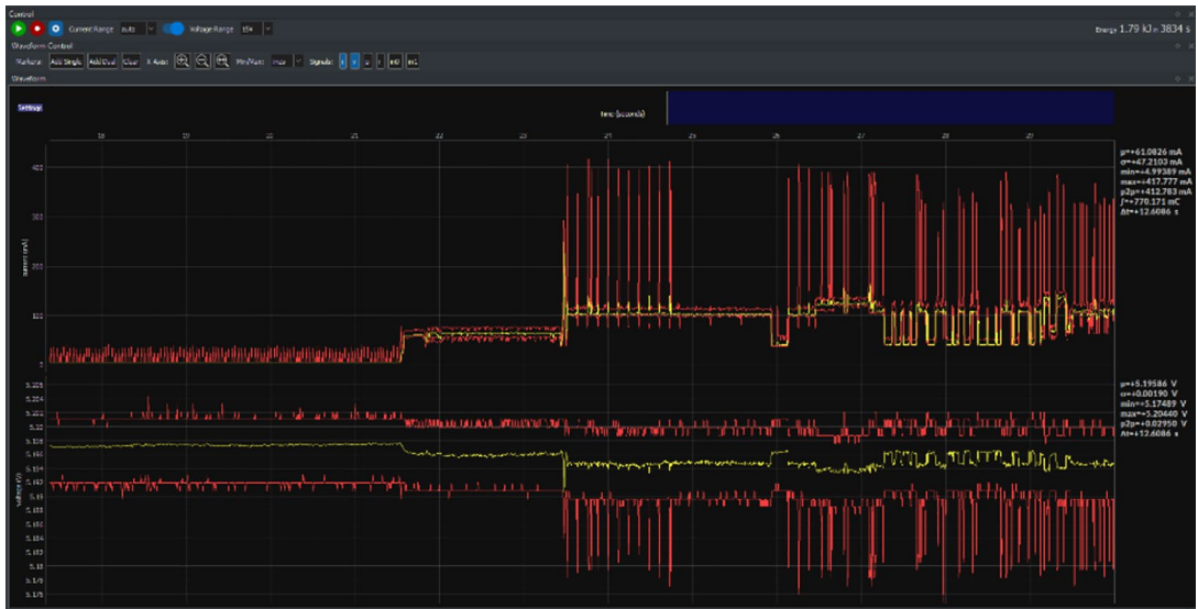
Figure 4-12. 60mA Current Consumption observed during regular operation of the sensor node
