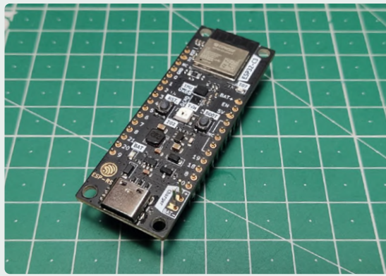
Figure 3: The ESP32-C3 integrates a USB-based debug module with a serial interface, avoiding the need for external probe hardware.
