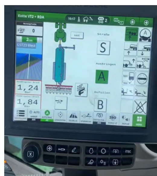
▲ Figure 1: ISOBUS (ISO 11783) user interface on a John Deere monitor. It controls a slurry tanker.
