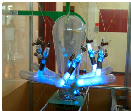
Figure 2: A mercury-arc rectifier. Source: Wikipedia / Timberwind / Public Domain.
