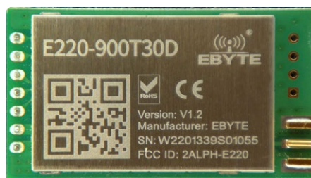
Figure 2: The E220-900T30D module incorporates an 8 dB power amplifier, increasing transmission power to 30 dBm or 1 W.
