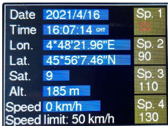
Figure 7: Screen 4 lets you set the speed limits. Here, the first limit, 'Sp. 1', is being set (in red, if you look closely).
