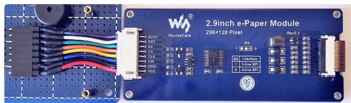
Figure 5: The e-Paper module utilized in the project with its “customized” connector. (Source: Waveshare)
