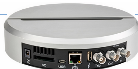
Figure 1: The Moku:Lab has two analog inputs and outputs and features a groove in the top of the housing for use as a tablet stand.
