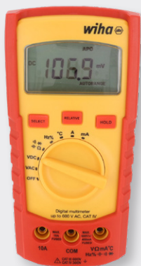
Figure 3: The WIHA.45218 Digital Multimeter can measure voltages in the range of 0 V to 600 V.
