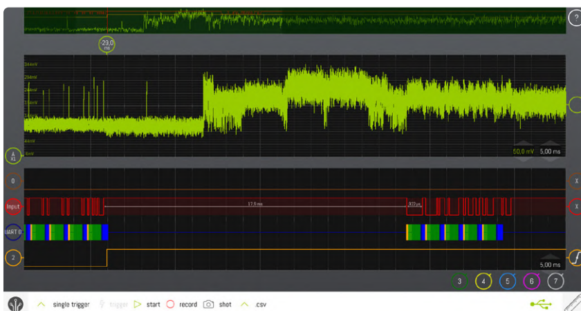
Figure 10: Power supply current (yellow trace) of a bank card when checking an incorrect PIN.
