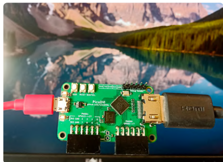
Figure 25: PicoDVI — RP2040 with DVI video output (source: Wren6991 / https://elektor.link/picodviimg ).
