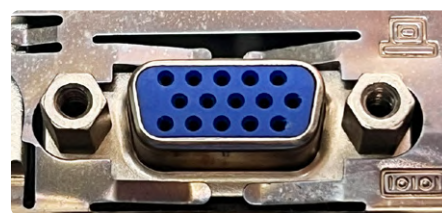
Figure 2: VGA socket on a PC (source: Dr. Thomas Scherer).
