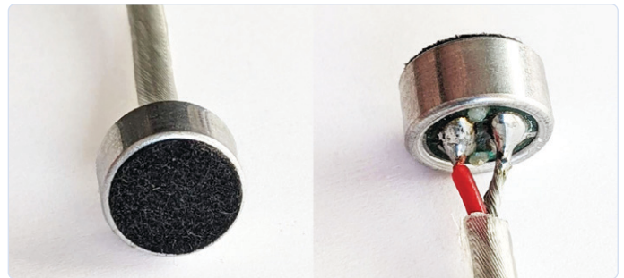
Figure 7: A small electret capsule with a 5 mm membrane.
