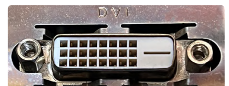
Figure 24: DVI-D socket on a PC (source: Dr. Thomas Scherer).
