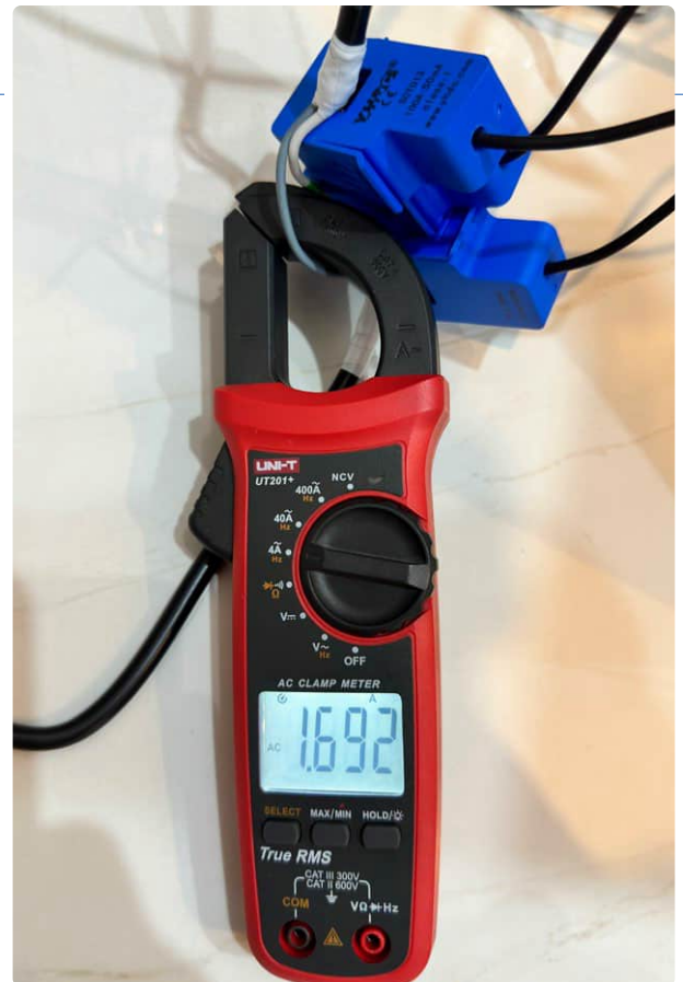
Figure 8: Clamp meter setup for calibration.
