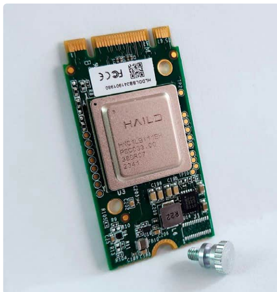
Figure 3: The accelerator board provides a way for the Hailo-8L chip to be connected to a PCIe interface via an M.2 connector.
