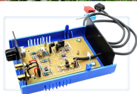
Analog 1-kHz Generator Sine Waves with Low Distortion
