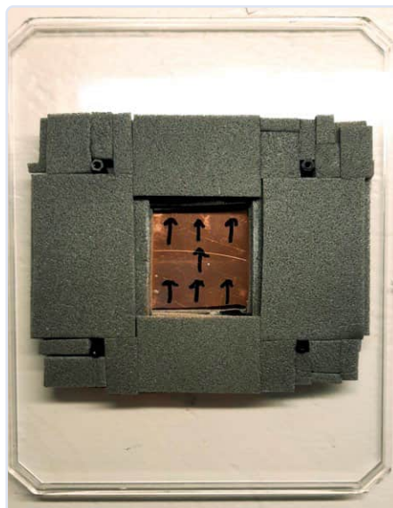
Figure 5: Copper sheet with thermal insulation and plastic standoffs.
