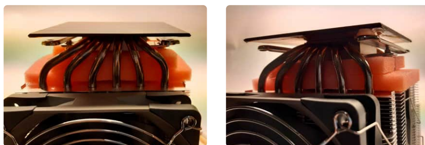
Figure 4: Copper sheet on top of the CPU cooler.
