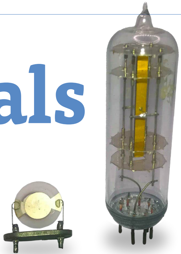
Figure 1: A small 1975 PCB-mount disc crystal of a few MHz with the cover removed, and a larger bar crystal — 100 kHz — from 1959.
