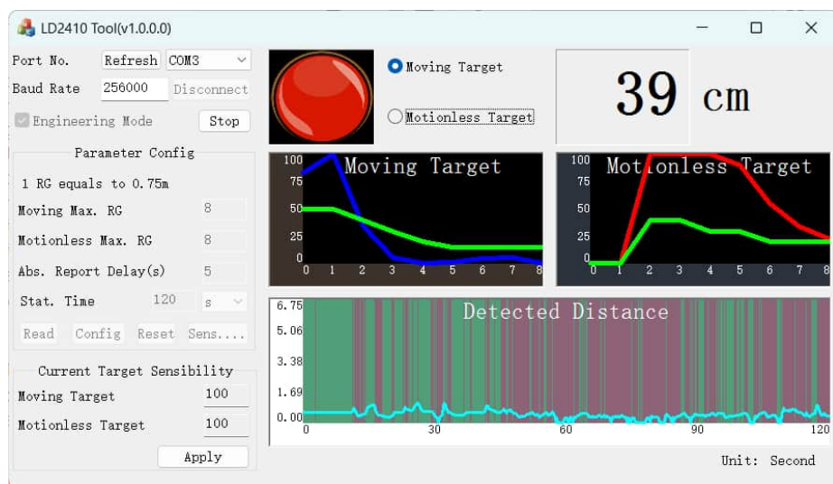
Figure 5: Use LD2410 Tool to configure the radar.
