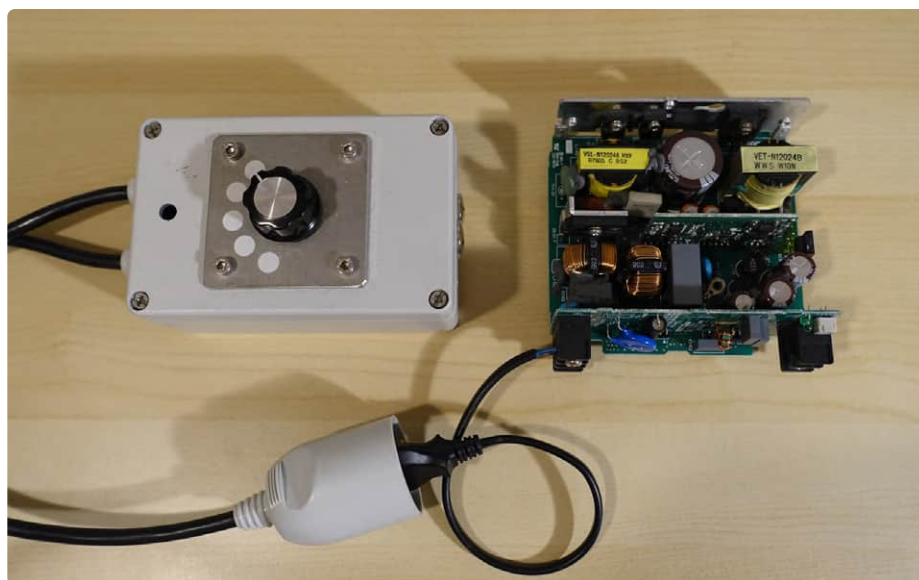
Figure 2: A home-made current limiter.
