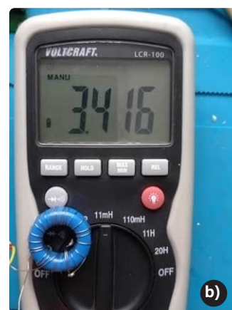
Figure 10: a) Measurements obtained with this project (left), and b) using a commercial inductance meter (right).
