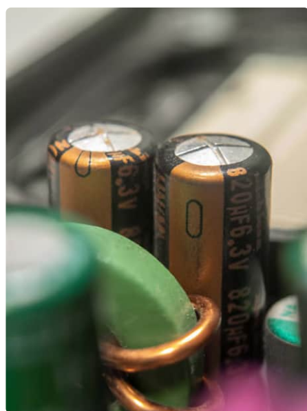
Figure 4: The infamous bulging electrolytic capacitors. (Source: Wikipedia [3])
