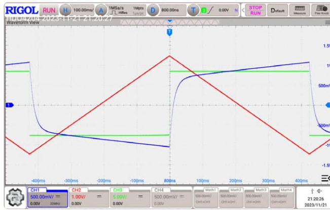
Figure 8: The raw voltage trace (blue) shows the jump transient of finite time at slope reversals.
