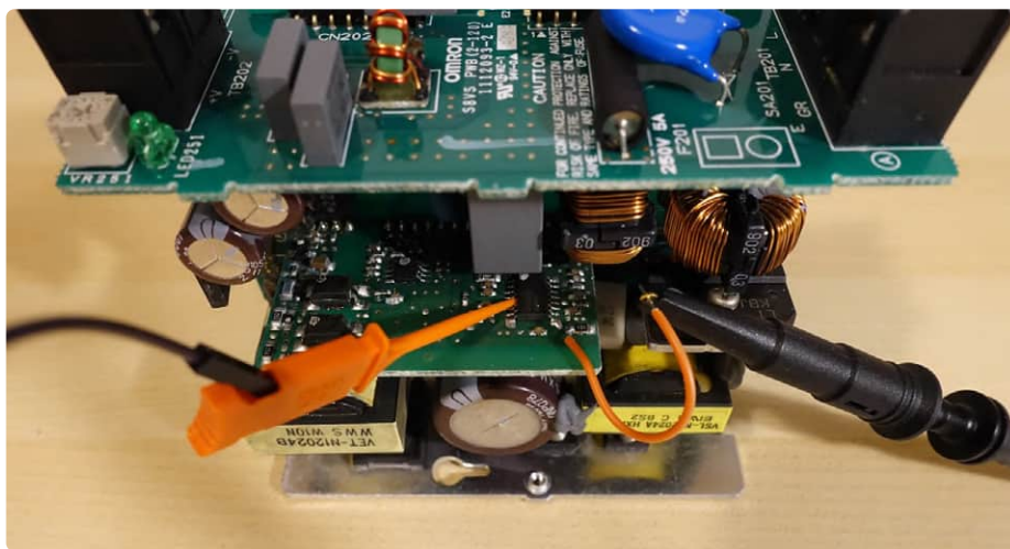
Figure 3: How to safely probe circuits for live testing.
