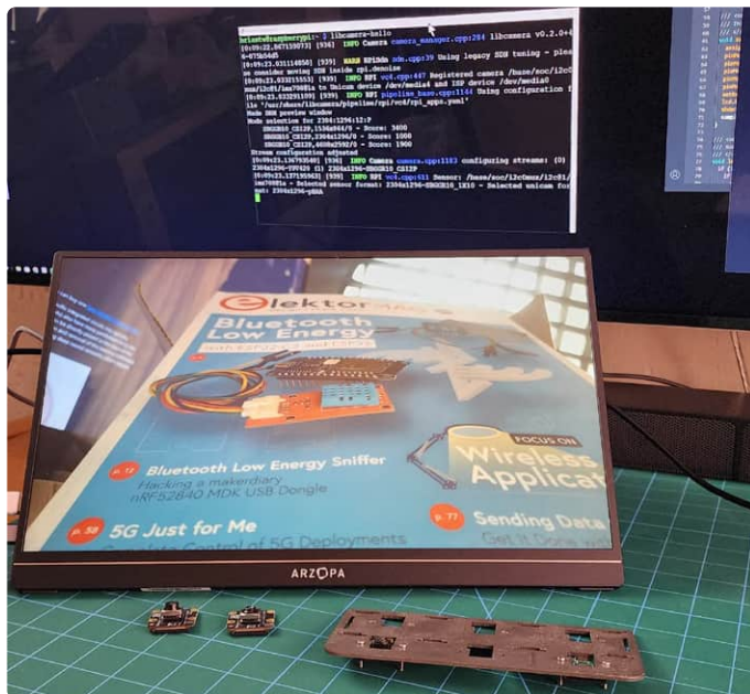
Figure 2: libcamera-hello tells us our camera is working.
