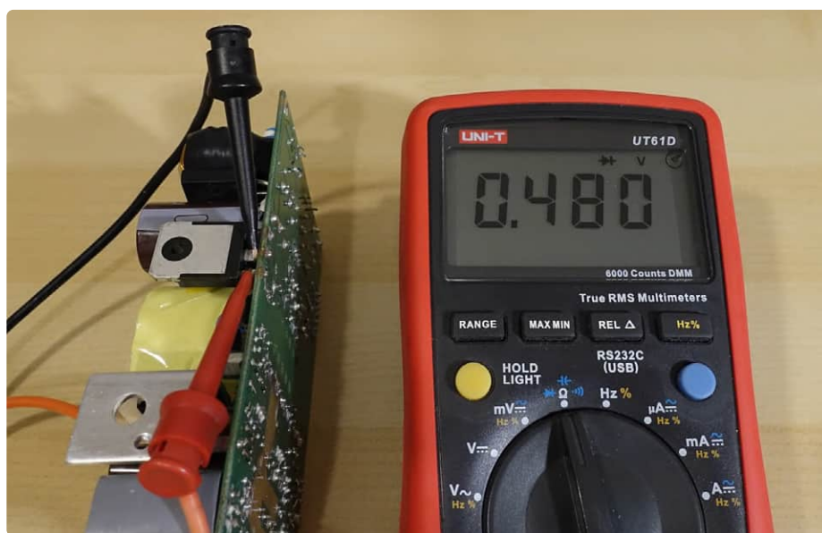
Figure 5: Using the diode mode to test a power MOSFET.
