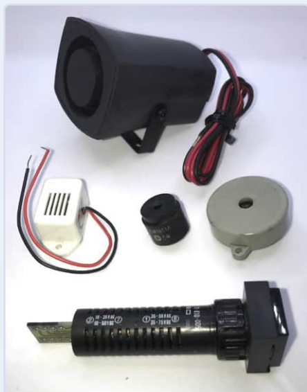
Figure 3: A selection of piezo buzzers (beepers). These have electronics inside to drive the element. Back: A 12 V Piezo siren. Middle: Three different piezo buzzers. Front: a multi-voltage, AC/DC piezo buzzer for industrial switchboard panel use.
