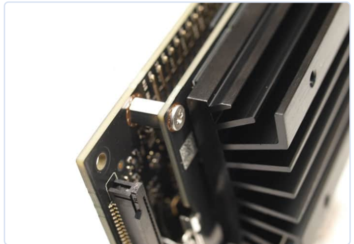
Figure 3: If you loosen the two screws, you can take your developer kit apart.
