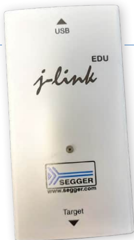
Figure 3: In many (but not all) situations, a JTAG or SWD programmer/debug pod is required for your Zephyr experiments.
