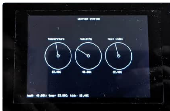
Figure 1: The ESP32 Terminal in its black enclosure showing weather data.
