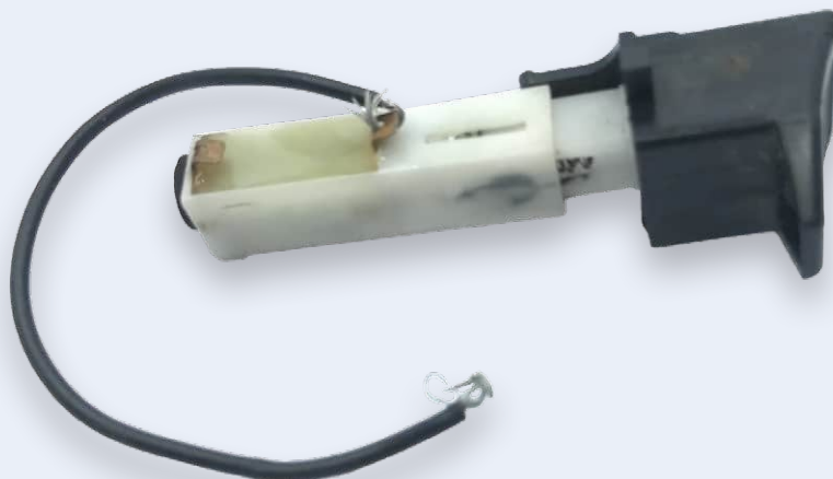
Figure 4: A piezo igniter out of a gas lighter. Press the button at the end, and it will “click” and generate a high voltage pulse to produce a spark across two electrodes.
