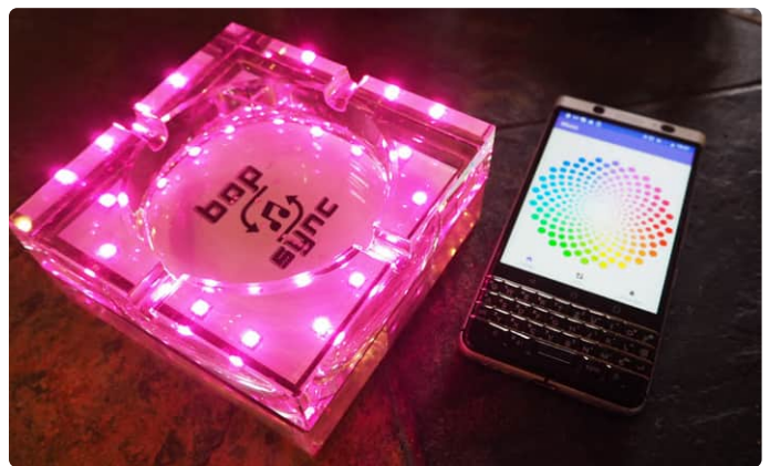
The BopSync ash tray, developed by Icy Beats LLC, uses a Bluetooth LE interface for control.
