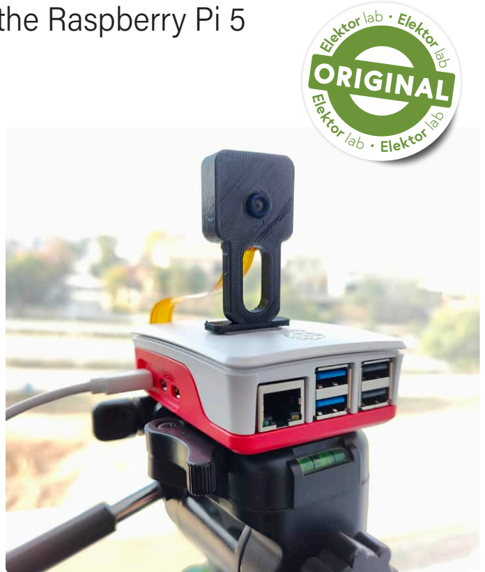
Figure 1: CaptureCount running on a Raspberry Pi 5 with the Raspberry Pi Camera Module 3 (Wide).
