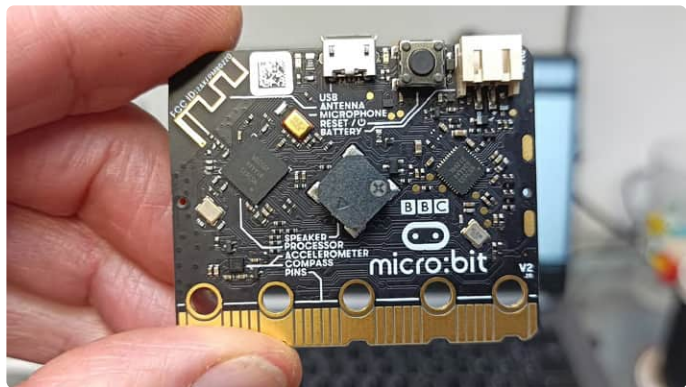
Figure 1: The tiny BBC micro:bit board is an excellent target for trying out the Zephyr RTOS. Who would have thought that this little board intended for teaching programming to 10-year-olds using MakeCode, a Scratch-like graphical language, would also be a super tool for seasoned embedded software developers interested in learning an industrial-grade, real-time operating system?
