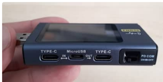
Figure 2: Some of the input/output connectors and the PD safety switch.
