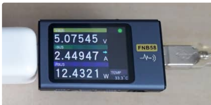
Figure 1: The FNB58 USB meter.
