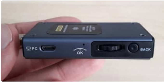
Figure 3: Buttons and PC connection.
