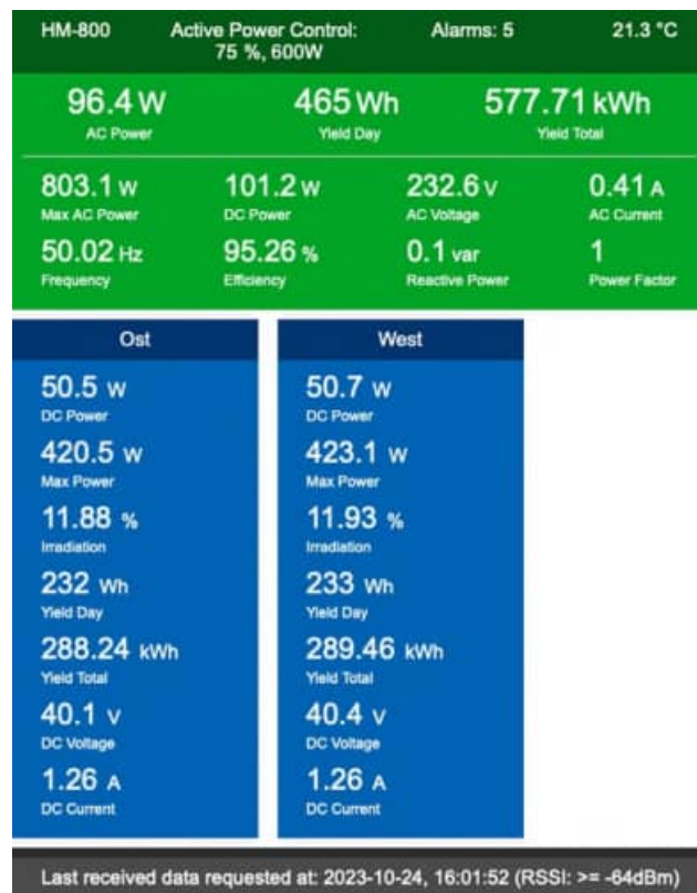
Figure 5: At the end of October, my new balcony power station produced less than 100 W under cloudy skies.
