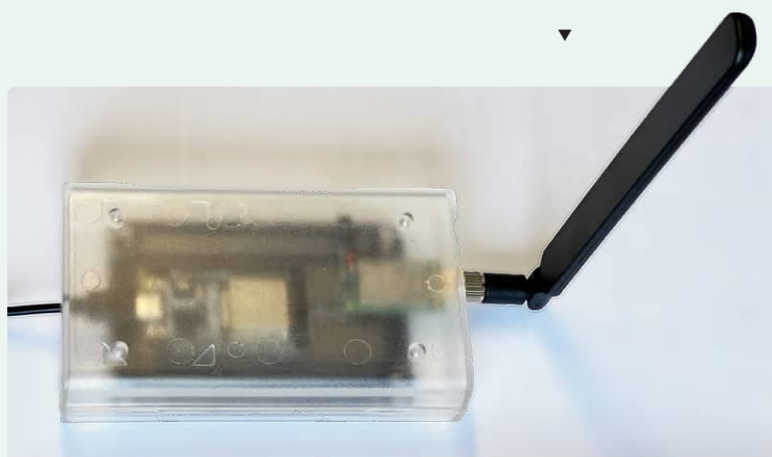
Figure 10: The first prototype (without display) built into a semi-transparent case with an external 2.4 GHz antenna.
