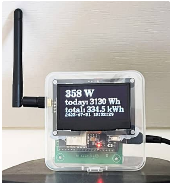
Figure 11: My self-built DTU with a 2.42" OLED display.
