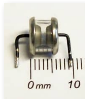
Figure 6: Gas-discharge surge suppressor. Source: https://commons.wikimedia.org/wiki/File:Gasableiter.jpg
