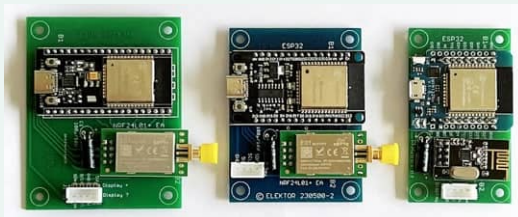
Figure 12: Completed boards. The one for the ESP32 BoB with 38 pins is still a beta version.
