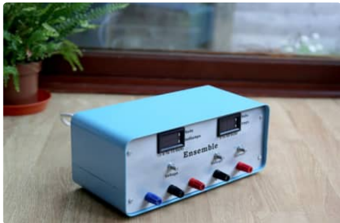
Figure 10: The completed power supply ready for the coming 40 years.
