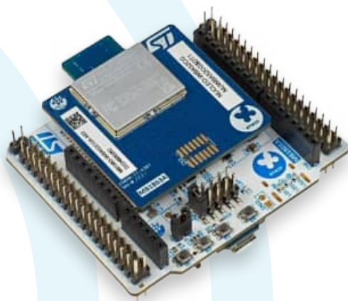
Figure 1: The actual radio chipset sits on a carrier board...
