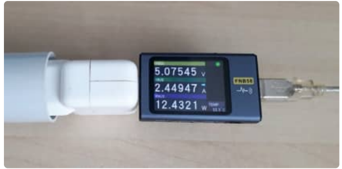
Figure 4: An Apple 2.4 A charger under load.
