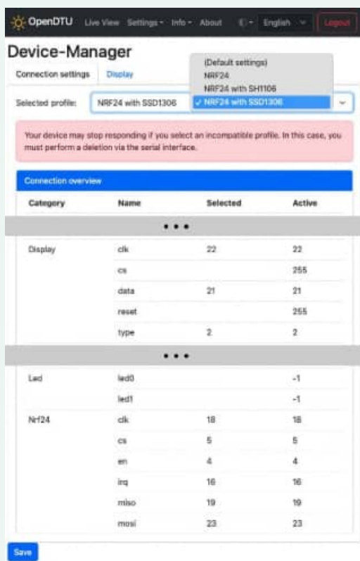
Figure 20: By means of a file with profiles, the assignment of the I/O ports to connected devices can be specified. Here the radio module and the display are of interest.
