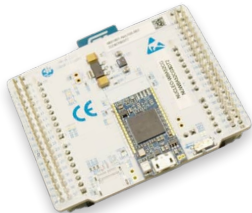
Figure 2: ...while the Arduino connector and the debugger are provided via a separate circuit board.
