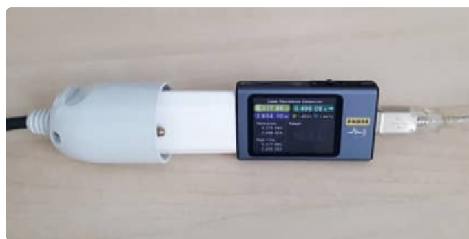
Figure 6: Calibration of the "Resistance Measurement" mode.
