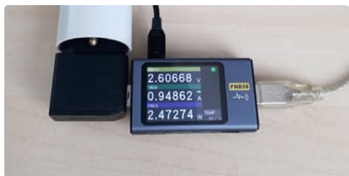
Figure 5: A cheap 1 A charger... Oops!
