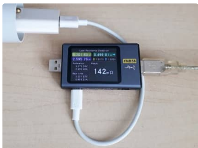
Figure 7: Adding a cable between the charger and the FNB58.
