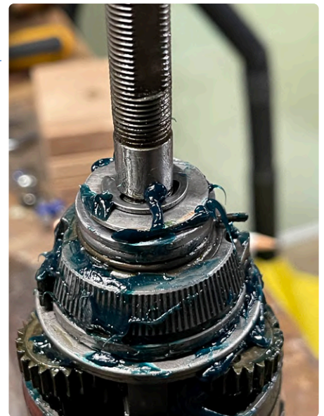
Figure 6: The inner mechanism of a seven-speed gear hub, regreased after removing the back-pedal brake.
