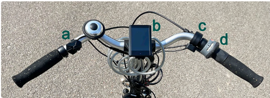
Figure 9: New handlebar fittings: (a) control buttons, (b) display, (c) thumb throttle (start assistance), and (d) shift grip before conversion to the Inter-5E.
