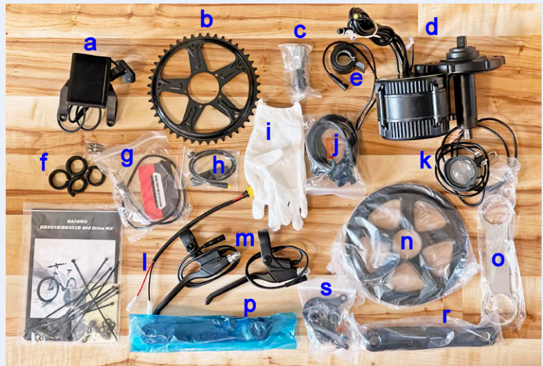
Figure 3: The scope of delivery excluding the battery: (a) display with mount, (b) chainring, (c) crank arm puller, (d) motor, (e) thumb throttle, (f) left spacer ring, (g) USB/TTL adapter, (h) gear shift sensor, (i) gloves, (j) cable harness, (k) LED headlamp, (l) battery connector, (m) brake levers, (n) chainring guard, (o) crankset bearing wrench, (p) left crank arm, (r) right crank arm, and (s) motor mount.
