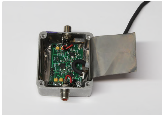
Figure 5: The PCB sandwich installed in an aluminium enclosure.
