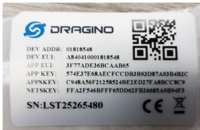
Figure 2: EUIs and software keys for the LHT65.
