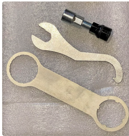
Figure 5: The crank arm puller at the top and the wrench at the bottom were included in the scope of delivery. I had to order the locking wrench in the middle separately.
