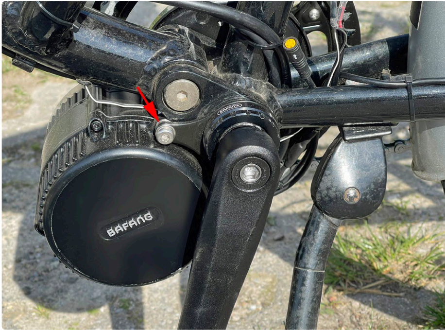
Figure 8: Motor and left mount. My bottom bracket was 70 mm wide, so the mount needed stainless steel washers (arrow) with 6 mm holes.
