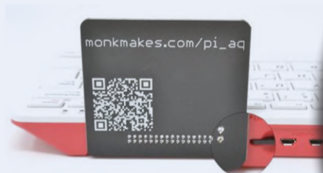
Figure 2: Air Quality Kit connected to a Raspberry Pi 400. (Source: MonkMakes)
