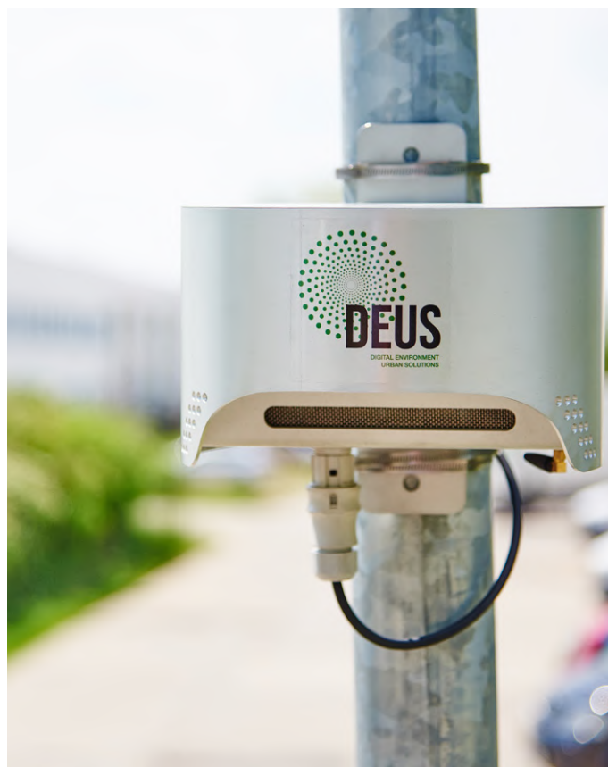
Figure 5: DEUS POLLUTRACK particulate matter sensors gather data from stationary and mobile IoT units. Data is delivered to the back-end using 4G and 5G cellular networks. (Source: DEUS POLLUTRACK)
