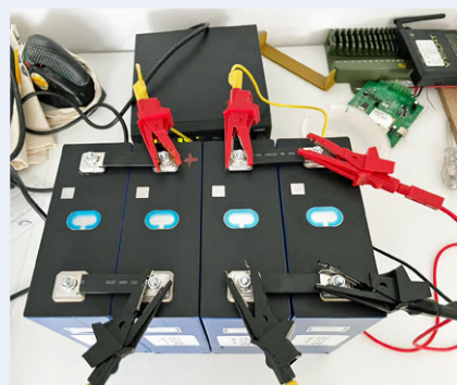
Figure 8: LiFePO 4 batteries under test before installation in Martin's boat. (Source: Martin Jepkens)
