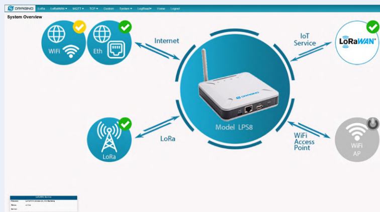
Figure 5: Communication paths available via the LPS8 gateway.
