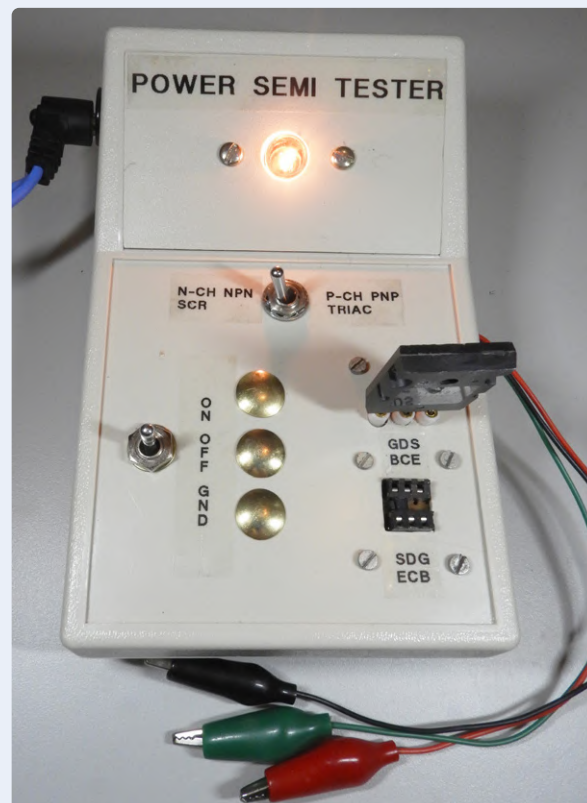
Figure 2: A simple Power Semiconductor Tester tests MOSFETs, transistors, SCRs and Triacs.
