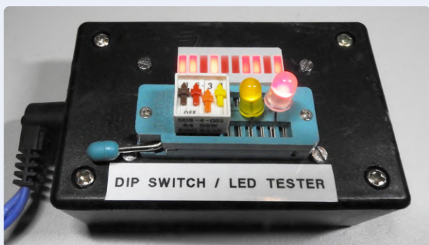
Figure 3: A DIY DIP Switch / LED tester shown testing a 4-way DIP switch and a couple of LEDs.
