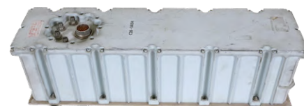
Figure 2: Collins Radio S-Band traveling-wave tube amplifier used for communication with earth during the Apollo mission. (Source: Ken Shirriff)
