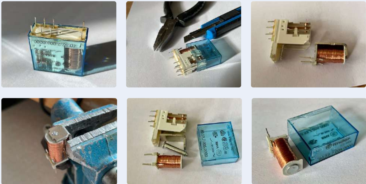
Figure 3: Taking the relay apart and preparing the solenoid.
