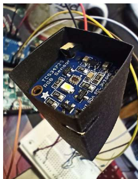
Figure 4: TCS34725 RGB sensor with black card shield fitted.
