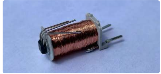
Figure 4: The Hall sensor glued to the iron core of the coil.
