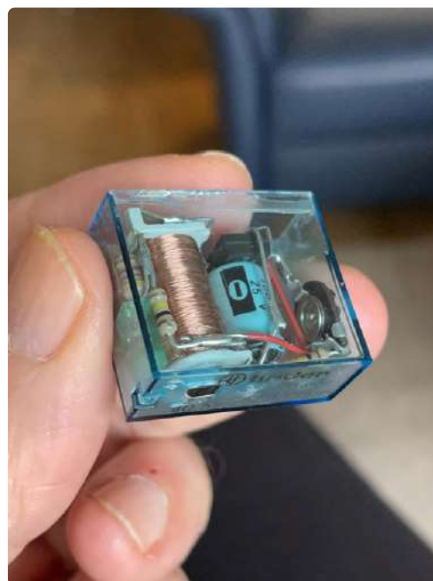
Figure 2: A single turn trimmer plus series resistor also fits into the enclosure.
