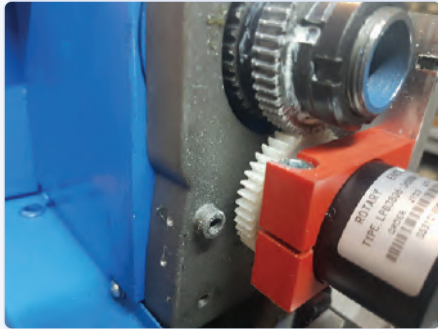
Figure 6: ...and is driven via a gear salvaged from the dismantled gearbox.
