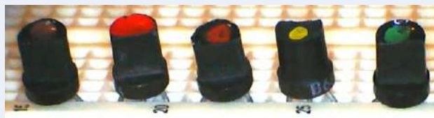
Figure 1: 2N2926 transistors. The colour specifies the transistor gain H_{fe} : Brown 35-70; Red 55-110; Orange 90-180; Yellow 150-300; Green 235-470.
