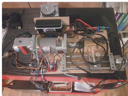
Figure 1: An early prototype with a DC motor as the 'main spindle', a Nema 17 stepping motor for the lead screw and motor control using a simple PWM module.
