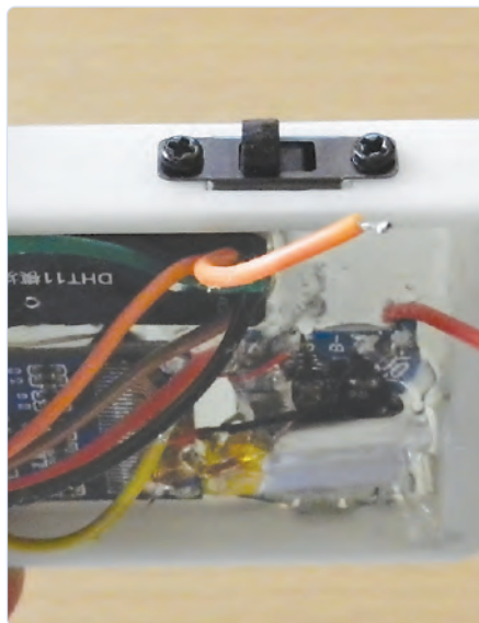
Figure 7: The switch is attached to the outside of the enclosure.
