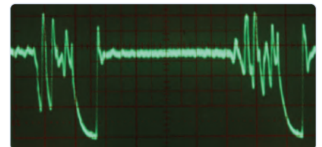
Figure 2: I_{dd} current captured on a vintage Tek 466 'scope while writing bytes 0xDE (left) and 0x01 (right) to SRAM (at 200 ns/div).
