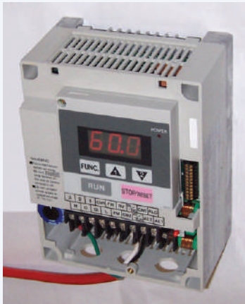
Figure 8: A small variable frequency drive for induction motors rated at a few kilowatts. This electronic switching circuit allows the rotational speed to be set. Larger versions are also available, offering more advanced functions. (Image credit: C. J. Cowie, CC 3.0 [6])
