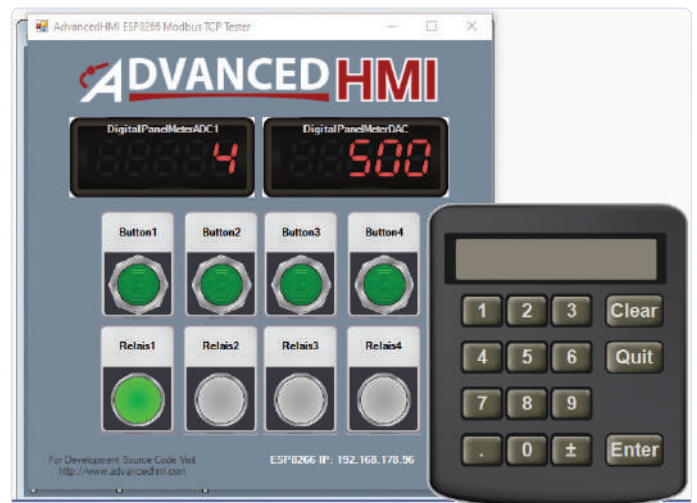
Figure 2: The AdvancedHMI software generates human-machine interface applications.
