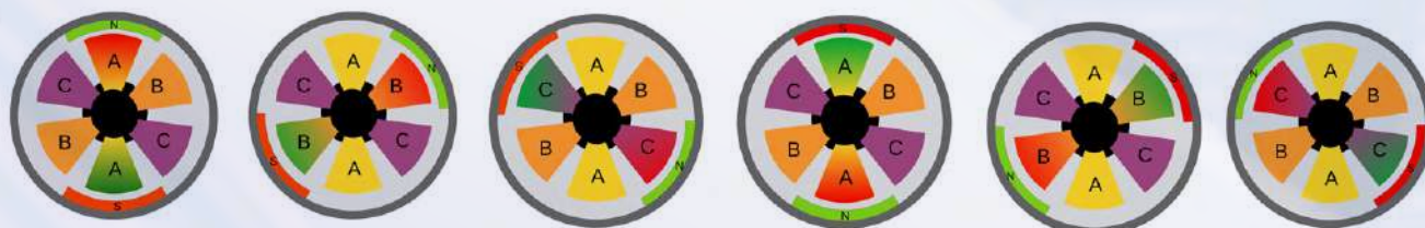
Figure 22: The rotor is pulled by a magnetic field.
