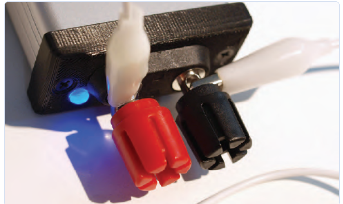
Figure 2: Croc clip power hook up.
