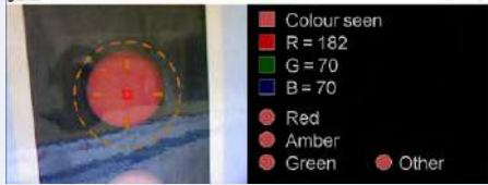
Figure 7: The response of tlight_detect.pde prior to learning any colors.
