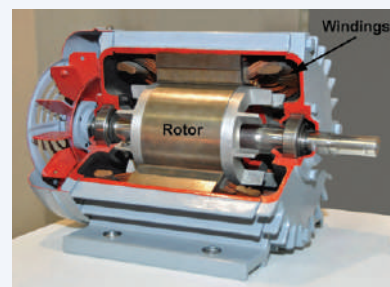
Figure 7: Cut-away induction motor rated in the low kilowatts. The stator windings and the short-circuited rotor can easily be seen. (Image credit: S. J. de Waard, CC 3.0 [5])
