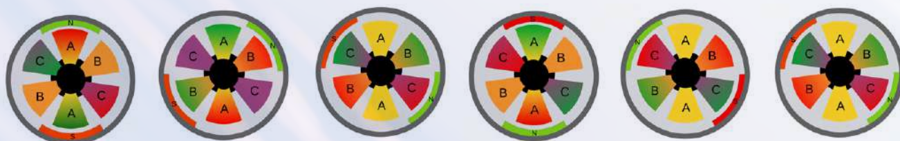
Figure 23: The rotor is driven by two of the three winding pairs.
