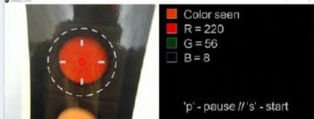
Figure 6: computer_vision.pde provides us with the RGB values the camera 'sees' for each traffic-light color.
