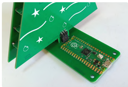
Figure 1: The addressable RGB LEDs of the Wordy Christmas Tree are controlled by a Raspberry Pi Pico board.
