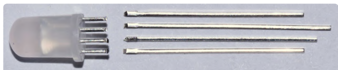
Figure 4: Cut wires. The top wire in the photo is pin 1. The flange is partially missing here.
