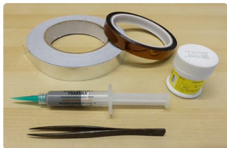
Figure 11: Solder paste and tools to work with hot air.
