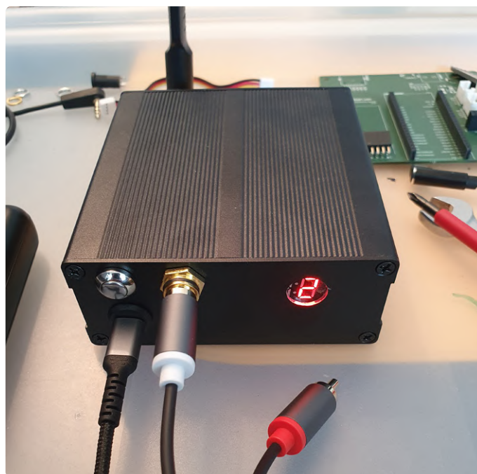
Figure 7: Prototype of the transmitter, with a cinch input, a button to switch the radio channel, and a seven-segment display for showing the radio channel index (0 to 9).
