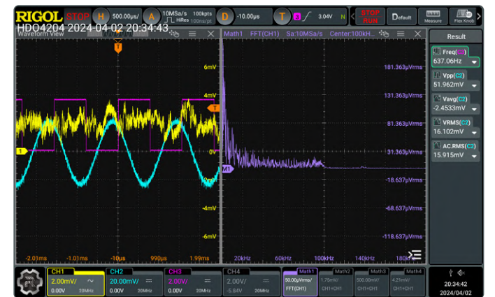
Figure 6: Badly defined signal from the same configuration as shown in Figure 5.
