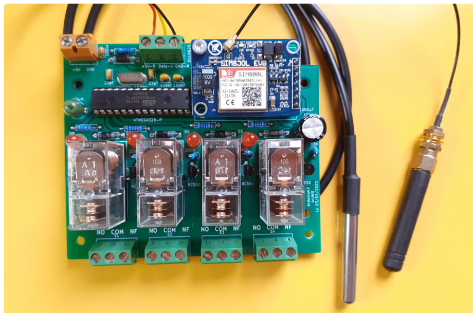
Figure 4: Version allowing remote modem reset, also featuring the more robust encapsulated sensor.
