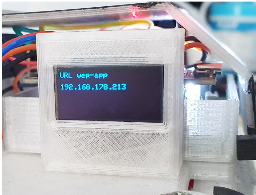
Figure 4: The 0.96" OLED display in a 3D printed housing shows the IP address the ESP32 obtains from the router's DHCP server.
