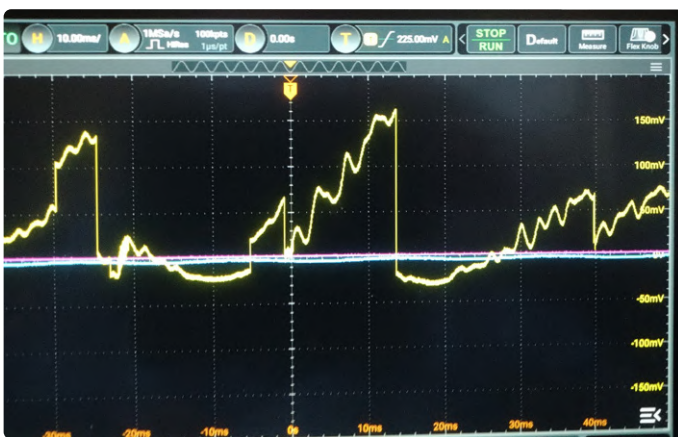
Figure 9: Interferometer signal showing unwanted mode jump effects.
