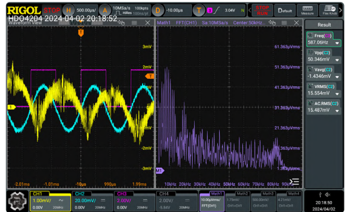
Figure 5: The same signal as shown in Figure 4, but from a different, less ideal setup. The traces exhibit considerable intensity modulation due to dependence of the total reflected intensity on the membrane displacement.
