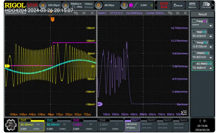
Figure 4: Signal from a vibrating membrane. On the left: CH1 (yellow) shows the amplified photodiode output, CH2 (cyan) the exciter drive voltage ( \Rightarrow synchronization). Right: Fourier transform (FFT) of CH1 showing a typical shape. The high-frequency edge relates to the maximum membrane velocity.
