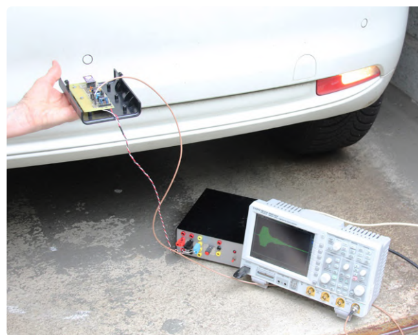
Figure 4: Testing the parking sensors on my son's car. This one worked fine, as you can see on the oscilloscope.
