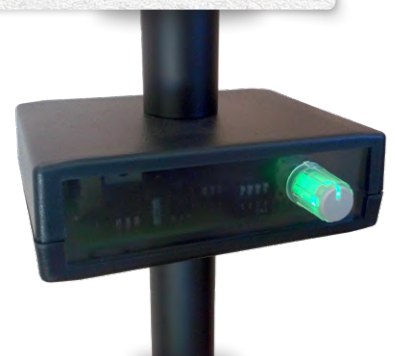
Figure 6: The dimmer unit installed on the lamp post.
