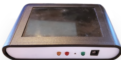
Figure 2: The finished IO-Homecontrol to MQTT adapter.
