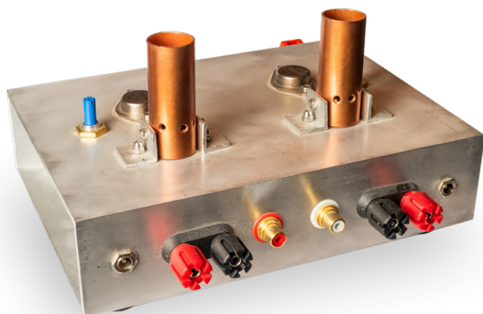
Figure 2: Real amplifiers glow in the dark! A rearview of the Lamp amp, built on a piece of aluminum rectangular profile.
