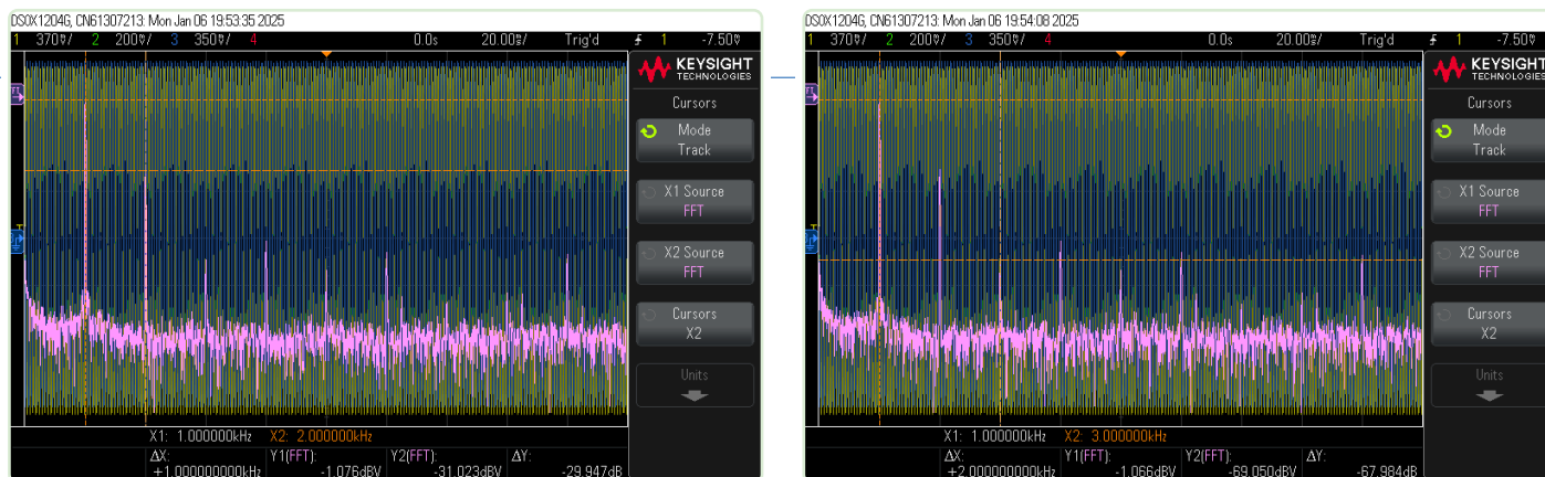
Figure 8: FFT using a 1 kHz sinewave input signal, where CH1 = V_{in} , CH2 = V_{out} , CHM = FFT, with 100 mW on 8 \Omega with feedback, 2 nd harmonic (left) and 3 rd harmonic (right).
