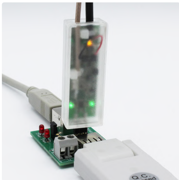
Figure 6: The USB adapter with a high-speed differential probe connected.
