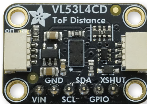
Figure 1: The VL53L4CD sensor on its breakout board.
