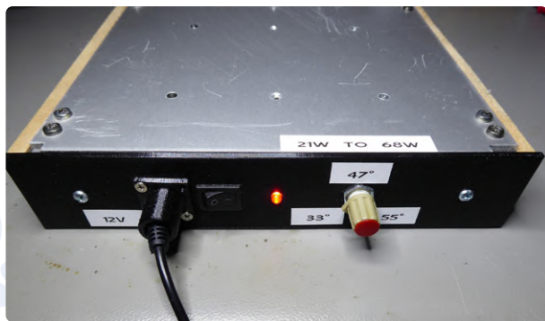
Figure 4: Side view with the adapter plug and knob to set the power. Temperatures are just an indication, since the end temperature is relative to the ambient temperature.
