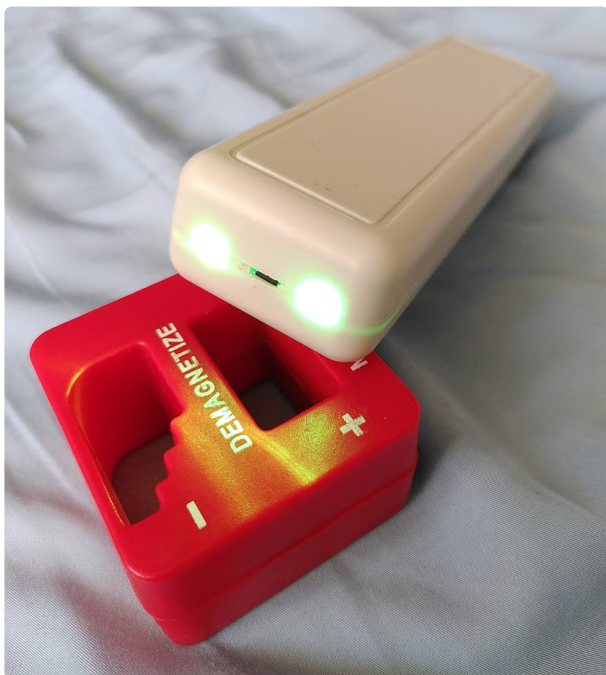
Figure 1: The Magnet Finder in action, here detecting a screwdriver magnetizer.
