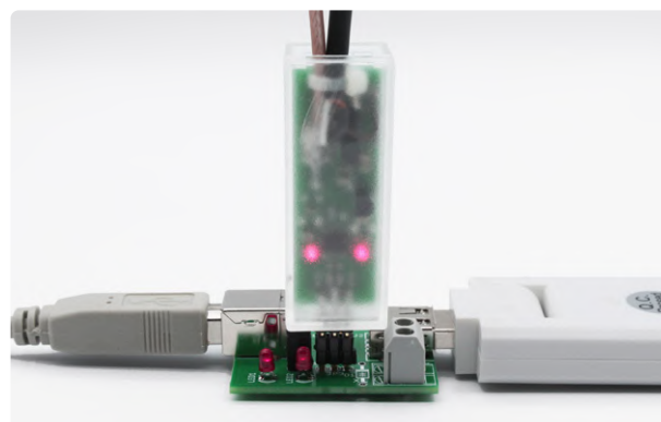
Figure 4: The USB adapter with connected current probe.
