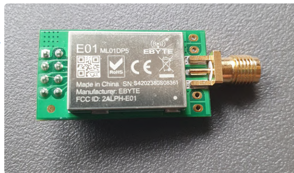
Figure 4: The nRF24 module from Ebyte [4] has additionally to the transceiver chip an SMA antenna connector and an antenna amplifier integrated.
