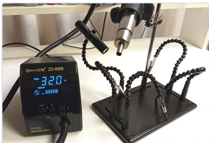
Figure 1: The ZD-8968 hot-air rework station with helping hands. (The separate stand is not shown here.)
