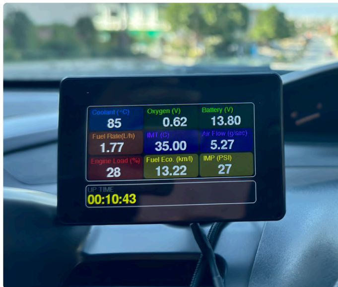
Figure 12: Close-up view of the finalized user interface for the custom OBD2 sensor dashboard, displaying real-time sensor data.
