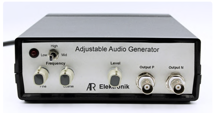
Figure 4: Front panel of the prototype design. The gain switch and stepped output attenuator are not fitted in this version.
