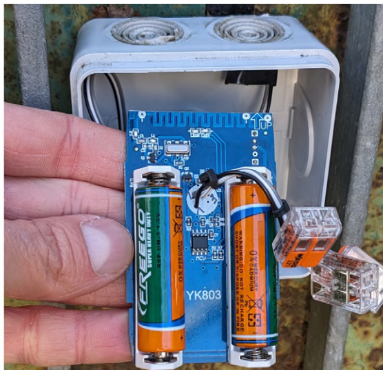
Figure 5: The PCB of the PR100 has to be mounted outside the box to allow signal transmission.
