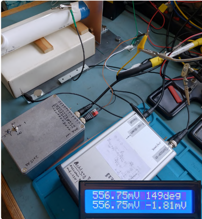
Figure 9: Setup for some test measurements (distance dependence, offset voltage effect). The "sensor" with the vibrating membrane at the "right" end faces the Cu plate, charged at a potential up to 1000 V, connected via a 33 M \Omega resistor. The "sensor" sits on a cardboard box to yield some distance from the grounded steel plate. The Cu plate is isolated by a glass plate from the steel ground. On the bottom right, the display shows the total average voltage and the phase angle (1 st line); the second line shows the voltages obtained by "rotating" the sync detector voltages with the calibration standard phase angle; thus the first value contains the proper E-field sign and the second value ideally should be zero.
