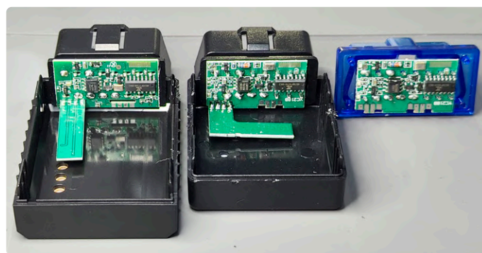
Figure 3: External view of three visually different ELM327 clone modules, which share identical internal circuitry.
