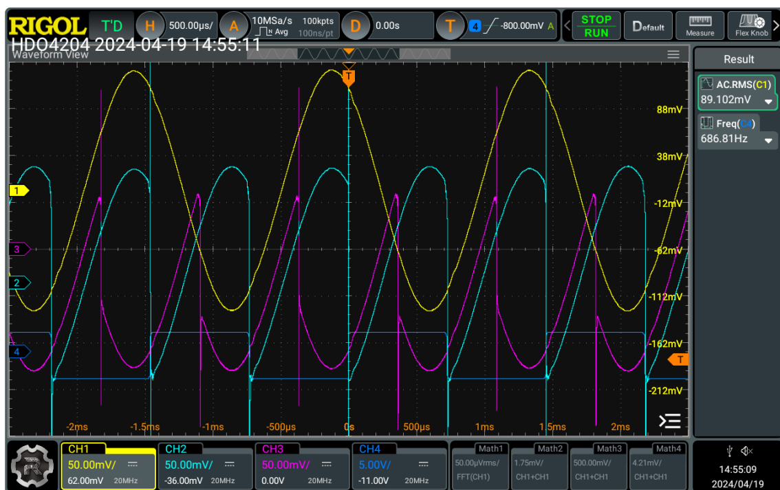
Figure 6: Phase detector outputs CH2 and CH3 obtained by multiplication of the yellow CH1 signal, CH4 shows the reference frequency. The oscilloscope's traces are obtained using averaging. The curves are vertically shifted, for a better visibility.
