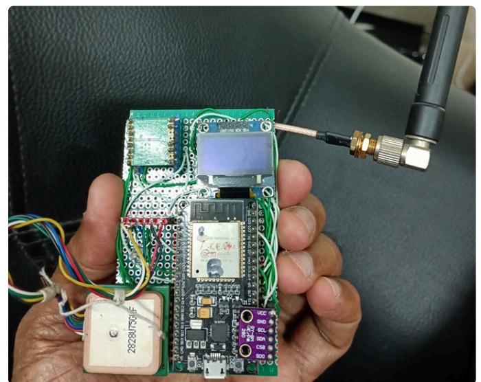
Figure 9: The prototype with ESP32, LoRa and OLED screen. GPS module and BME280 sensor are added.
