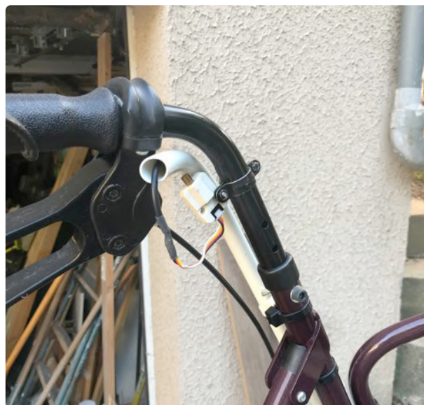
Figure 2: The vibration motor is bolted near the handle. A piece of PVC pipe hides the wiring.
