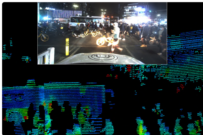
Figure 2: The real-time point cloud of automotive-grade solid-state Robosense LiDAR M1. (Source: Robosense)
