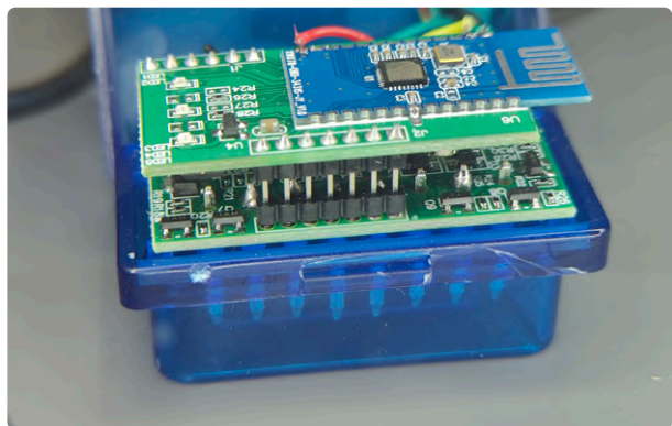
Figure 6: The PIC microcontroller-based “Double PCB” ELM327 module variant, featuring two stacked circuit boards.
