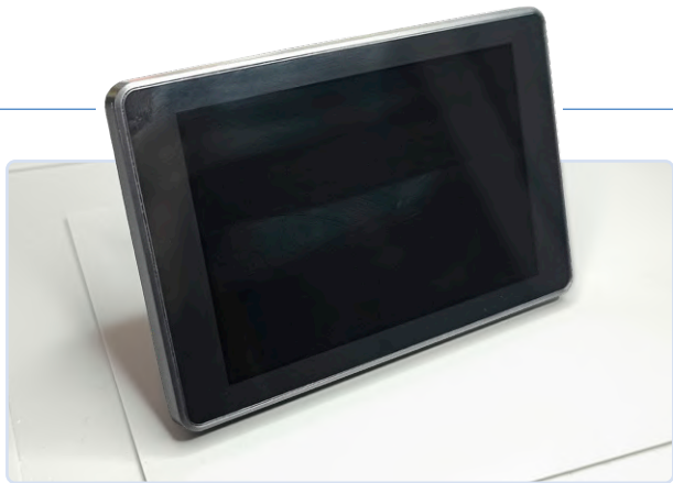
Figure 4: The JC3248W535 ESP32-S3-based LCD development board used for the sensor dashboard.
