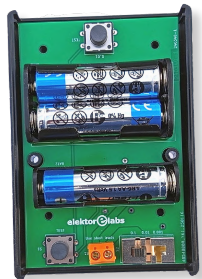
Figure 2: The adapter is powered by three 1.5-V AA cells.
