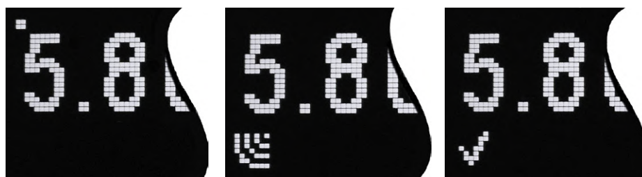
Figure 8: Auxiliary indicators, with display value updated (left), GPS output pulse received (mid), and 10 subsequent successful GPS pulses received (right).
