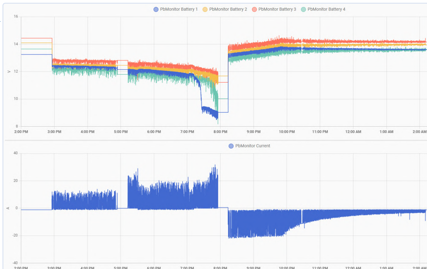
Figure 7: Charging and discharging trends of the battery bank, visualized using the Home Assistant History dashboard.
