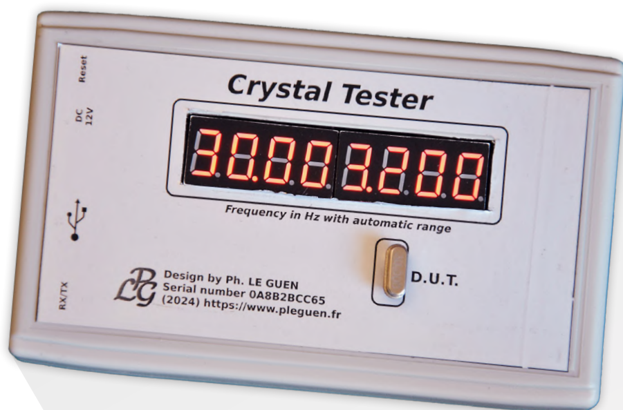
Figure 1: The eight-digit display prototype of the Crystal Tester at work, while testing a 30 MHz quartz.
