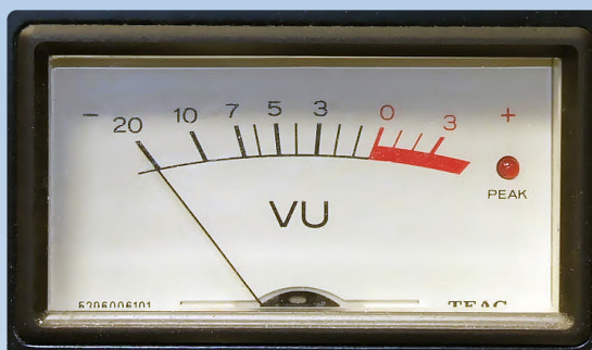
Figure 3: VU meter, calibrated in decibels, this one also has a peak LED. (Source: Wikipedia – Iainf – Creative Commons License, https://it.wikipedia.org/wiki/VU_meter#/media/File:VU_Meter.jpg )
