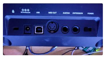
Figure 1: The M-Audio Keystation 88 MK3 has both USB and legacy 5-pin DIN connectors for its MIDI traffic.
