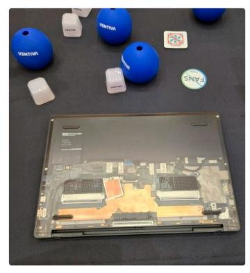
A proof-of-concept thin laptop developed by Dell and Intel using the Ventiva ICE9 cooling system. (Source: Ventiva)
