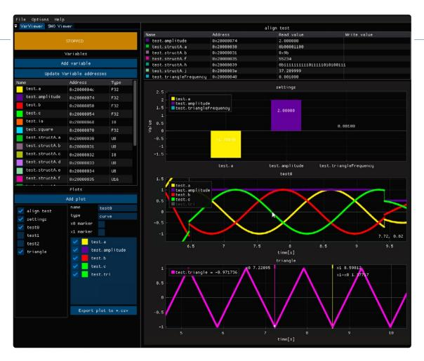
Figure 1: In Variable Viewer mode, users can visualize memory data as time-based graphs, bar charts, or tables, and edit variables directly for dynamic testing and development.
