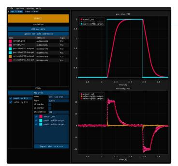
Figure 2: Variable Viewer is used here in a cascaded servo drive PID with separate plots created for the position control loop and for the velocity control loop
