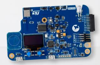
Figure 3: The STM32WB55MM-DK development board.
