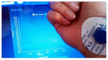
Figure 17: The RA electrode in place, with a "live" signal acquisition visible in the background.
