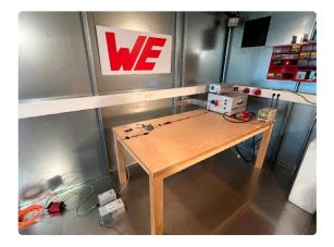
Figure 8: Measurement of the conducted interference emission on the PSE board of the SPoE reference design.
