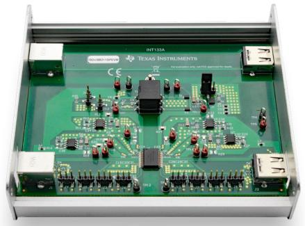
Figure 1: The evaluation board from TI with the designation ISOUSB211DPEVM, built into a metal casing.
