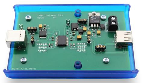
Figure 5: The custom-made, assembled circuit board in its housing.
