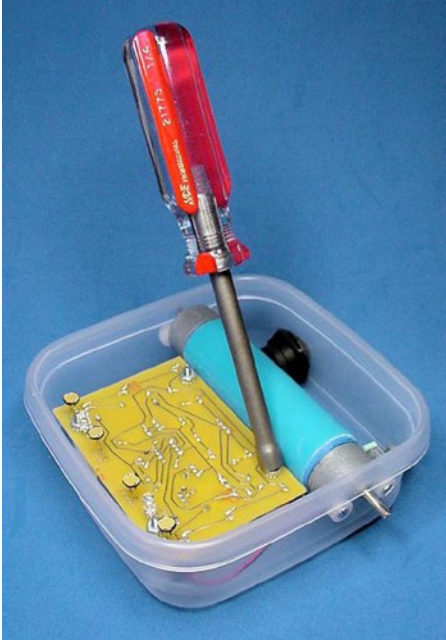
Figure 24-28. Nutdriver tightening nuts onto standoff screws
