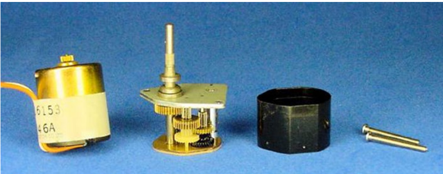
Figure 17-24. Spur gearhead motor consists of: (left to right) DC brush motor, spur gearbox, gearbox cover, and joining screws
