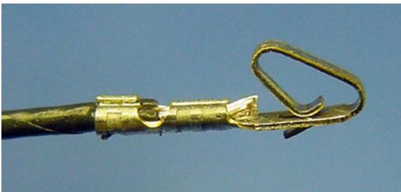
Figure 22-17. Two crimps attaching wire to terminal
