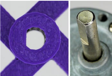
Figure B-14. A D-shaped hole in the center of the wheel hub fits a D-shaped motor shaft
