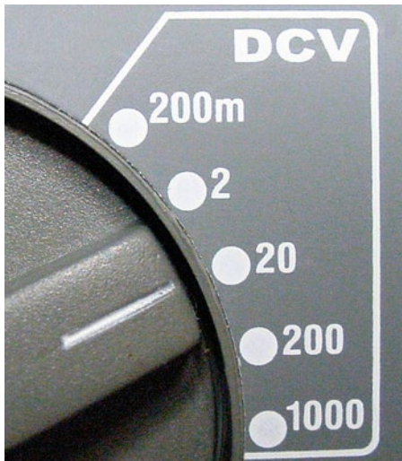
Figure 7-3. Dialing a DC voltage range above 9
