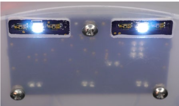
Figure 26-8. Line-following sensors soldered onto the bottom of the board
