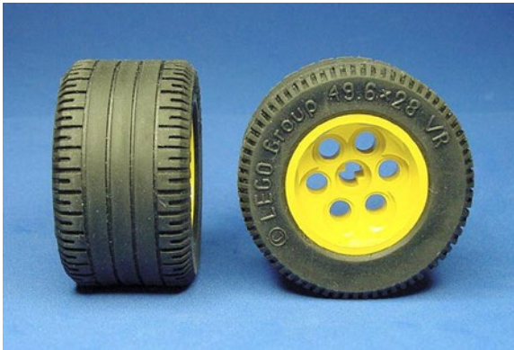
Figure 19-12. LEGO wheels selected for Sandwich. 49.6 × 28 VR: rim #6595 and tire #6594
