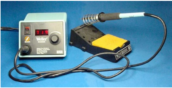
Figure 21-4. Temperature-adjustable soldering iron with sponge and stand
