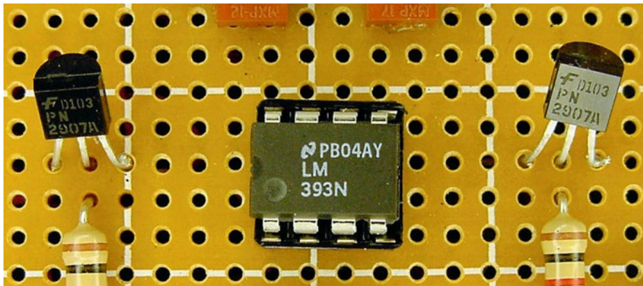
Figure 6-15. Comparator (center) flanked by two transistor switches (left and right)
