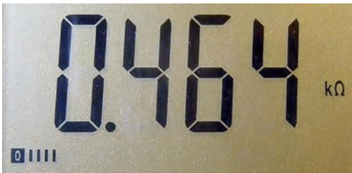
Figure 9-9. Non-friendly display of an in-range resistor value on a multimeter
