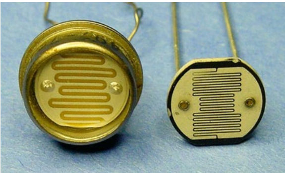
Figure 14-12. Encapsulated and exposed ceramic cadmium-sulfide photoresistors
