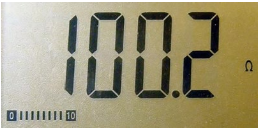
Figure 9-7. Meter displaying resistance of approximately 100 \Omega
