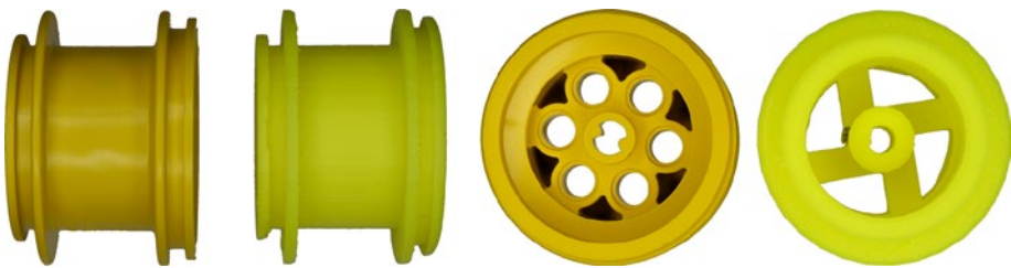
Figure B-19. Matching the dimensions of an industrial-molded Lego hub on a 3D-printed hub
