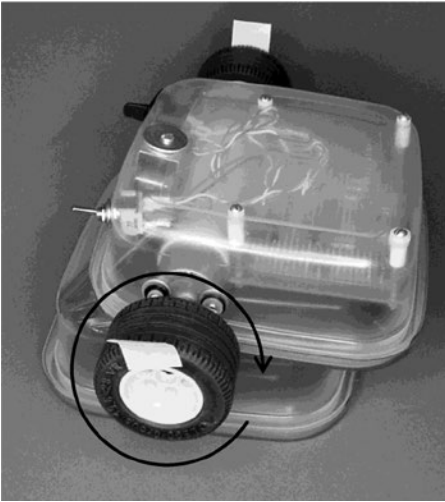
Figure 25-2. The robot's right motor spins clockwise
