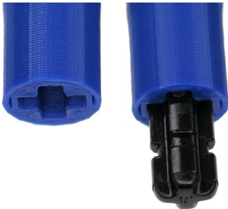
Figure B-11. The Lego cross axle fits snugly without epoxy
