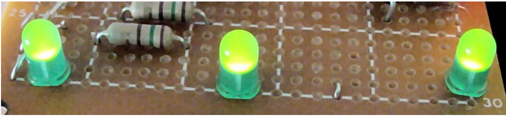
Figure 6-14. Brighter-left indicator LEDs as seen from left-side of robot
