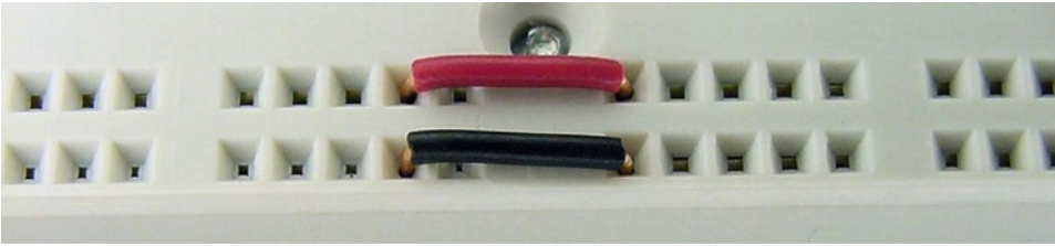
Figure 12-10. Extending buses by connecting with wire
