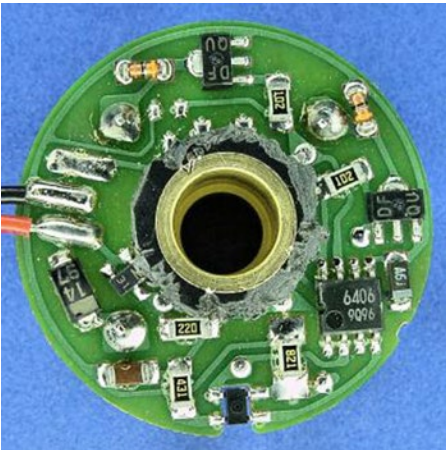
Figure 17-9. Circuit built into brushless motor
