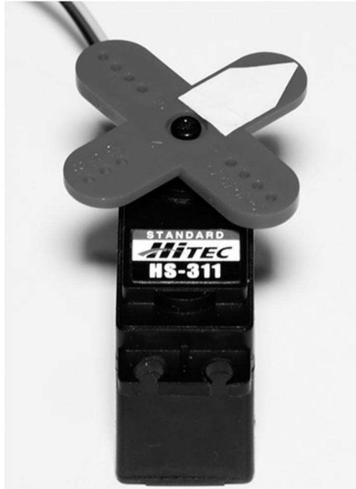
**Figure 10-13** *Hitec model HS-311 analog servo.*
