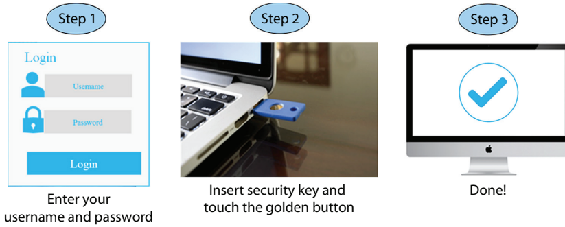
FIGURE 4.6 FIDO two-step authentication process.
