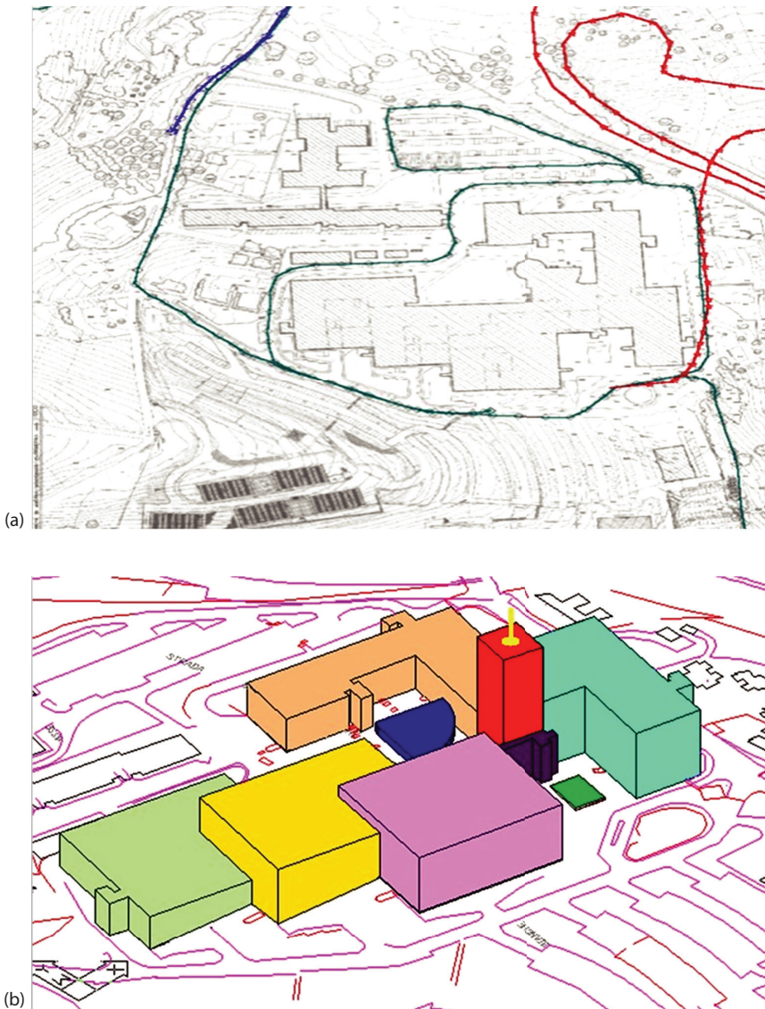
FIGURE 14.3 (a) Considered area with a path for the comparison among different models. (b) Details of the transmitting antenna placement.
