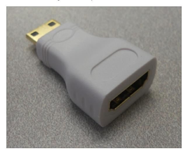
To use this connector, simply connect the adapter to your Raspberry Pi Zero, then the cable with the regular HDMI connections to the
