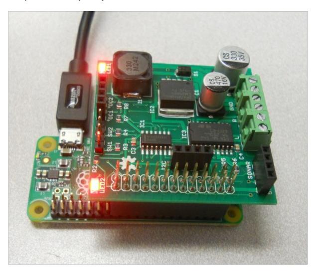
The board provides the drive signals for the DC motors on the vehicle. You can also turn the vehicle by driving each motor separately. You can change the vehicle's direction and make very sharp turns by reversing the signals. The following steps show how to connect the motor control board:
