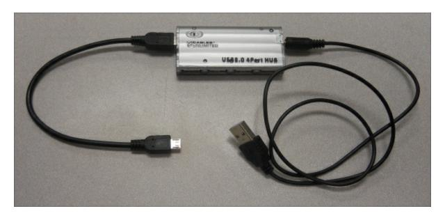
Note that there are two connections on this hub. The one to the far right is a power connection and it will be plugged into a battery or a USB power adapter with a USB port. The connection to the left is the USB connection, which will be plugged into the Raspberry Pi. To connect the power USB board to the Raspberry Pi Zero you need a cable that connects to a microUSB connector. Now, you'll have more connections to add a mouse and keyboard, webcams, and a USB WLAN device.
