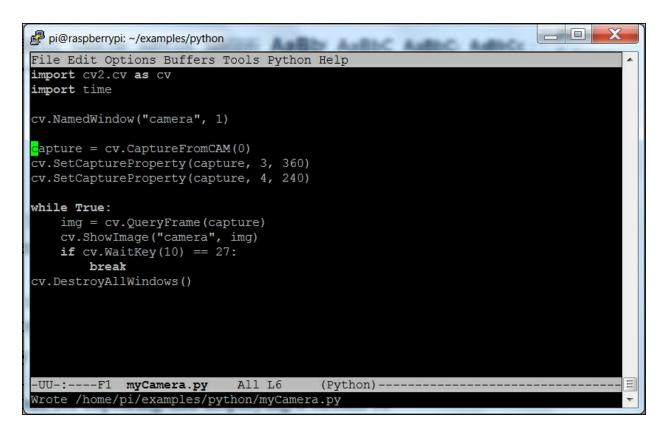
The two lines that you'll add are the two with the <a href="cv.SetCaptureProperty">cv.SetCaptureProperty</a>; they will set the resolution of the image to 360 by 240. To run this program, you'll need to either have a display and keyboard connected to Raspberry Pi or use vncviewer. When you run the code, you should see the window displayed as shown:
