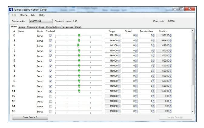
You can now use the sliders to actually control the servos. Make sure that servo 0 moves the right front lower servo, 1 the right front middle servo, 2 the right front upper servo, and so on. You can also use this to center the servos. Set all the servos so that the slider is in the middle. Now, unscrew the servo horn on each servo until the servos are centered at this location. At the zero location for all of your servos your quadruped should look like this:
