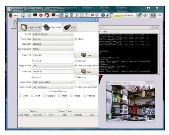
You will notice that as you adjust the resolution down, the update rate goes up; this is related to the size of the image. There are a lot of additions that you can make to your Raspberry Pi controlled car, such as adding the joystick control or more autonomy. However, let's move on to the next project.
