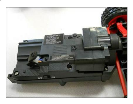
Remove this plug and these wires; you'll use Raspberry Pi Zero and a motor controller to provide the voltage to the drive system of the car. The motor will run faster or slower based on the voltage that is applied to these wires and the polarity of the voltage will determine the direction. Raspberry Pi Zero will need to provide a positive or negative 6-volt signal to control the speed and direction of the car.
