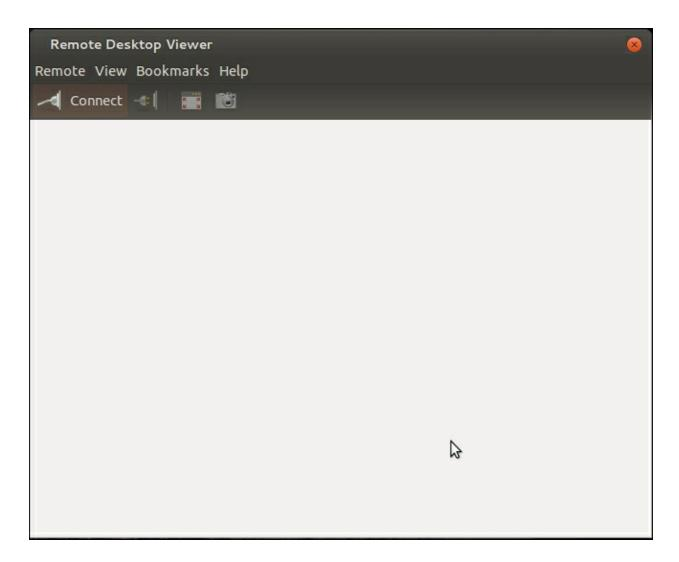
Make sure that vncserver is running on the Raspberry Pi Zero. The easiest way to do this is to log in using SSH and run vncserver at the prompt. Now, click on **Connect** on the **Remote Desktop Viewer**. Fill in the screen as follows, under the **Protocol** selection, choose **VNC**, and you should see the following screenshot:
