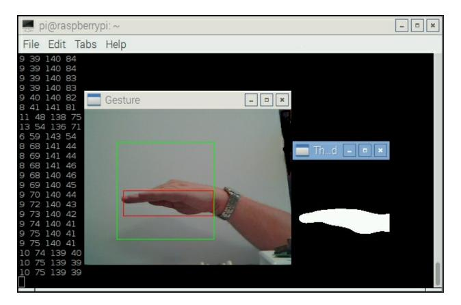
You can add some simple code to determine if your hand is making a rock, paper, or scissors using the ratios of x and y. In the preceding picture, you can see that the ratio of width to height is roughly 140/80 for paper. For a rock, the ratio is going to be roughly 85/55. For scissors, it is going to be 140/40. Here is the code for the library that determines a rock/paper/or scissors:
