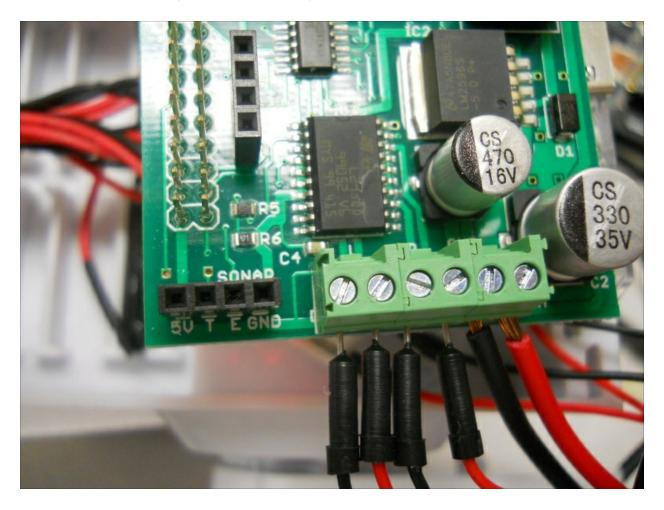
To use this connector, simply connect the VCC to the 5V, the Trig to the T connection, the Echo to the E connector, and the GND to the GND connection. You can then use the library for the motor controller board and simply call the function rr.get\_distance(). Similarly, there is also a special connector and libraries for the I2C interface, if you want to add the compass to your mobile project.
