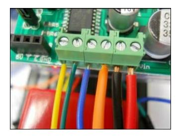
4. Connect the 3.3-volt and GND connectors to the **General Purpose Input/Output (GPIO)** pins of Raspberry Pi. Here is a layout of these pins:
