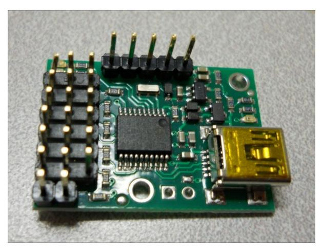
Make sure you order the assembled version. This piece of hardware will turn the USB commands from the Raspberry Pi Zero into signals that control your servo motors. There are two connections that you'll need to make to the servo controller to get started: the first to the
