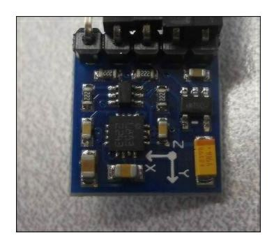
This type of digital compass uses magnetic sensors to measure the earth's magnetic field. The output of these sensors is then made accessible to the outside world through a set of registers that allow the user to set things, such as the sample rate and continuous or single sampling. The X, Y, and Z directions are the output using registers as well.
