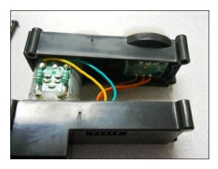
As you can see in the preceding image, the blue and yellow wires are attached to a DC motor, and the orange, brown, and red wires are attached to another control circuit. The motor will drive the wheels left or right, the polarity of the voltage will determine the direction, and its magnitude will cause the wheels to turn more or less sharply. The
