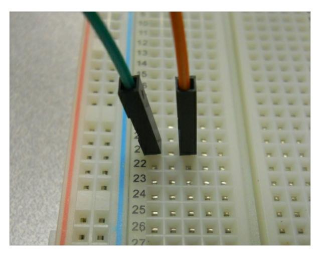
The two rows on each side of the board are generally designed to provide power, so they are connected up and down. Connect pin 2, 3 volts, to the + connection and pin 6, GND, to the + and – rows of the breadboard, as shown:
