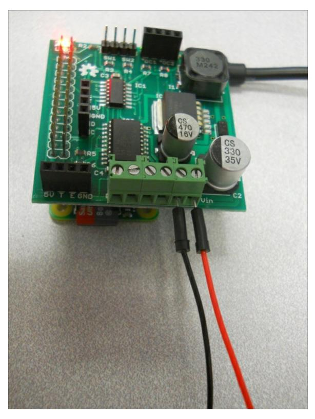
2. Next, connect one of the drive signals to the motor 1 connector on the board. Connect motor 1 to the right motor and motor 2 to the
