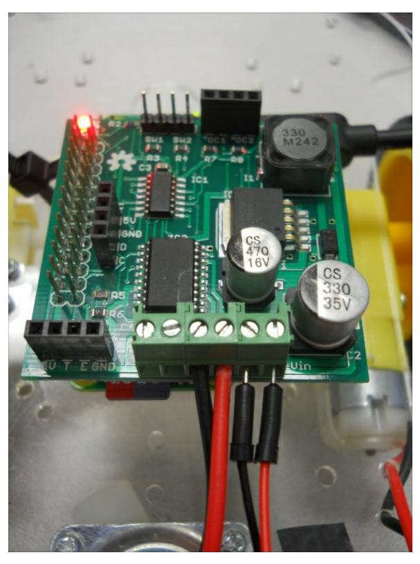
3. Then, connect the second drive connector to the motor 2
