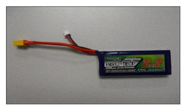
This battery will come with two connectors, one with larger gauge wires for normal usage and a smaller connector to connect to the battery recharger. You'll want to build connectors that can connect to the screw-type connectors of the servo controller. I purchased a few XT60 connector pairs and soldered some wires to the mating connector of the battery and then screwed these into the servo controller.
