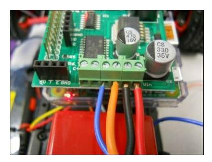
3. Connect the front drive connector to the motor 2 connectors on the board, as shown in the following image:
