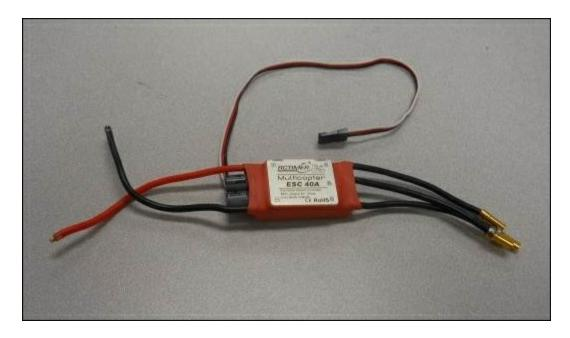
The red and black wire connectors are the connectors that are soldered to the bottom plate of the frame. The other three
