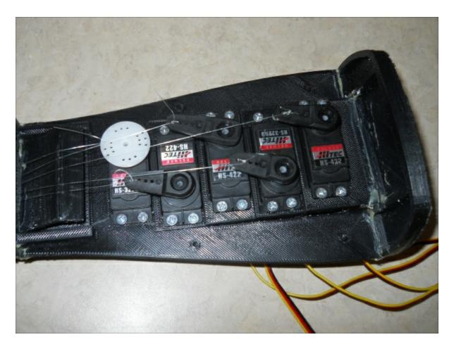
Connect each of the digits to a servo, and then connect the entire hand to a bracket; this will act as the wrist. You'll also connect this to a servo that can turn the wrist.
