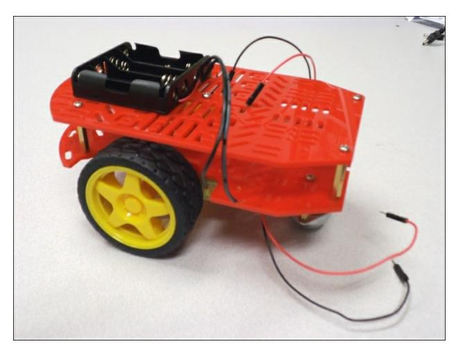
This one also needs to be assembled but it is fairly straightforward. You could also choose a tracked platform instead of a wheeled platform. A tracked platform has more traction but is not as nimble, as it takes a longer distance to turn. Again, manufacturers make preassembled units. The following image is an example of a preassembled tracked platform made by Dagu. It's called the Dagu Rover 5 Tracked Chassis:
