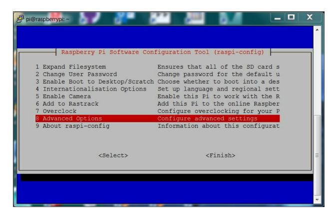
Now, you'll turn off sending the serial output on boot up by selecting the A8 Serial, Enable/Disable shell and kernel m option, as shown:
