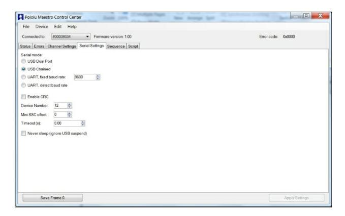
Make sure that **USB Chained** is selected; this will allow you to connect and control the motor controller over USB. Now go back to the main screen by selecting the **Status** tab; now you can actually turn on the 12 servos. The screen should look like this:
