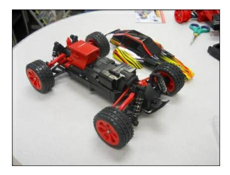
There are two connections that you will want direct access to. The first is the drive motor, and the second is the steering mechanism. For this particular model of RC car, the drive mechanism is in the rear. What you are normally looking for is two wires that will directly drive the DC motor of the car. In this system, there is a connector in the rear of the car; it looks similar to the following image:
