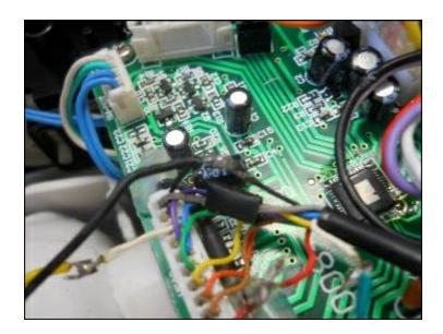
3. Now, snip the white wire and connect a wire to the end that is connected to the white header connector, as shown in this image:
