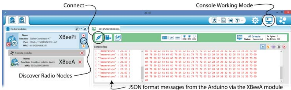
Figure 13-13: The XCTU Console working mode receiving JSON messages from the Arduino XBee device
