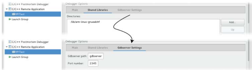
Figure 7-9: Setting the RPi gdb server port
