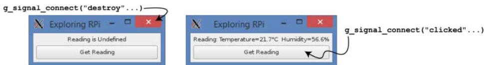
Figure 14-5: The GTKsensor application
