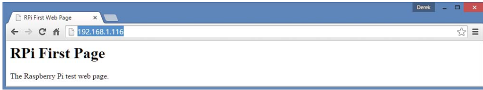
Figure 12-3: The first web page from the Nginx server
