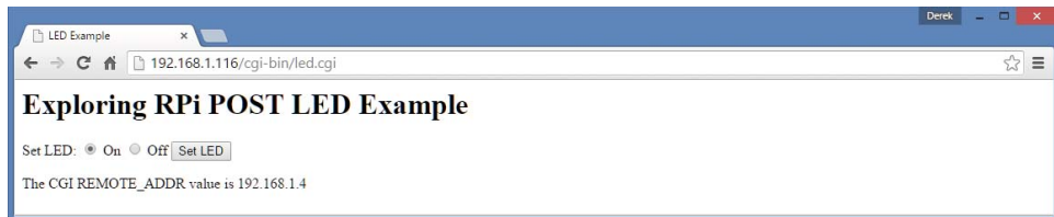
Figure 12-7: The LED Cgicc form post example
