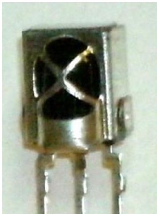
Figure 5-1. The VS1838B PIN photodiode
