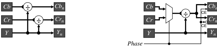
Figure 5.22 Sharing a divider in a two-phase pipeline.
