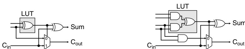
Figure 2.10 Left: logic required to implement a full adder with a single logic cell; right: a two-bit multiplication in a single logic cell. (Adapted from Elzinga et al. (2000); reproduced by permission of Xilinx, Inc.)
