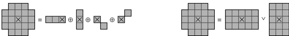
Figure 8.49 Example structuring element decompositions. Left: series decomposition using dilation; right: parallel decomposition using OR.
