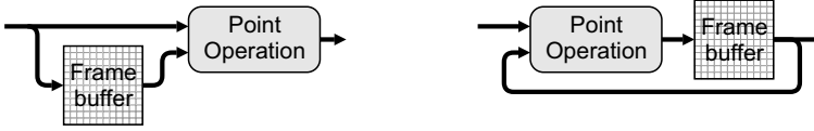
Figure 6.18 Two-image point operation applied to successive images. Left: sequential access; right: recursive access. A frame buffer is required to hold the image from the previous frame.
