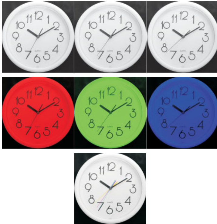
Figure 6.28 Temporal false colouring. Images taken at different times are assigned to different channels, with the resultant output showing coloured regions where there are temporal differences.
