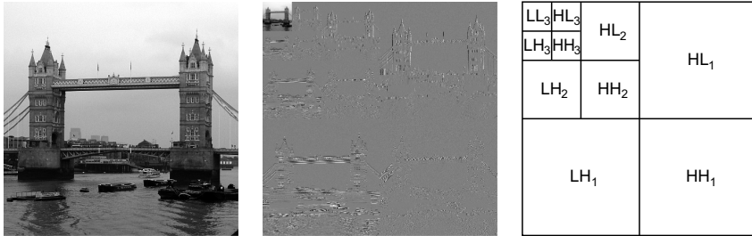
Figure 10.20 Two-dimensional wavelet transform of an image. Left: input image; centre: wavelet transform (using the Haar wavelet); right: position of the decomposition components for each level. (Photo courtesy of Robyn Bailey).
