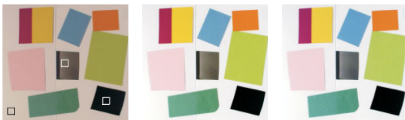
Figure 6.44 Correcting using black, white and grey patches. Left: original image with the patches marked; centre: stretching each channel to correct for black and white, using Equation 6.90; right: adjusting the gamma of the red and blue channels using Equation 6.91 to make the grey patch grey.
