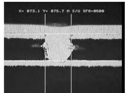
FIGURE 29.2 Example of a plated filled blind microvia.
