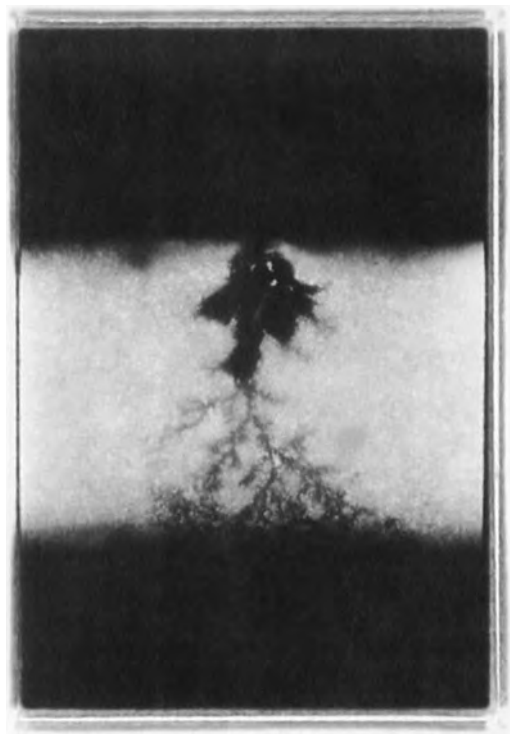
FIGURE 57.10 Transmitted light micrograph through a PCB that failed in the field. Dendritic growth has formed at the interface of a UV-cured screened solder mask and the FR-4 surface.
