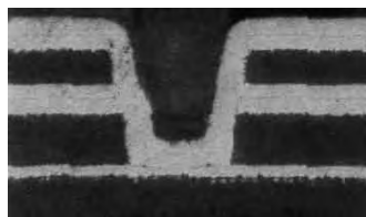
FIGURE 29.5 Horizontal PTH/pulse-plated microvia.
