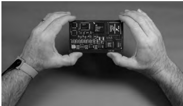
FIGURE 52.2 Appropriate method of handling board to avoid contamination and electrostatic discharger damage. Note position of fingers and the use of a grounding wrist strap.
