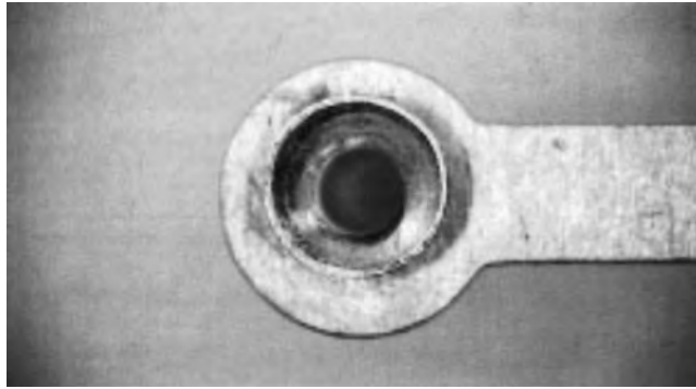
FIGURE 52.8 Flared flange. Acceptable for all Classes.
