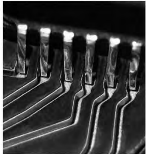
FIGURE 23.36 Various views of SEMs of imprinted circuit liquids and traces. (Courtesy of Dimensional Circuits.)
