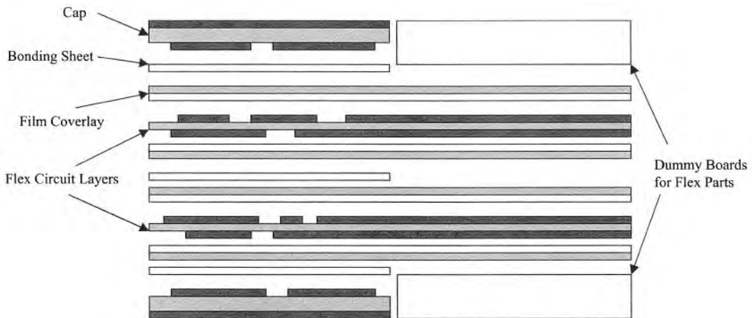
FIGURE 65.5 Standard manufacturing flow for multilayer rigid/flexible circuits.
