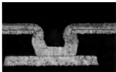
FIGURE 29.4 Horizontal PTH/pulse-plated resin-coated copper.
