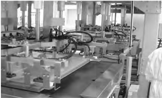
FIGURE 6.12 Automated build-up of copper and prepreg.
