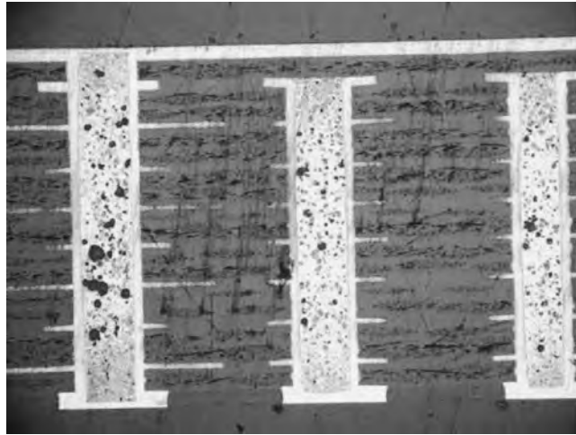
FIGURE 27.20 Micrograph of conductive via fill.
