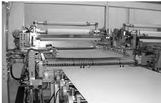
FIGURE 6.10 Sheeting of rolls of copper foil.
