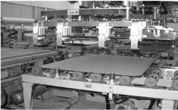
FIGURE 6.11 Automated build-up of copper and prepreg.
