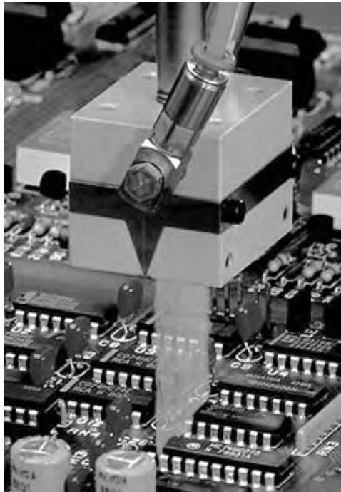
FIGURE 41.3 Selective coating using an atomizing nozzle. (Courtesy of Asymtek.)
