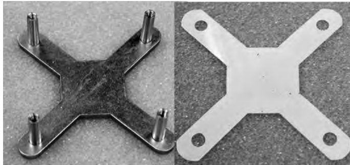
FIGURE 50.2 Stainless steel bolster plate (l) and insulator (r). (Courtesy of Hewlett-Packard.)
