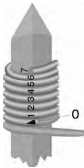
FIGURE 52.36 Solderless wire wrap acceptability. (IPC)
