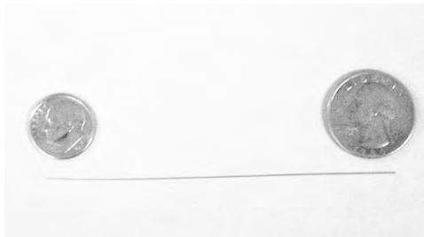
FIGURE 39.1 Tapered pin for a fine-geometry fixture.
