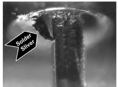
FIGURE 49.8 A solder sliver (dashed outline) pushed out of a HASL-coated PTH.
