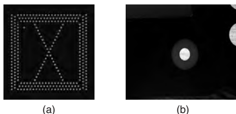
FIGURE 40.22 Vision system images: (a) a flip chip component; (b) a printed circuit board fiducial. ( Courtesy of Universal Instruments. )
