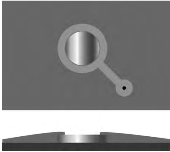
FIGURE 51.10 Soldermask defined BGA land. (Courtesy of IPC.)
