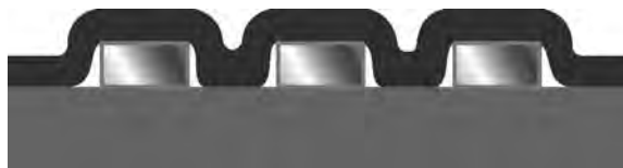
FIGURE 51.11 Soda strawing between copper trace and solder-mask. (courtesy of IPC.)
