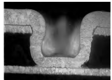
FIGURE 29.12 Example of a blind via that is 5.0 mil in diameter and 3.0 mil deep, plated with chemically mediated bath.
