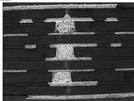
FIGURE 23.19 Examples of TLPS cross-sections of three layer pairs with lasered-vias filled with TLPS paste vias and buried vias for FR-4 innerlayers.
