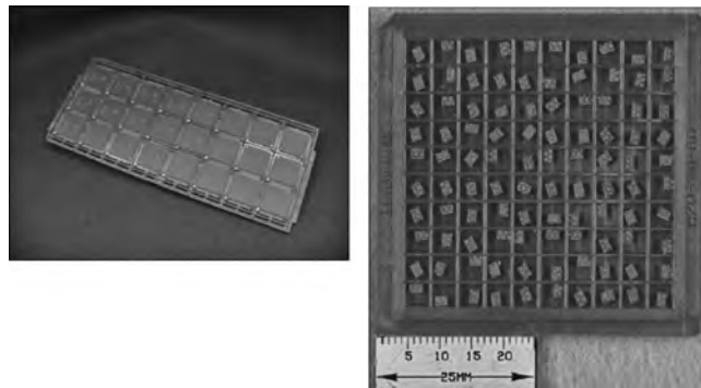
FIGURE 40.28 Components packaged in matrix trays. (Courtesy of Sandia National Laboratories.)
