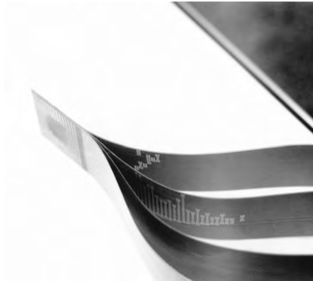
FIGURE 65.7 Example of typical multilayer rigid/flexible circuit with via holes. (Source: Toshiba.)
