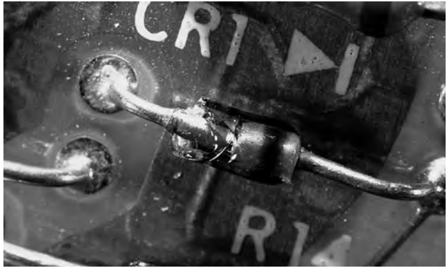
FIGURE 52.15 Example of physical damage to component after insertion. This is a “defect” condition and cause for rejection. (a) Axial lead component, (b) Chip component. (IPC)
