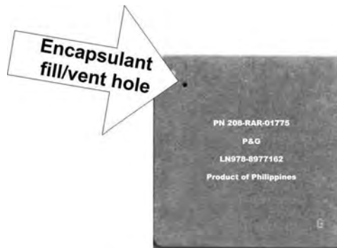
FIGURE 46.4 If water enters an improperly sealed encapsulant vent/fill hole on an IC package, shorting or corrosion can occur. (Courtesy of Hewlett-Packard.)
