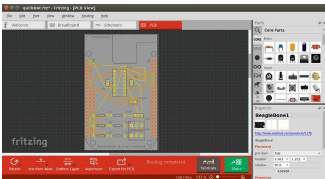
Figure 9-18. PCB with original board, without notch for Ethernet connector
