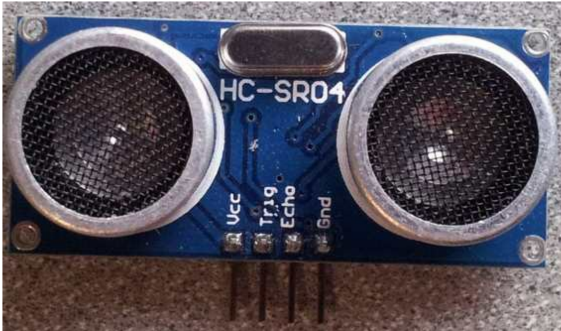
Figure 2-12. HC-SR04 Ultrasonic range sensor
