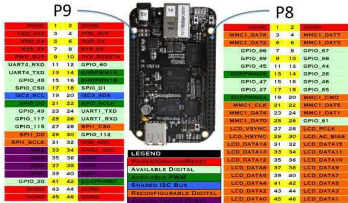
Figure 2-3. Some of the many sensor connection options on the Bone
