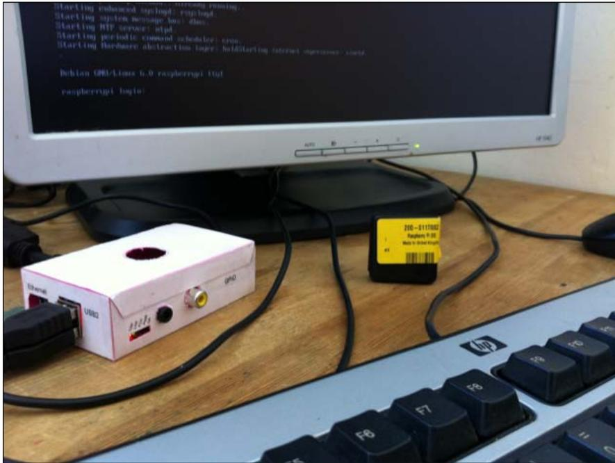
The preceding image shows a Raspberry Pi in the Punnet with monitor, keyboard, and mouse.
