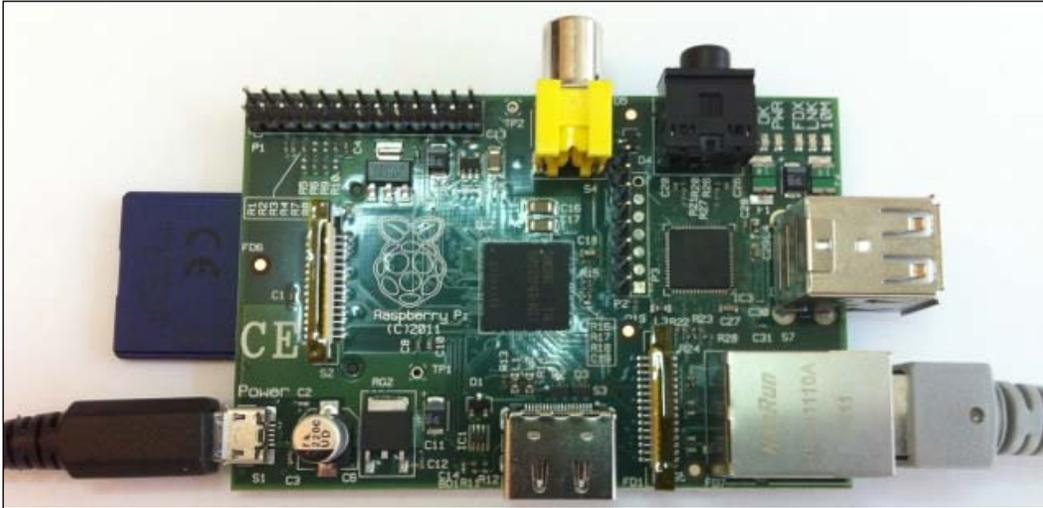
The preceding image shows a Raspberry Pi with an SD card, a network, and power cables.
