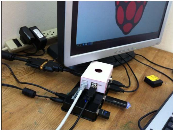
The preceding image shows a Raspberry Pi in the Punnet lying on a USB hub with devices attached.
