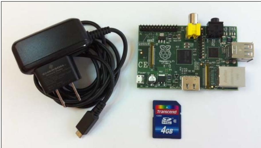
The preceding image shows a Raspberry Pi without a case, an SD card, and a power supply.
