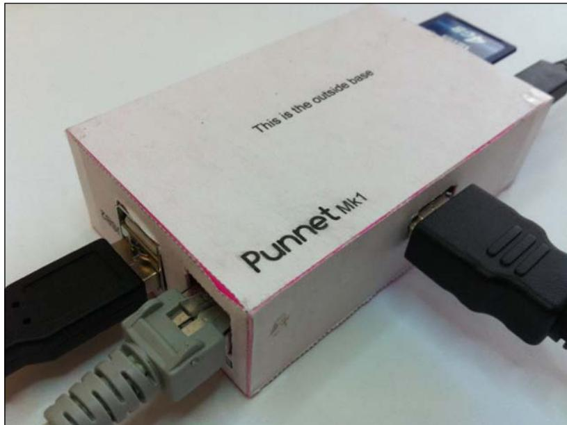
The preceding image shows the Punnet in use. A printed Punnet was glued to pink card stock before folding. The card stock added strength and stability to the case.
