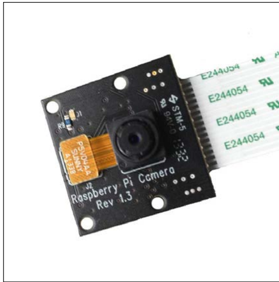
The Raspberry Pi NoIR camera module; it looks similar to the standard model
