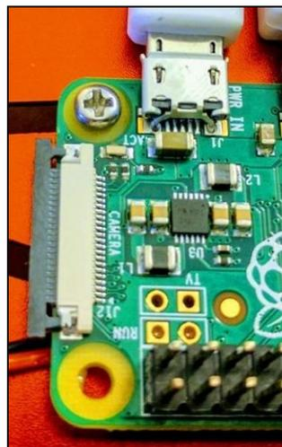
Slide the tabs of the camera interface carefully
