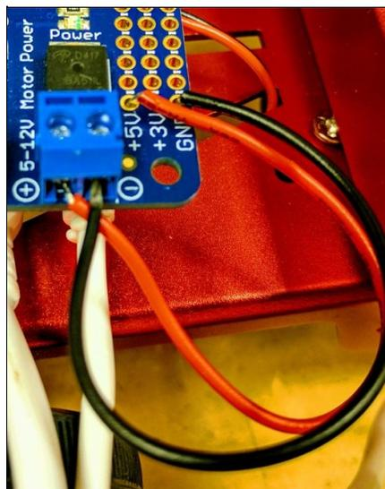
Connect 5V and GND to the motor power supply terminals
