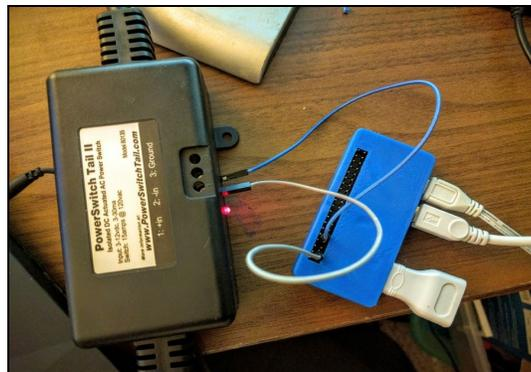
PowerSwitch Tail II connected to a Raspberry Pi Zero
