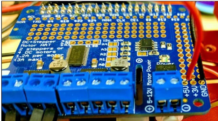
Solder red and black pieces of wires from 5V and GND pins
