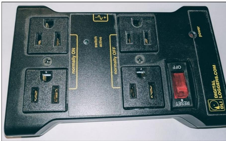
Enclosed high power relay for Raspberry Pi
