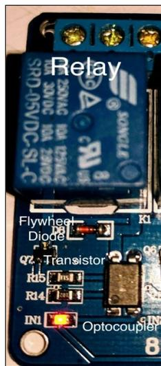
The components of each relay circuit (labeled)
