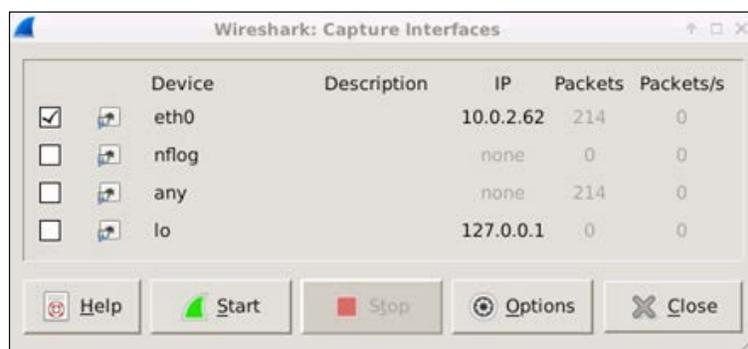
If you are running the Raspberry Pi as a bridge between two Ethernet interfaces, you will need to select the `bridge0` interface as your data source. If you are using the ARP poisoning method to read data, meaning you are only using one interface, you will need to select a network facing port such as `eth0`, as shown in the previous screenshot example. Click on the **Start** button once you click the check box next to the interface you are going to monitor.
