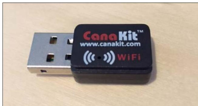
The **CanaKit** Wi-Fi adapter is good for the Raspberry Pi because of its size, portability, and compatibility.
