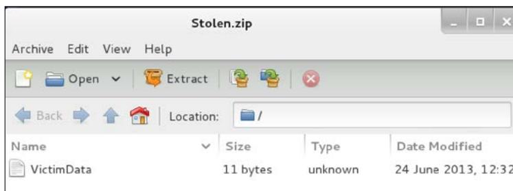
To compress files, you can drag the file into the window and File Roller will ask you whether you want to create a new compressed file. Here is an example in the following screenshot of dropping the `VictimData` file into File Roller and creating a new compressed file called `VictimDataNew.tar.gz`. At the file prompt, I told File Roller to call my new file `VictimDataNew` and it added the `.tar.gz` extension once the file was compressed:
