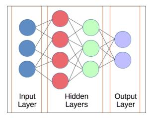
Typically, we consider fully connected layers. The outputs of each neuron in a layer go to all neurons in the next layer. While we do define a fully connected network, many of the weights will be set to zero during the training process, effectively removing these links. Fully connected neural networks are also simpler and more efficient to program than other connection patterns.
