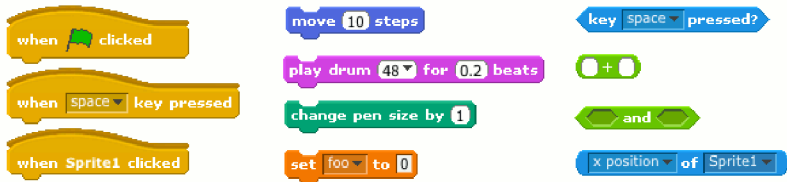
Figure 5-2. There are three types of blocks in Scratch: hat blocks (left), stackable blocks (center), and reporter blocks (right).
