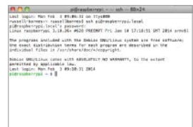
Fig 2: The Avahi tool enables you to log into your Pi via SSH by name, rather than needing to discover its IP address
