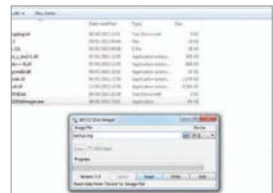
Fig 4: Win32 Disk Imager makes backing up the entire OS easy, and you can even use it to write the image back to the SD card
