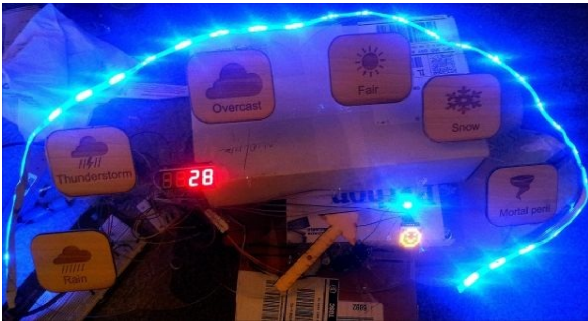
A Weasley weather clock built using the Arduino and the Raspberry Pi
