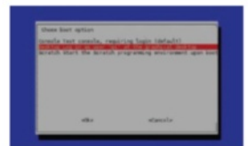
Fig 3: Change the default selection to desktop for the next time you use the Raspberry Pi
