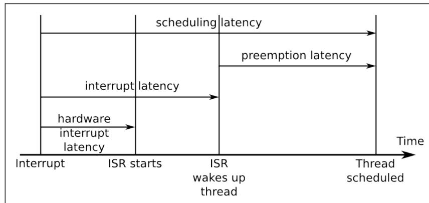
Firstly, there is the hardware interrupt latency from the point at which an interrupt is asserted until the **ISR (interrupt service routine)** begins to run. A small part of this is the delay in the interrupt hardware itself but the biggest problem is interrupts disabled in the software. Minimizing this *IRQ off time* is important.
