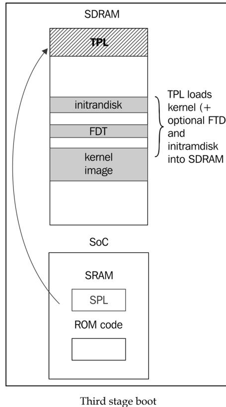
At the end of the third phase, there is a kernel in memory, waiting to be started. Embedded bootloaders usually disappear from memory once the kernel is running and perform no further part in the operation of the system.
