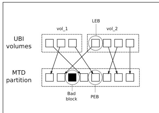
In this way, UBI fulfills two of the requirements of a flash translation layer: wear leveling and bad block handling.
