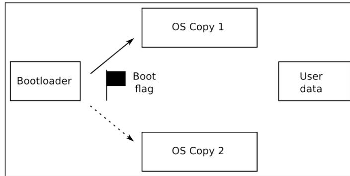
Initially, the boot flag is not set, so the bootloader loads copy 1. To install an update, the updater application, which is part of the operating system, overwrites copy 2. When complete, it sets the boot flag and reboots. Now, the bootloader will load the new operating system. When a further update is installed, the updater in copy 2 overwrites copy 1 and clears the boot flag and so you ping-pong between the two copies.
