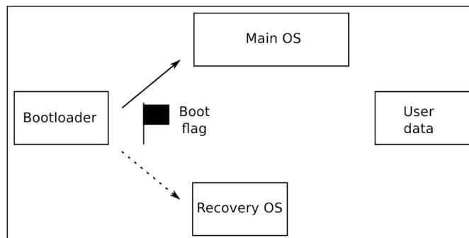
When you want to install an update, set the boot flag and reboot. Once the recovery operating system is running, it starts the updater which overwrites the main operating system images. When done, it clears the boot flag and reboots again, this time loading the new main operating system.
