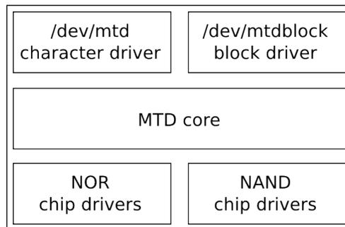
The chip drivers are at the lowest level and interface with flash chips. Only a small number of drivers are needed for NOR flash chips, enough to cover the CFI standard and variations plus a few non-compliant chips which are now mostly obsolete. For NAND flash, you will need a driver for the NAND flash controller you are using; this is usually supplied as part of the board support package. There are drivers for about 40 of them in the current mainline kernel in the directory `drivers/mtd/nand`.
