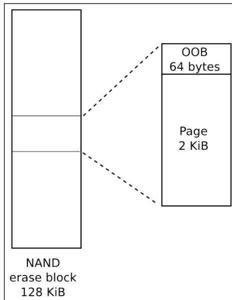
During production, the manufacturer tests all the blocks and marks any that fail by setting a flag in the OOB area of each page in the block. It is not uncommon to find that brand new chips have up to 2% of their blocks marked bad in this way. Furthermore, it is within the specification for a similar proportion of blocks to give errors on erase before the erase cycle limit is reached. The NAND flash driver should detect this and mark it as bad.
