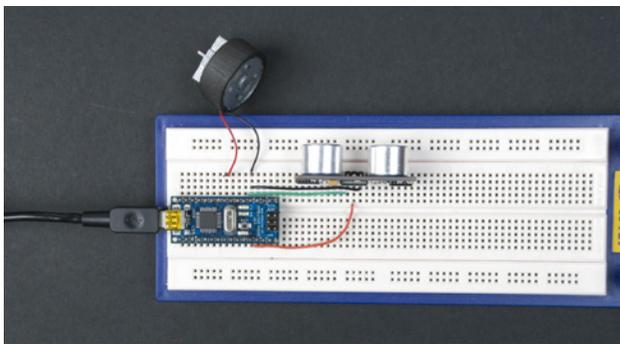
Figure 3-17. Vibration motor and ultrasonic sensor connected
