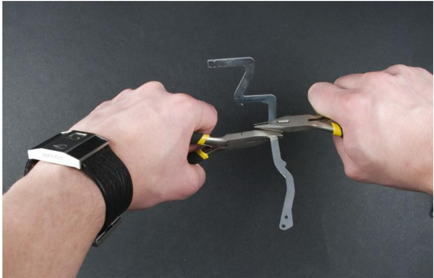
Figure 8-51. Cutting the front fork
