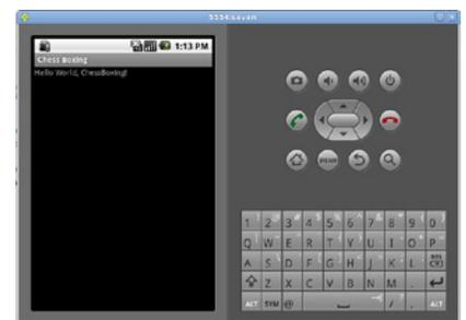
Figure 6-20. “Hello World” in the emulator, indicating a successful installation
