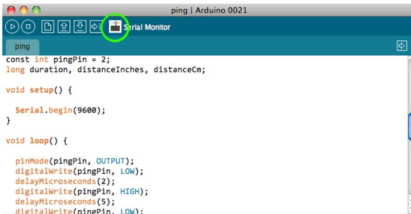
Figure 3-13. The Arduino development environment's Serial Monitor button
