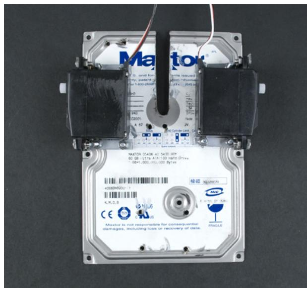
Figure 8-38. Attached wheel servos from below
