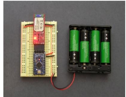
Figure 8-18. Bluetooth Mate connected to Arduino Pro Mini
