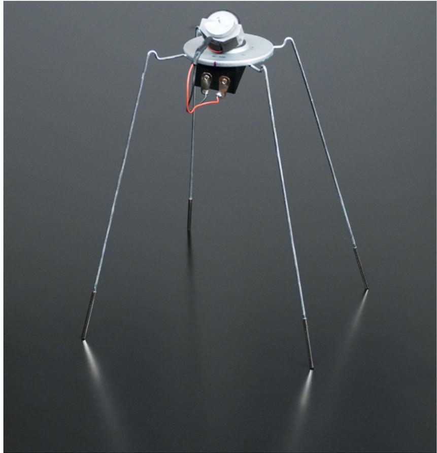
Figure 3-21. Vibrating robot, still lacking the ultrasonic sensor
