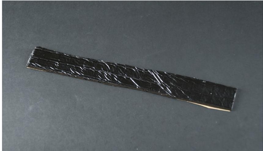
Figure 5-35. Strip of bitumen carpet for balancing the tube
