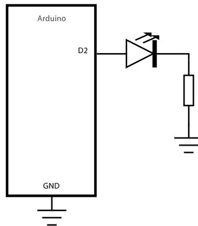
Figure 5-9. Connection diagram
