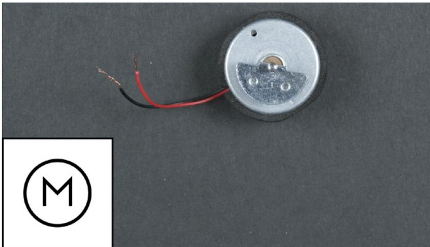
Figure 3-14. Vibration motor
