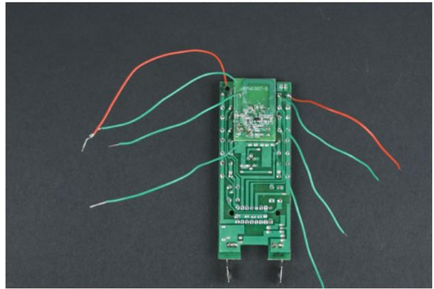
Figure 7-16. Soldered wires
