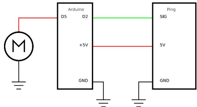
Figure 3-18. Vibration motor and ultrasonic sensor schematic
