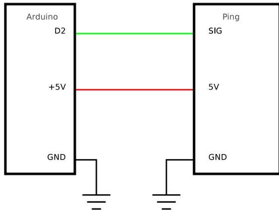
Figure 3-12. Schematic for the ultrasonic sensor circuit
