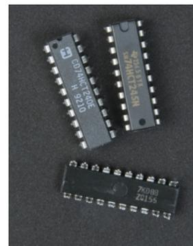
Figure 7-22. Integrated circuits
