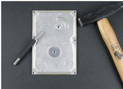
Figure 8-29. Making marks for the holes with a punch
