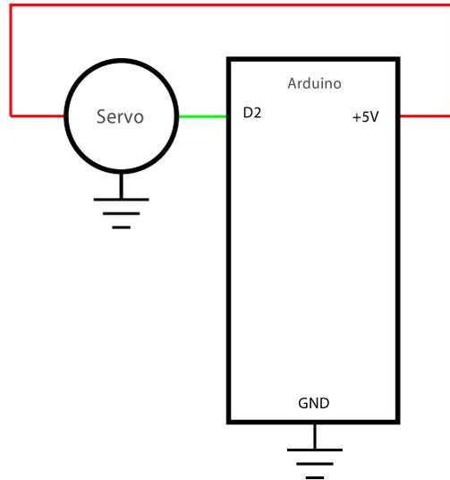
Figure 4-5. Arduino/servo schematic
