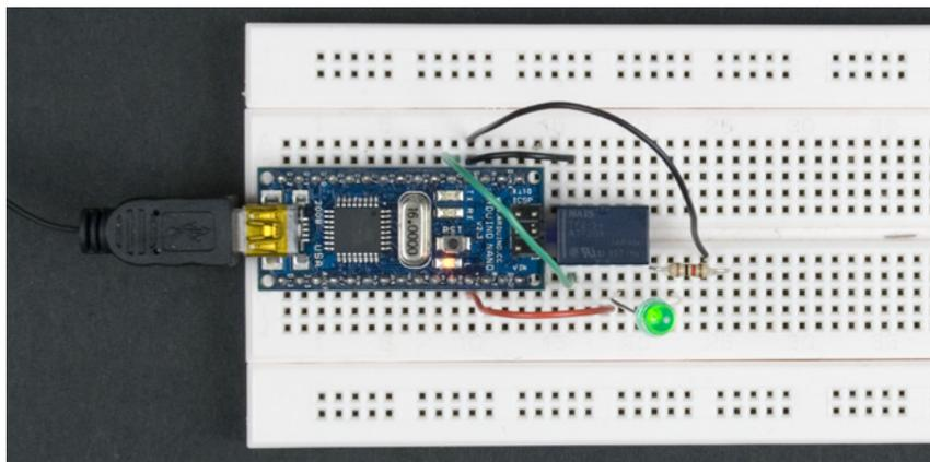
Figure 7-5. Connecting the LED with a relay
