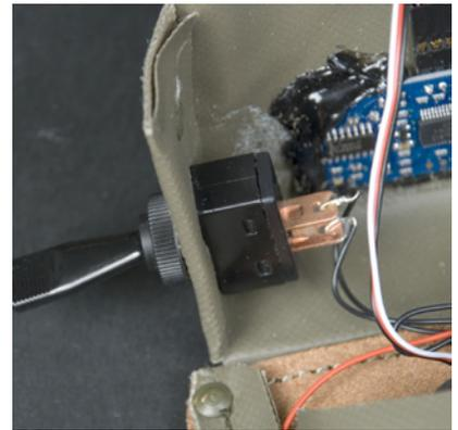
Figure 3-40. A switch attached to the enclosure
