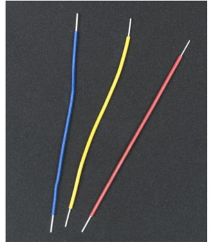
Figure 3-7. Jumper wires
