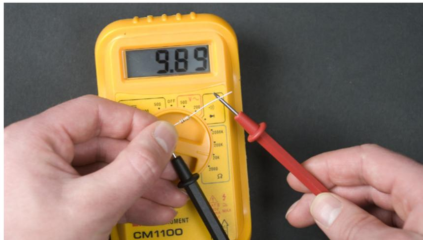
Figure 5-6. Measuring resistance with a multimeter
