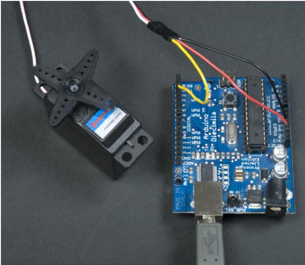
Figure 4-4. Servo connection
