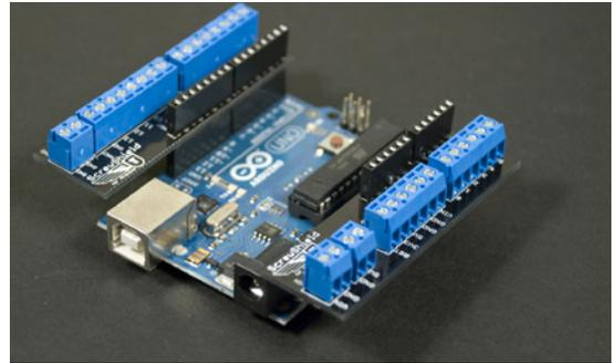
Figure 4-22. The ScrewShield
