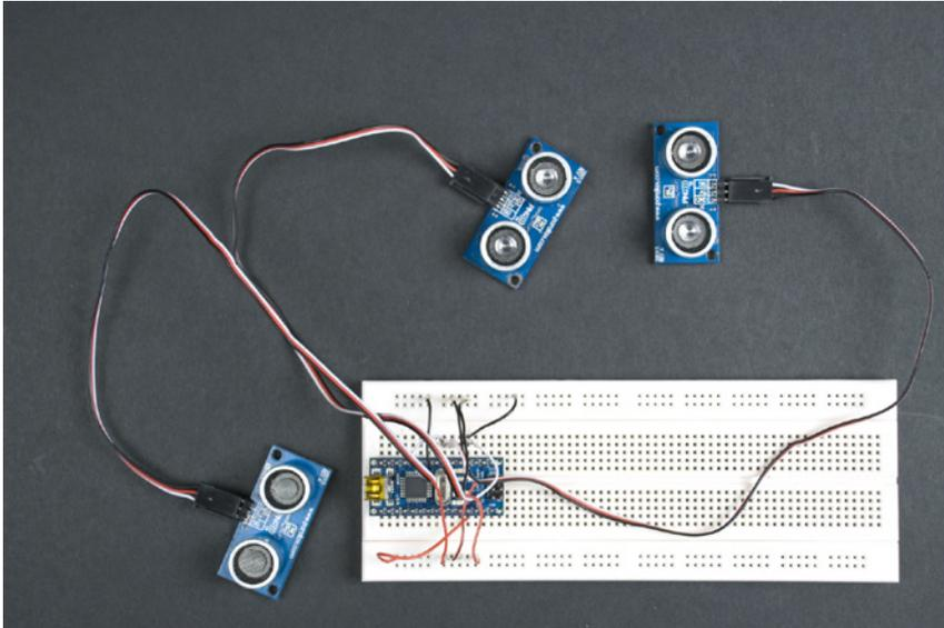
Figure 5-33. Ultrasonic sensors attached to the prototyping breadboard
