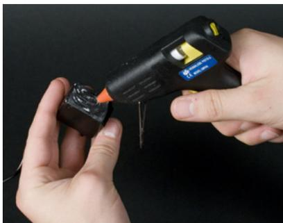
Figure 4-13. Spreading the hot glue
