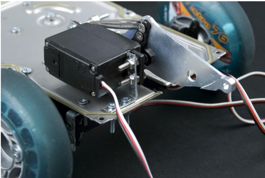
Figure 8-49. Kicking mechanism
