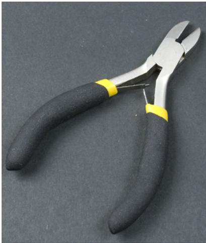
Figure 1-13. Diagonal-cutter pliers
