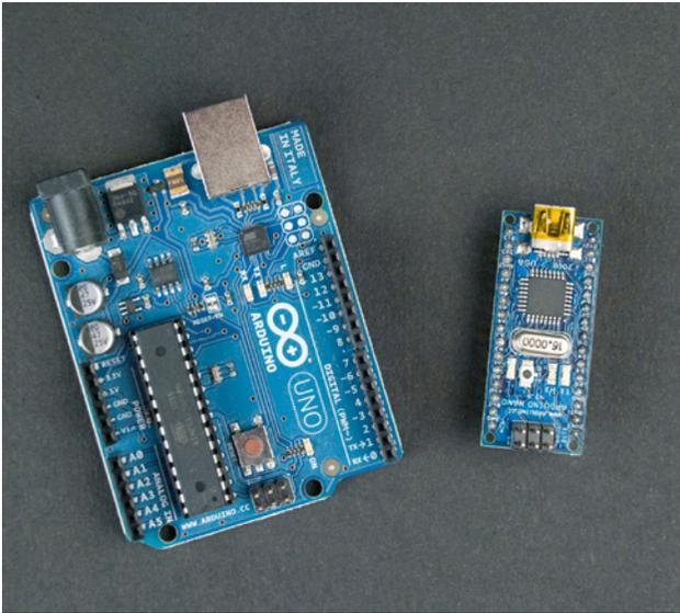
Figure 2-1. Arduino Uno (left) and Arduino Nano (right)
