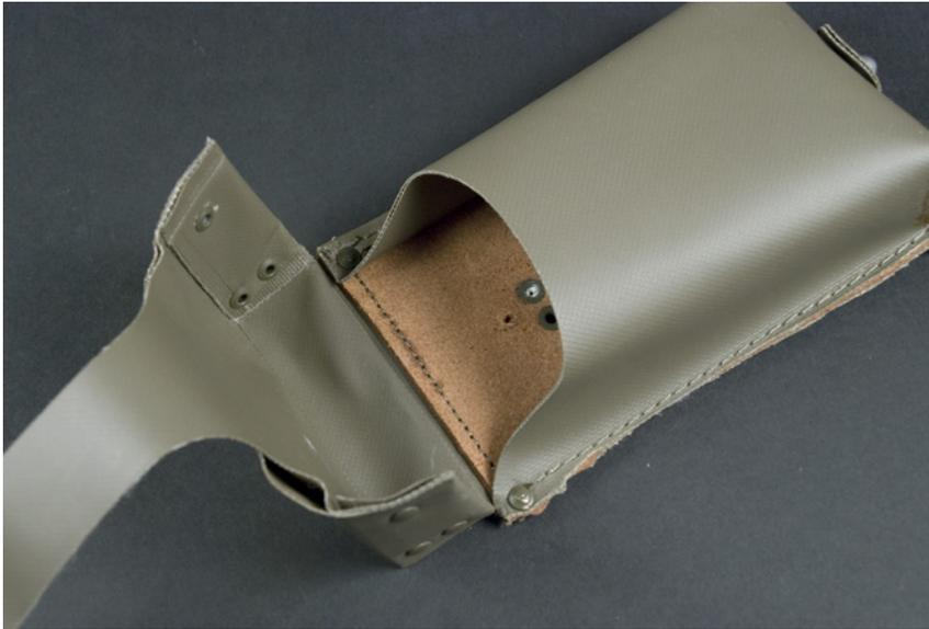
Figure 3-23. Hole created for attaching the vibration motor
