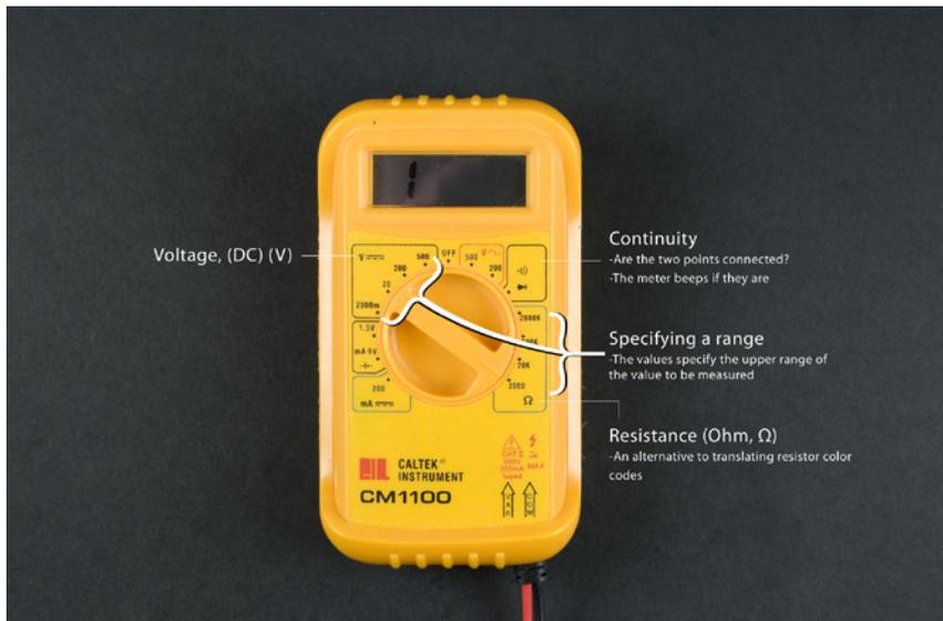
Figure 1-26. The most common functions of a multimeter
