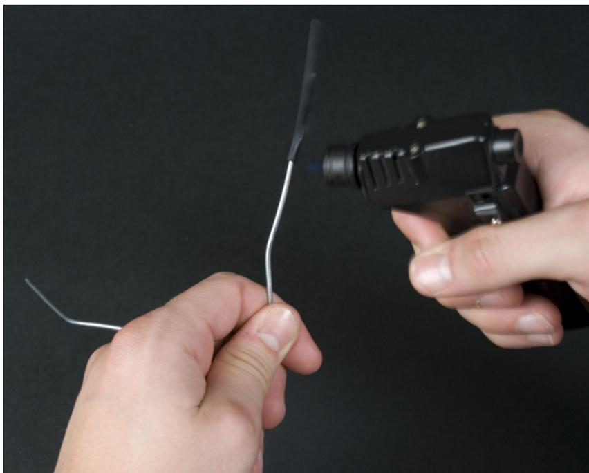
Figure 4-9. Attaching the heat-shrink tubing
