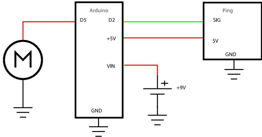
Figure 3-44. Connection diagram
