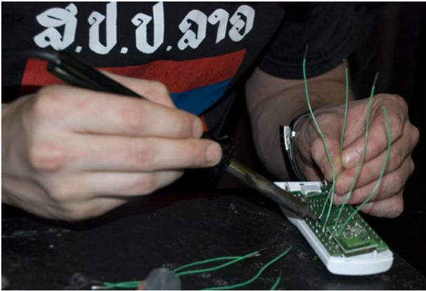
Figure 7-15. Soldering wires to the remote control switches
