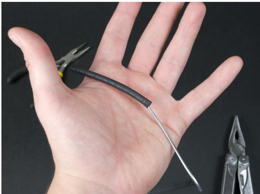
Figure 4-8. Heat-shrink tubing
