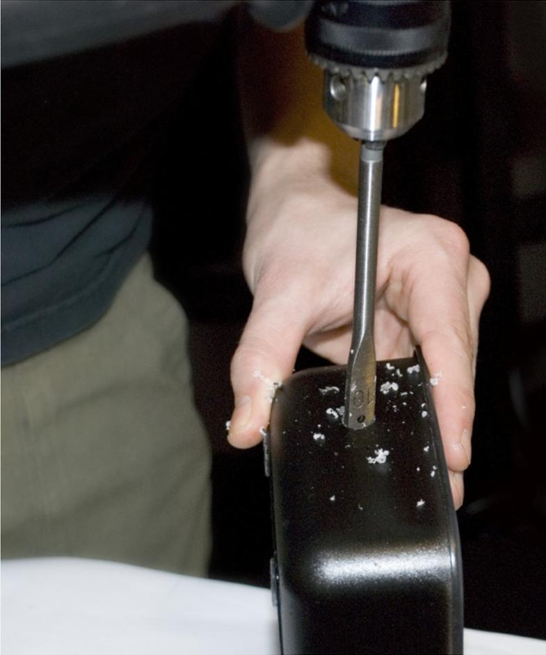
Figure 7-33. Drilling a hole for the USB cable
