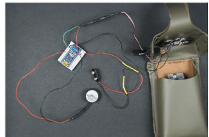
Figure 3-43. All components attached together; larger heat-shrink tubing neatly covers the individual soldered points covered by smaller heat-shrink tubing
