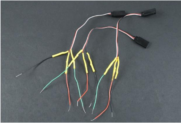
Figure 8-57. Heat-shrink tubing over the solder joints
