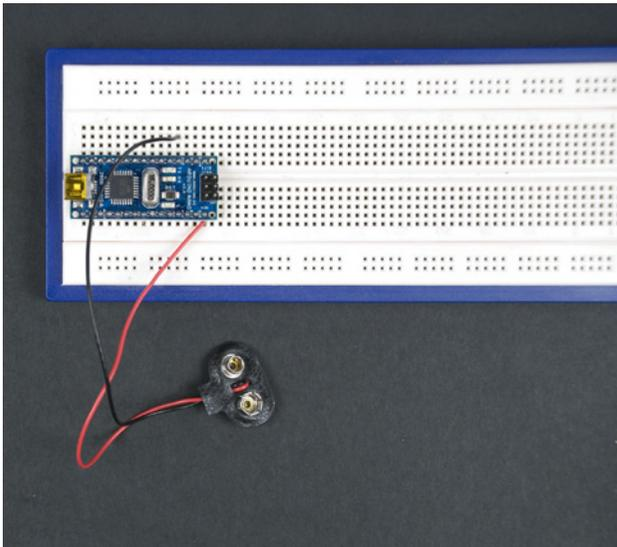
Figure 3-19. A battery connected to the Arduino
