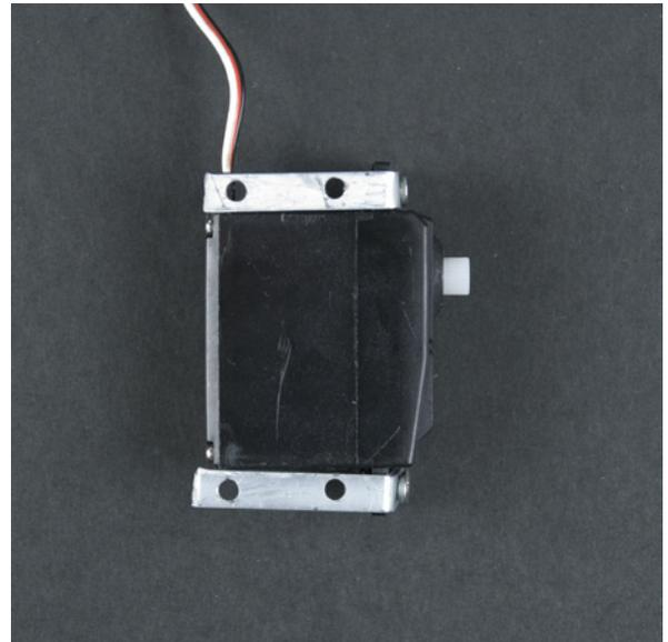
Figure 8-35. Wheel servo attachments from the side
