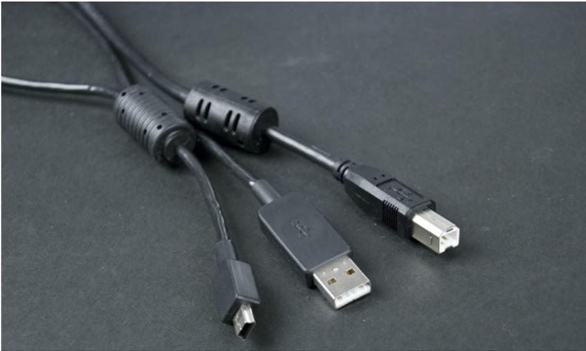
Figure 2-3. Arduino USB cables: Mini-B, USB-A, and USB-B
