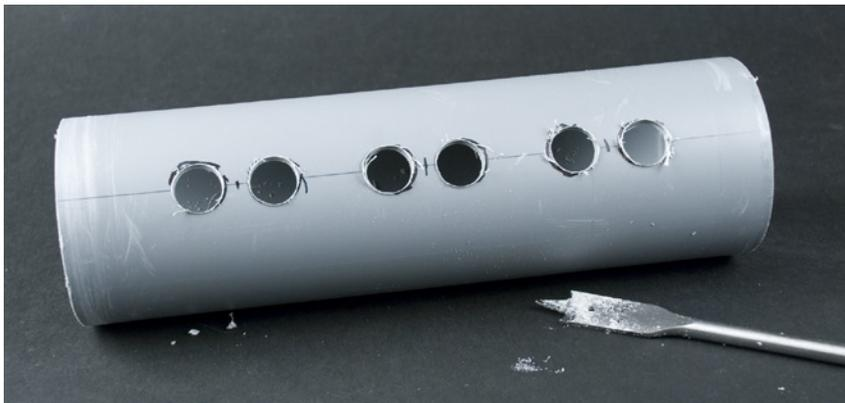
Figure 5-29. The 16mm holes for the sensors
