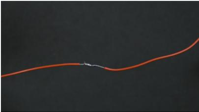
Figure 3-38. Finished soldered joint
