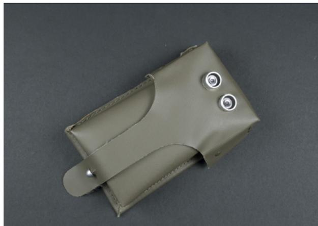
Figure 3-29. The ultrasonic sensor in place
