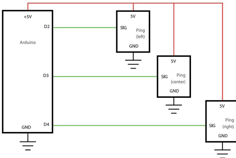
Figure 5-34. Connection diagram
