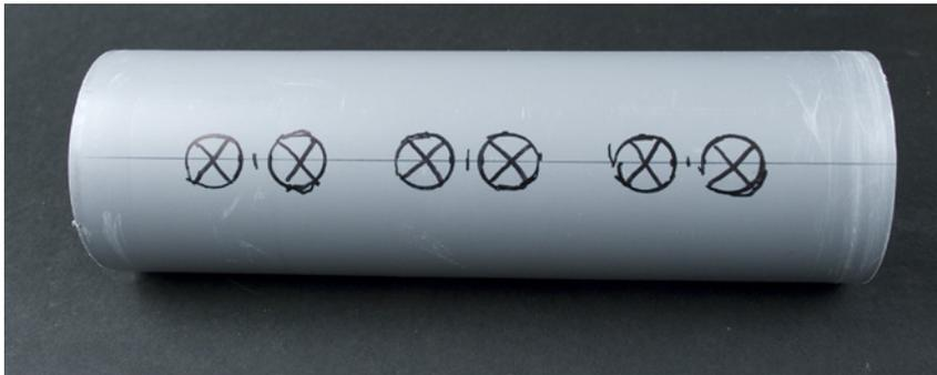
Figure 5-28. The marked ultrasonic sensor positions
