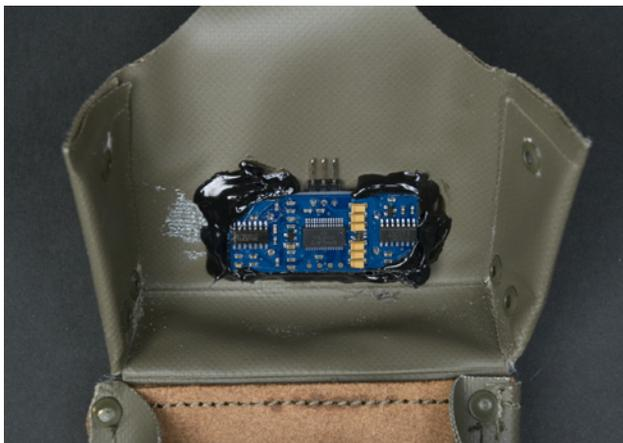
Figure 3-28. A hot-glued ultrasonic sensor
