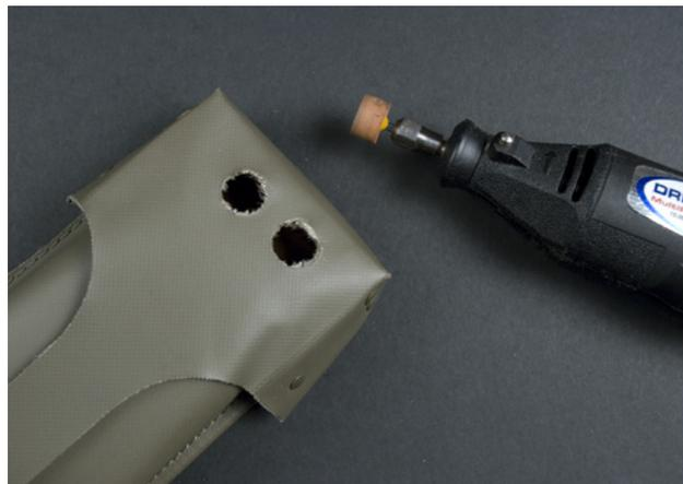
Figure 3-27. Holes created with a mini drill
