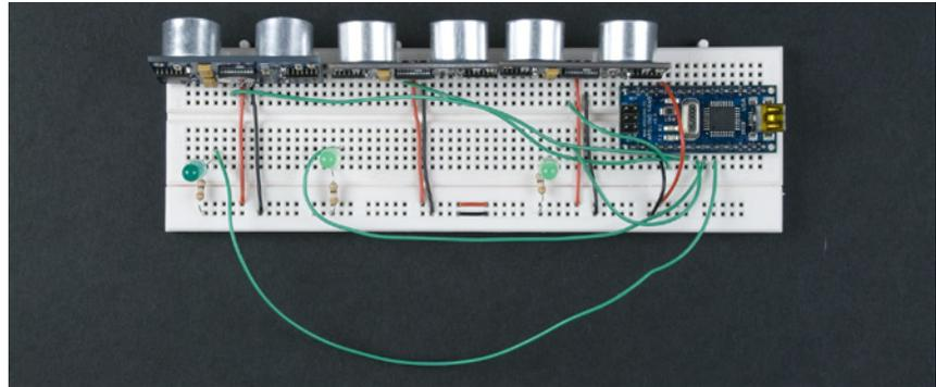
Figure 5-12. LEDs connected for testing
