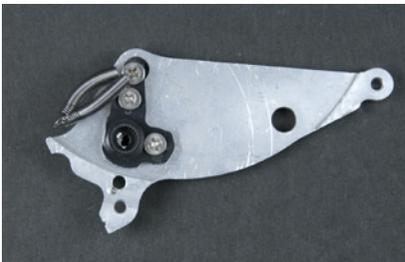
Figure 8-45. Kicker leg with servo horn attached
