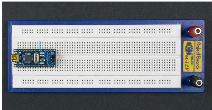
Figure 3-9. Arduino Nano on a breadboard
