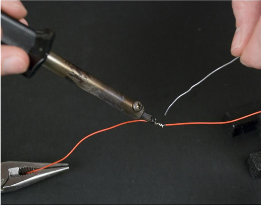
Figure 3-35. Heating the parts for approximately one second
