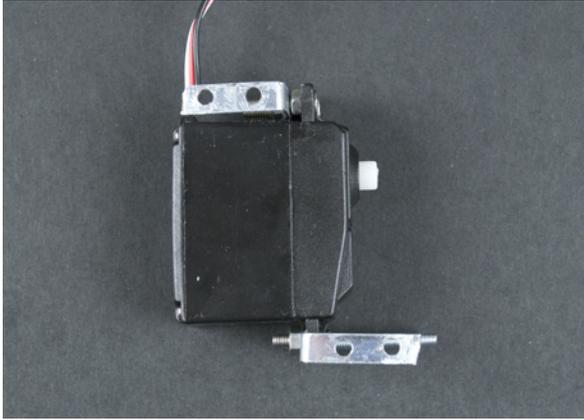
Figure 8-32. Kicker servo attachments from the side
