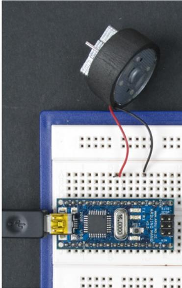
Figure 3-15. Connecting a vibration motor
