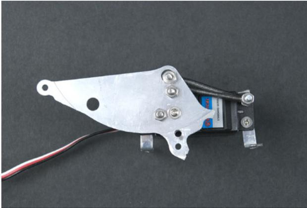
Figure 8-46. Kicker leg attached to the servo
