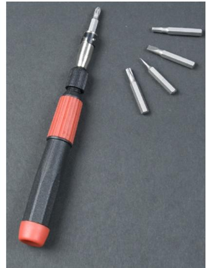
Figure 1-16. Screwdriver kit with a variety of bits
