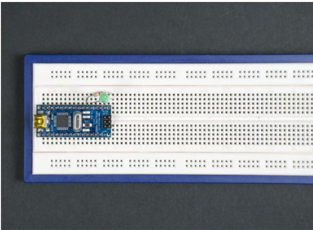
Figure 5-8. Connecting an LED to the Arduino Nano
