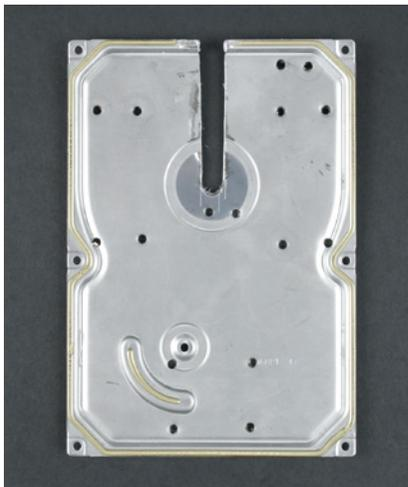
Figure 8-30. Drilled 3mm holes and notch cut for the kicker leg
