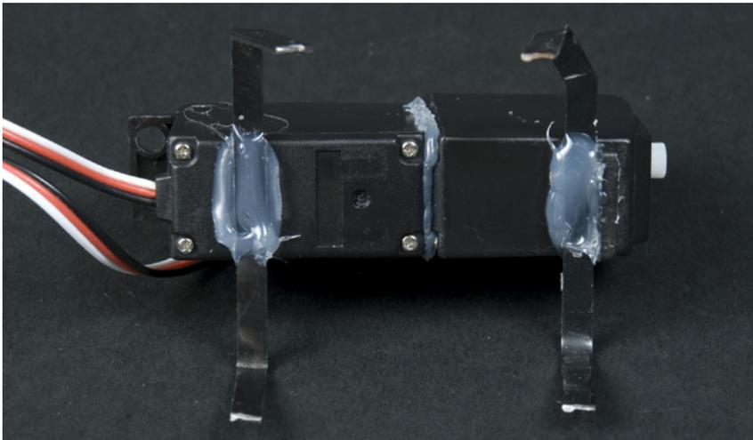
Figure 4-16. Gluing attachments
