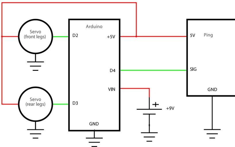
Figure 4-25. Ultrasonic sensor and servo connection schematic
