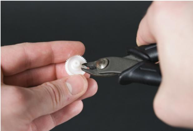
Figure 8-10. Cutting off the obstructions
