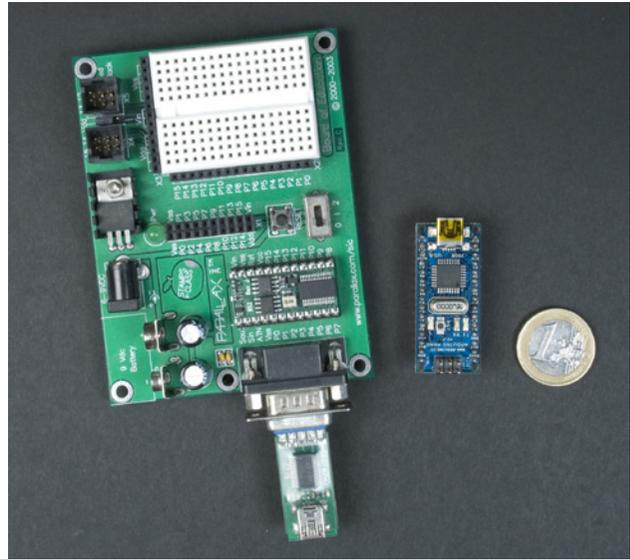
Figure 2-2. Basic Stamp (left) and Arduino Nano (right)
