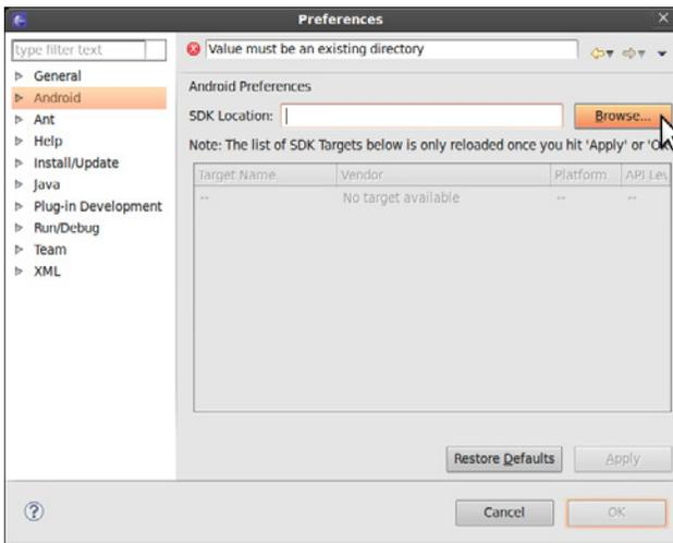
Figure 6-10. Pointing Eclipse to the Android SDK directory
