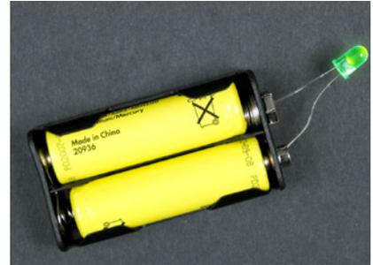
Figure 1-28. Simple closed circuit powering an LED
