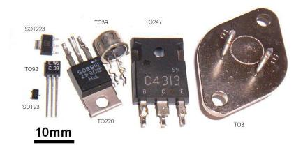
Figure 2-3. Various transistors. Source: Ulf Seifert.
