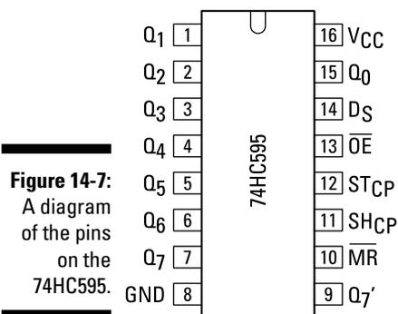
In the case of the 74HC595, there are eight output pins and, conveniently, there are also eight bits in a byte. The values are sent one bit at a time to the shift register. When the clock pin (SH\_CP) is set HIGH, all the bits shift one place forward, the last pin “shifts out” and a new pin takes its value from the
