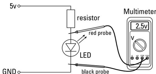
A good way to test your multimeter is to measure the voltage between the 5V pin and GND on your Arduino. Make sure that your Arduino is plugged in, and connect a jump wire to each pin to make them easier to access with your probes. Place the red voltage probe on the 5V wire and the black common probe on the GND wire. This should return a value of 5V on the screen of your multimeter and prove that your Arduino is supplying 5 volts as expected.
