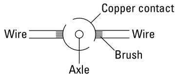
With a freely spinning coil in place on an axle, you can affect the coil by placing two permanent bar magnets near it. As shown in Figure 8-2, the magnets are placed on either side of the coil, with different poles on each side. If you put electrical current across the coil, you give it a polarity — either north or south, as with conventional bar magnets. If the coil is north, it is repelled by the north bar magnet and attracted by the south bar magnet.
