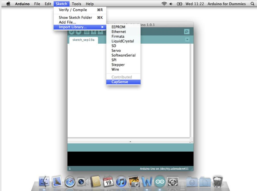
The easiest way to make a capacitive sensor is to use the CapSense library by Paul Badger. By using the CapSense library (I explain how in the “Getting the CapSense Library” sidebar), you can do away with mechanical switches altogether and replace them with highly robust capacitive touch sensors or capacitive presence detectors.
