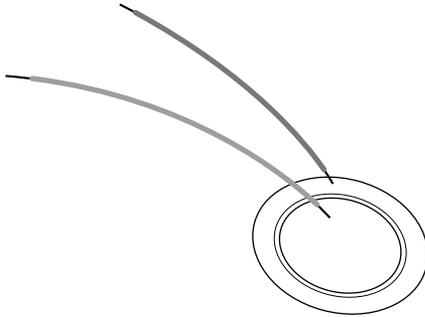
Connect the piezo buzzer to the breadboard and use a set of jump wires to connect it to digital pin 8 on one side and ground on the other. Some piezos have a polarity, so make sure that you connect the positive (+) to pin 9 and the negative (-) to GND. Other piezos don't have a polarity, so if you see no symbols, don't worry. The piezo circuit is shown in Figure 8-16, and the circuit diagram appears in 8-17.
