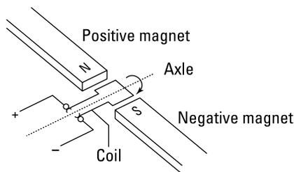
If you look at the brush again, you realize that something else happens when the coil does a half rotation: the polarity flips. When this happens, the cycle starts again and the north coil becomes south and is pushed away by the south magnet back to north again. Because of the momentum produced when the coil is repelled, this movement continues in the same direction while sufficient power exists.
