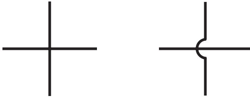
Figure 4-8: Nonconnecting crossed wires
