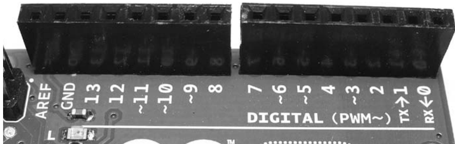
Figure 2-5: The digital input/output pins
