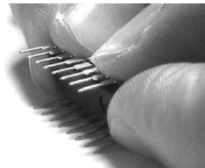
Figure 11-12: Bending the microcontroller pins
