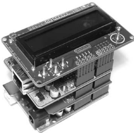
Figure 8-4: Three stacked shields with an Arduino Uno
