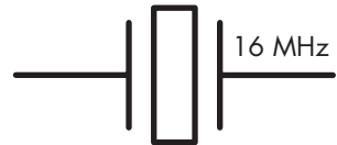
Figure 11-4: Crystal oscillator schematic symbol
