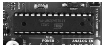
Figure 11-13: Correct orientation of the microcontroller in an Arduino
