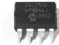
Figure 17-2: Microchip Technology's 24LC512 EEPROM
