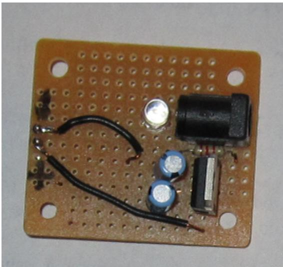
*Figure B-1. A small voltage regulator circuit.*
