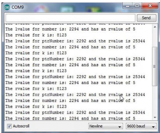
*Figure 8-5. Sample run of simple pointer program.*
