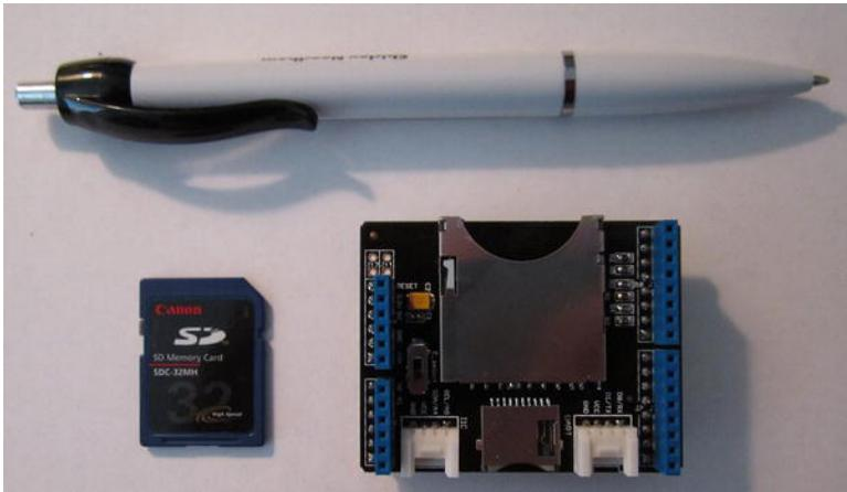
**Figure 10-8.** An SD card and shield.
