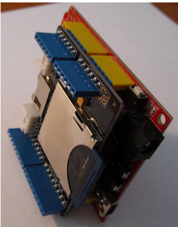
**Figure 10-9.** Stacked SD shield and board. (Shield and mc board courtesy of Seeed Studio.)
