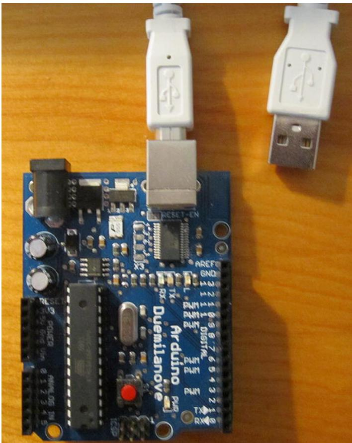
Figure 1-6. The µc board with USB cable attached.
