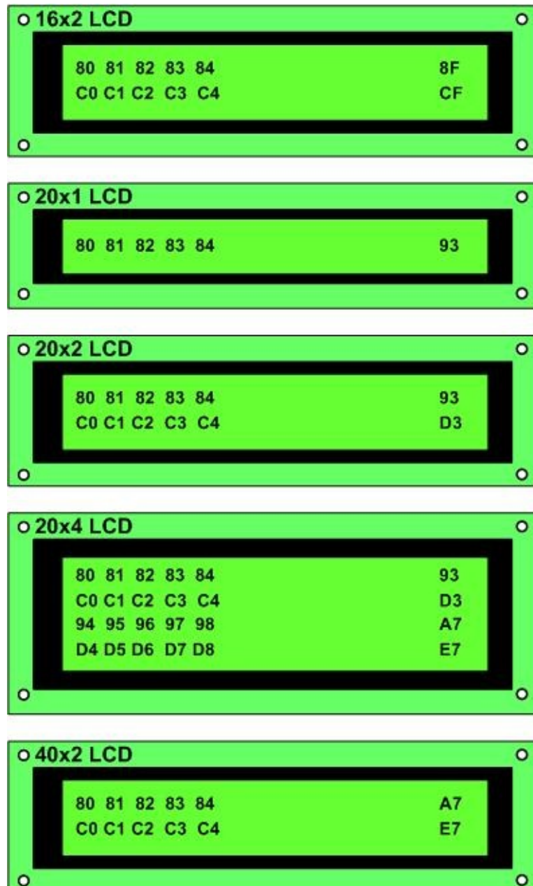
Figure 3-4: Cursor Addresses for Some LCDs
