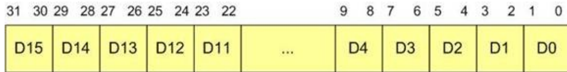
Figure 15-9: c3 Domain register
