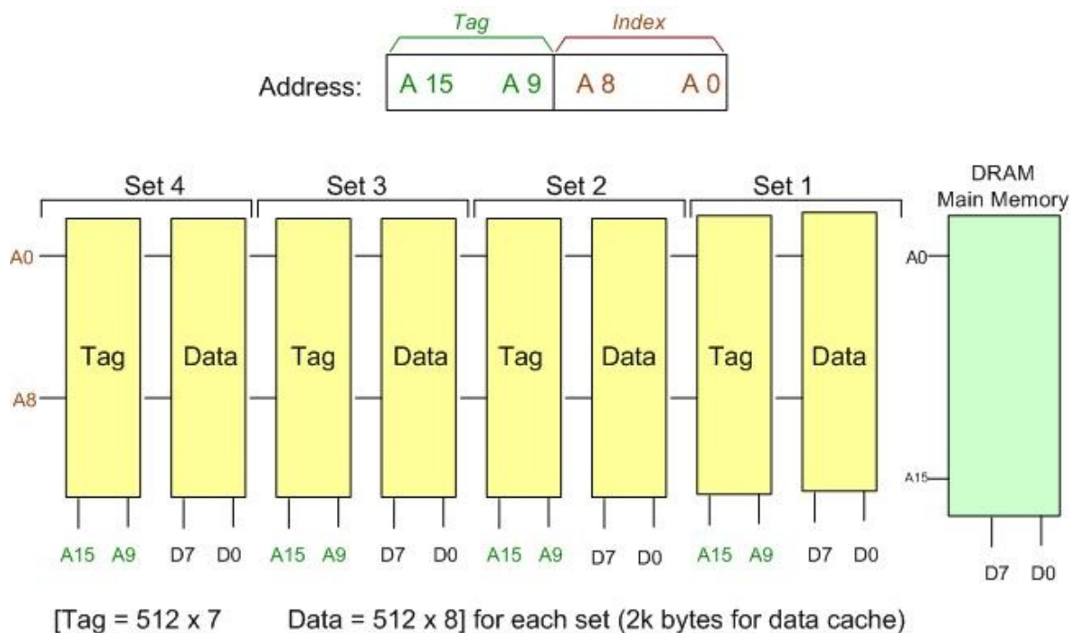
Figure 14-7: a 2KB Four-way Set Associative Cache for a 16-bit System
