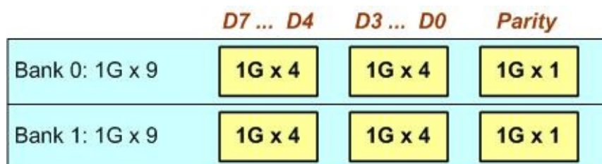
Figure 13-14: A Possible Memory Configuration for 2G DRAM
