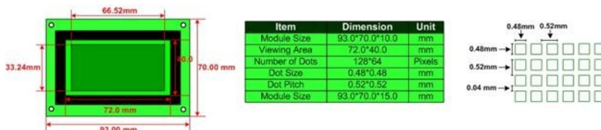
Figure 12-4: Mechanical specifications of a GDM12864 128x64 LCD
