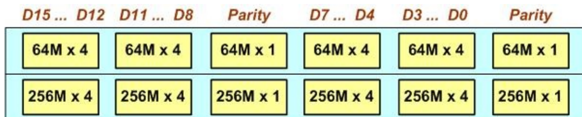
Figure 13-3: DRAM Banks for 16-bit systems
