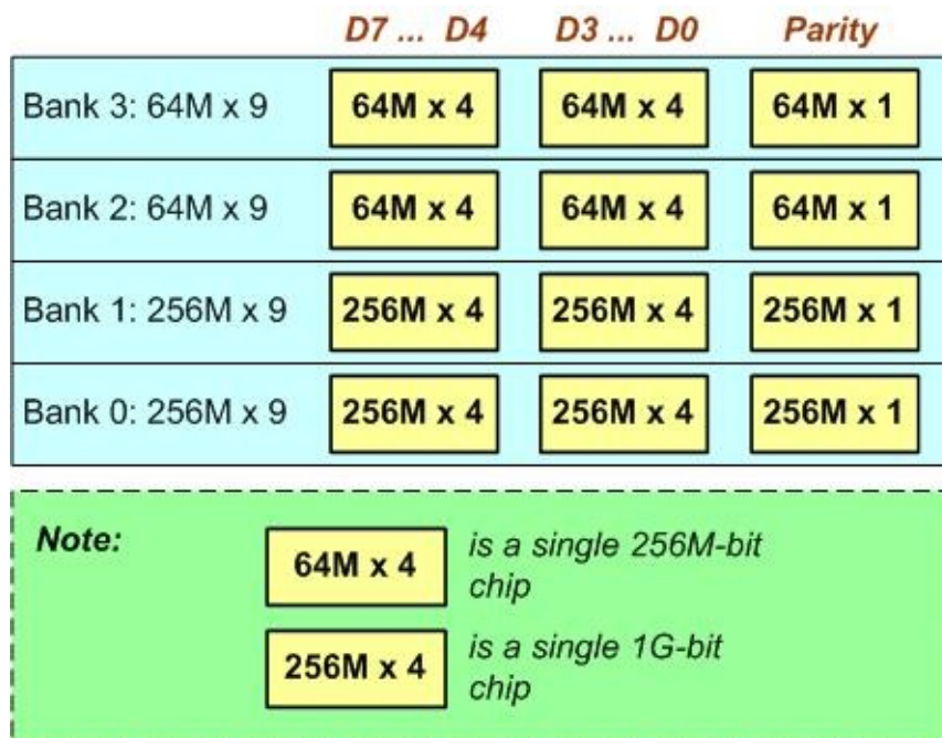
Figure 13-2: A Possible Memory Configuration for 640M DRAM
