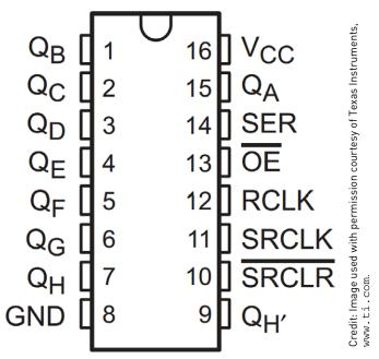
Figure 7-2: Shift register pin-out diagram
