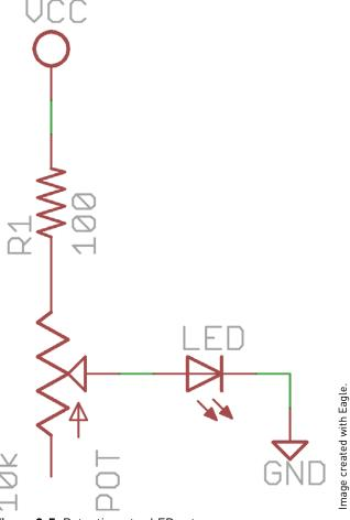
Figure 9-5: Potentiometer LED setup
