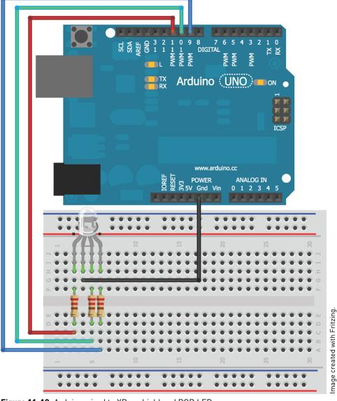
Figure 11-18: Arduino wired to XBee shield and RGB LED
