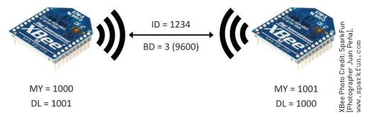
Figure 11-7: XBee point-to-point system
