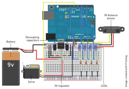
Figure 4-14: Sweeping distance sensor wiring diagram
