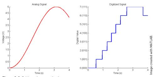
Figure 3-2: 3-bit analog quantization
