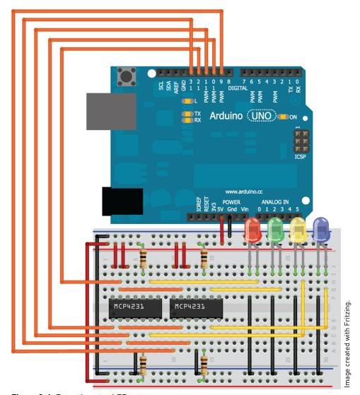
Figure 9-6: Potentiometer LED setup
