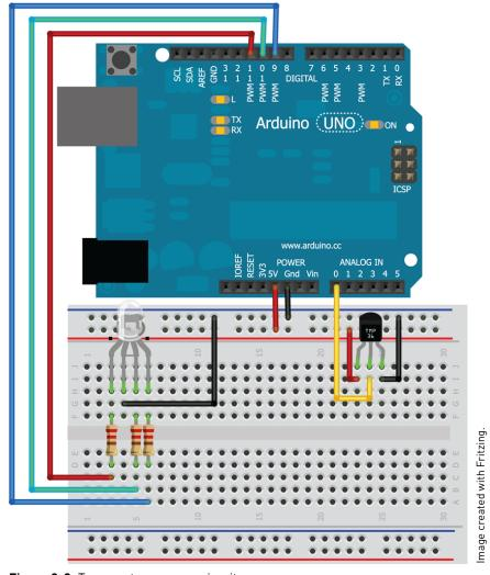
Figure 3-8: Temperature sensor circuit
