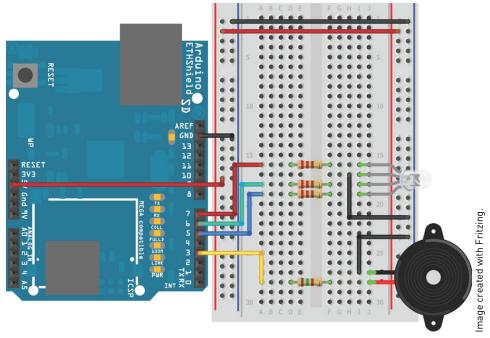
Figure 14-2: Arduino server wired to RGB LED and speaker
