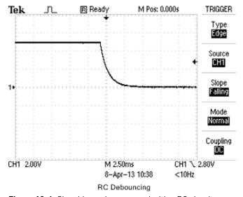
Figure 12-4: Signal bouncing removed with a RC circuit
