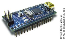
Figure 1-7: The Arduino Nano
