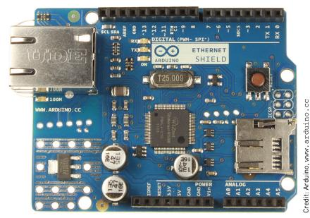
Figure 13-9: Arduino Ethernet SD shield
