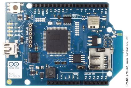
Figure 13-10: Arduino Wi-Fi SD shield
