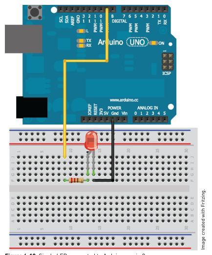
Figure 6-10: Single LED connected to Arduino on pin 9
