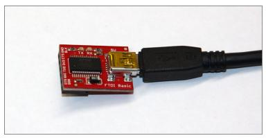
Figure 6-4: SparkFun FTDI adapter board
