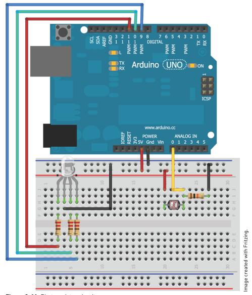
Figure 3-11: Photoresistor circuit
