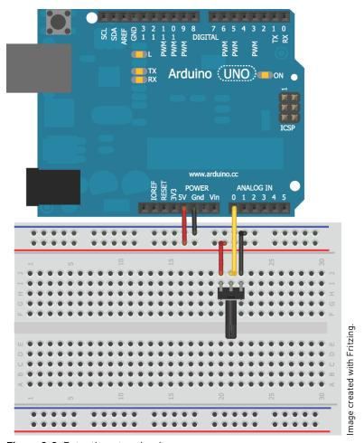
Figure 3-3: Potentiometer circuit
