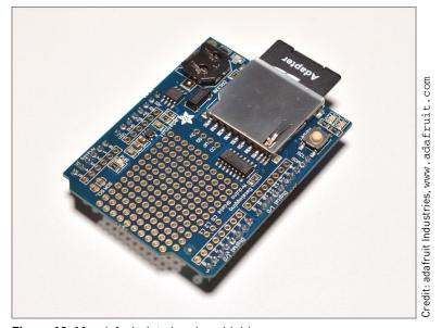
Figure 13-11: adafruit data logging shield
