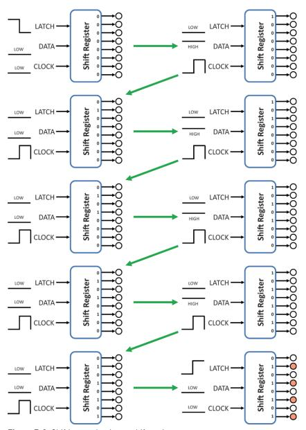
Figure 7-3: Shifting a value into a shift register
