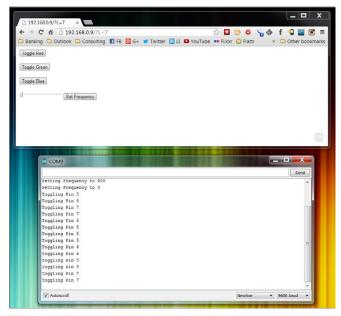
Figure 14-5: Arduino control web page and serial debugging
