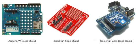
Figure 11-4: Various XBee shields
