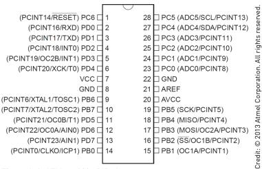
Figure A-3: ATMega 328p DIP pin-out
