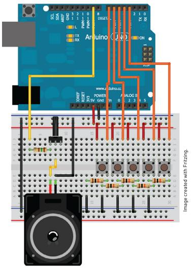
Figure 5-6: Micro piano wiring diagram
