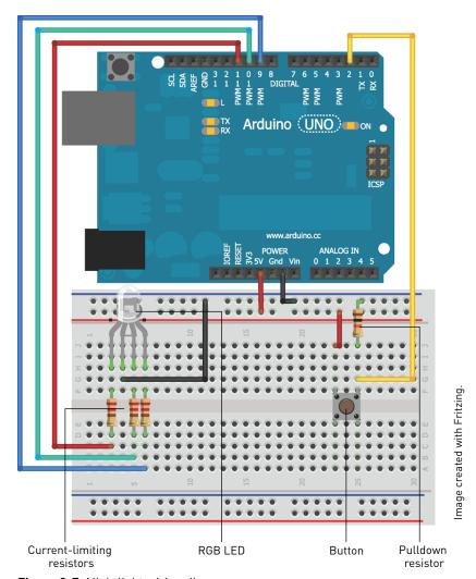
Figure 2-7: Nightlight wiring diagram
