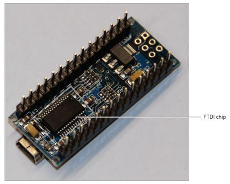
Figure 6-2: Arduino Nano with integrated FTDI chip shown
