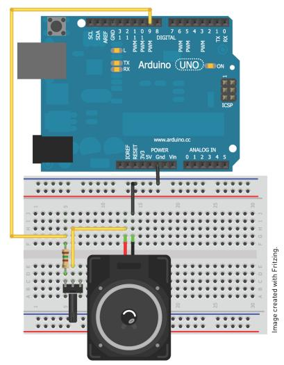
Figure 5-5: Speaker wiring diagram
