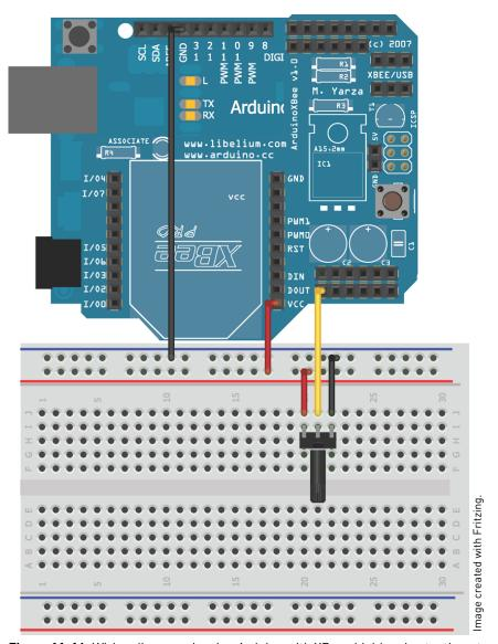
Figure 11-16: Wiring diagram showing Arduino with XBee shield and potentiometer
