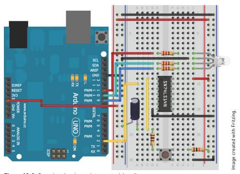
Figure 12-8: Complete hardware interrupt wiring diagram
