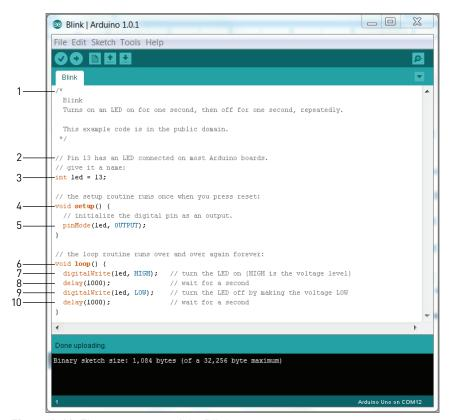
Figure 1-13: The components of the Blink program
