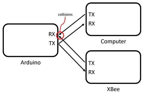
Figure 11-5: Colliding UART communication lines
