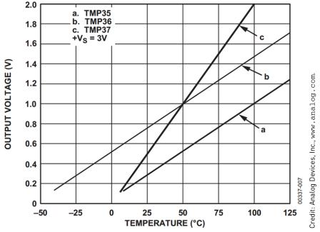
Figure 3-7: Voltage to Temperature Correlation
