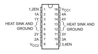
Figure 4-6: H-bridge pin-out and logic table
