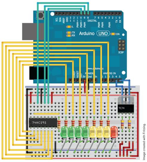
**Figure 8-8:** I<sup>2</sup>C temperature sensor with shift register bar graph (part of the TC74 has been made transparent so you can see the wires that connect behind it)
