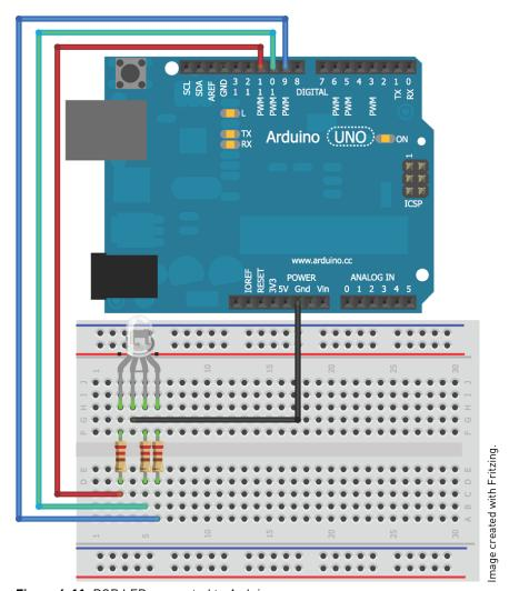
Figure 6-11: RGB LED connected to Arduino
