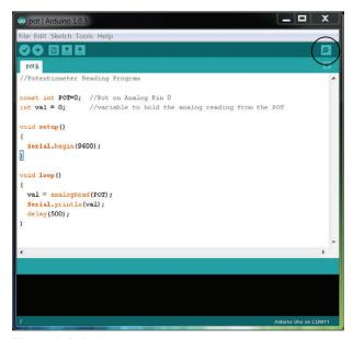
Figure 3-5: Serial monitor button
