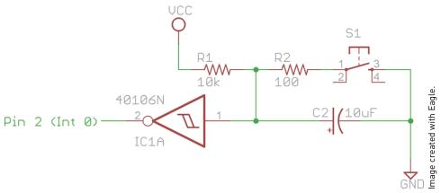
Figure 12-6: Final step for creating a debounce circuit: adding an inverting Schmitt trigger
