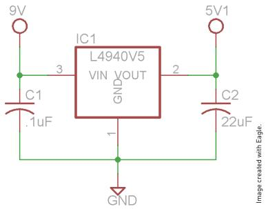
Figure 4-11: 5V Linear regulator schematic
