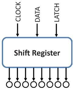
Figure 7-1: Shift register input/output diagram
