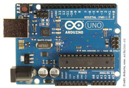
Figure 1-3: The Arduino Uno
