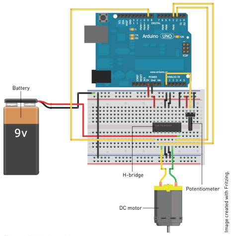
Figure 4-7: H-bridge wiring diagram
