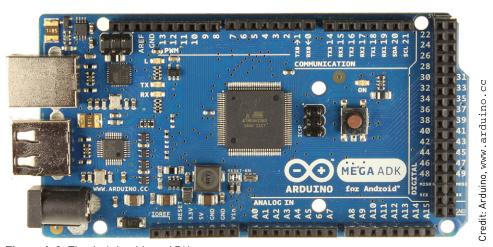
Figure 1-8: The Arduino Mega ADK
