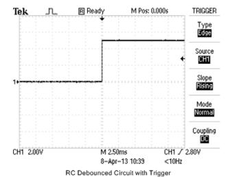
Figure 12-7: Final output of debounce circuit
