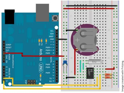
Figure 13-19: Real-time clock circuit assembled on breadboard
