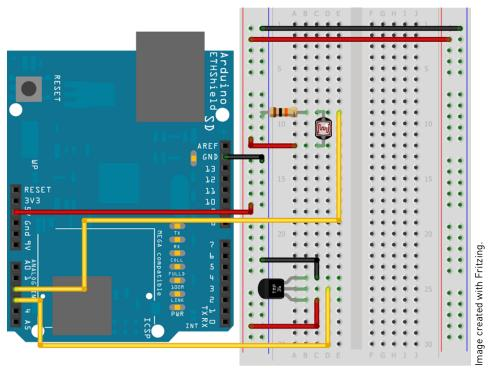
Figure 14-10: Adding a TMP36 temperature sensor
