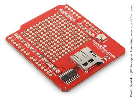
Figure 13-12: SparkFun MicroSD shield
