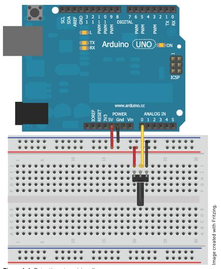
Figure 6-6: Potentiometer wiring diagram
