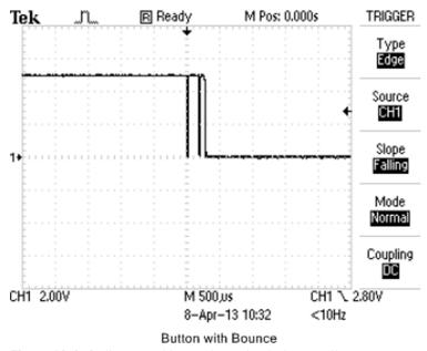
Figure 12-2: Ordinary pushbutton bouncing before settling
