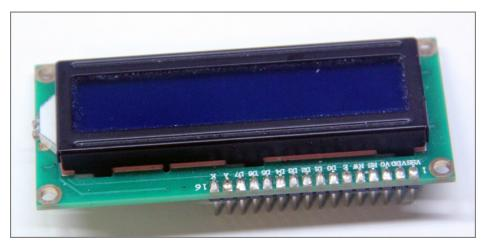
Figure 10-1: LCD with Headers soldered on
