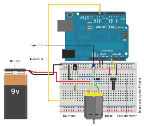
Figure 4-4: Adding a potentiometer
