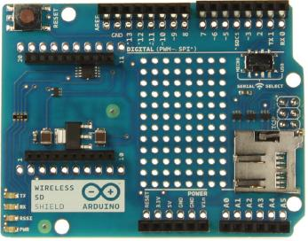
Figure 13-8: Arduino Wireless SD shield
