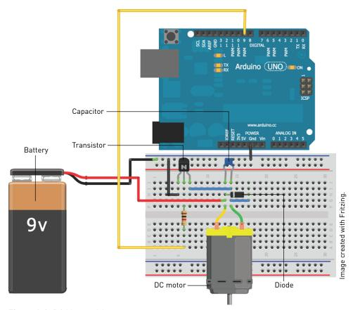
Figure 4-3: DC Motor wiring
