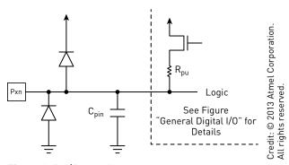
Figure A-2: I/O pins diagram
