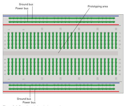
Figure 2-1: Breadboard electrical connections
