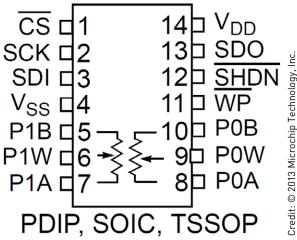
Figure 9-2: MCP4231 Pin-out diagram
