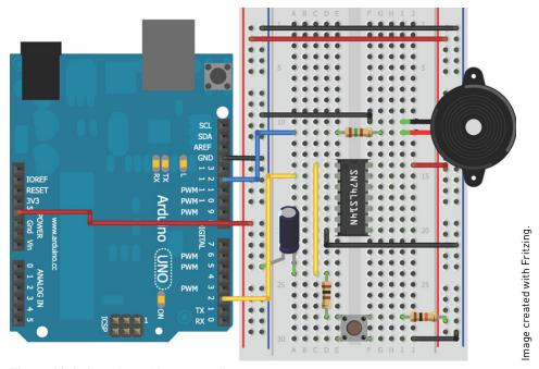
Figure 12-9: Sound machine wiring diagram
