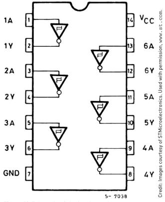
Figure 12-5: Inverting Schmitt trigger pin-out
