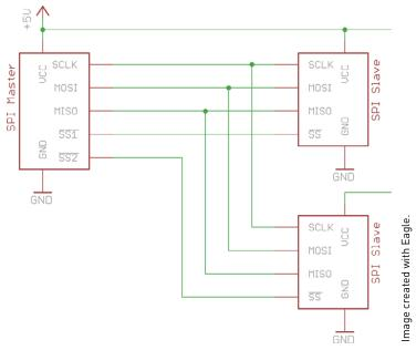
Figure 9-1: SPI reference hardware configuration
