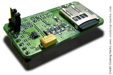
Figure 13-7: Cooking Hacks MicroSD shield
