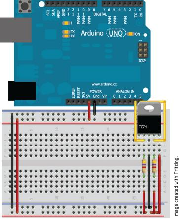
Figure 8-4: Temperature sensor
