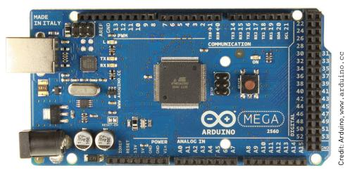
Figure 1-5: The Arduino Mega 2560
