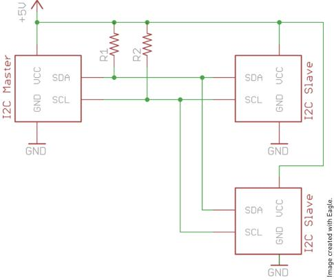
Figure 8-1: I<sup>2</sup>C reference hardware configuration
