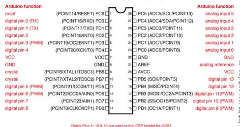
Figure A-4: Arduino ATMega Pin Mapping
