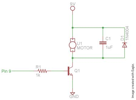
Figure 4-1: DC motor control schematic
