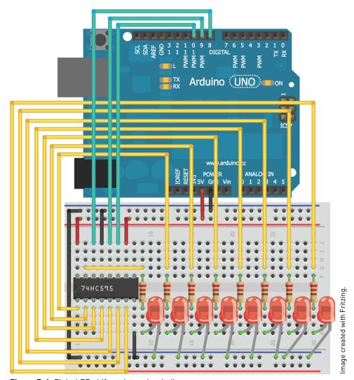
Figure 7-4: Eight LED shift register circuit diagram
