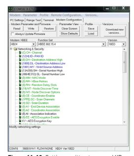
Figure 11-12: Settings written to second XBee
