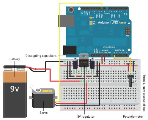
Figure 4-12: Servo experiment wiring diagram
