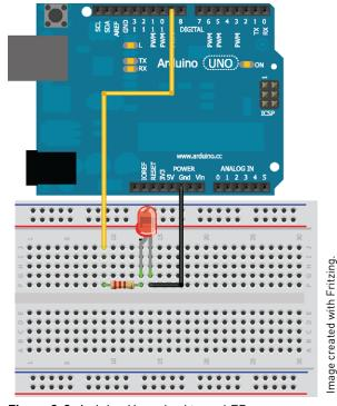
Figure 2-2: Arduino Uno wired to an LED
