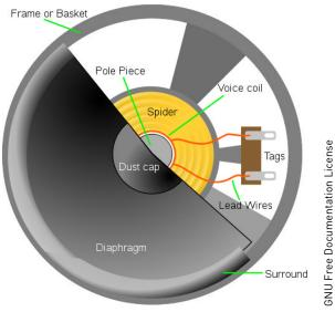
Figure 5-2: Speaker cross section
