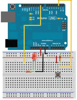
Figure 2-5: Wiring an Arduino to a button and an LED
