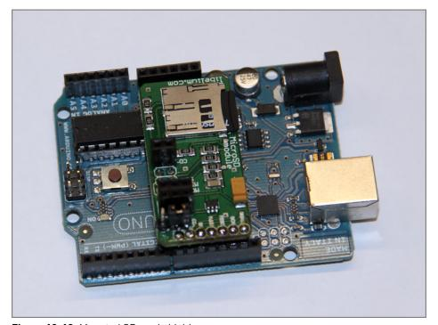
Figure 13-13: Mounted SD card shield
