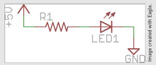
Figure 2-3: Simple LED circuit
