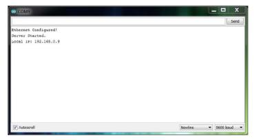
Figure 14-4: DHCP IP acquisition confirmation via serial
