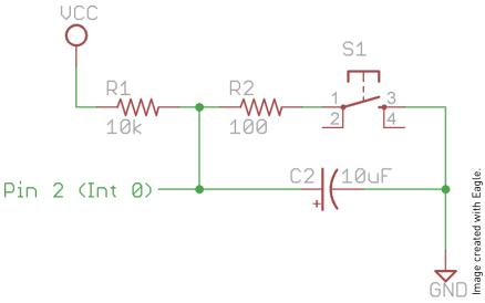
Figure 12-3: Creating a debounce circuit: adding a capacitor and a resistor
