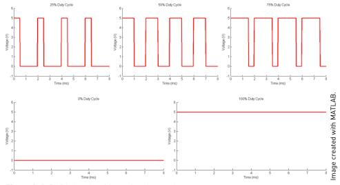
Figure 2-4: PWM signals with varying duty cycles
