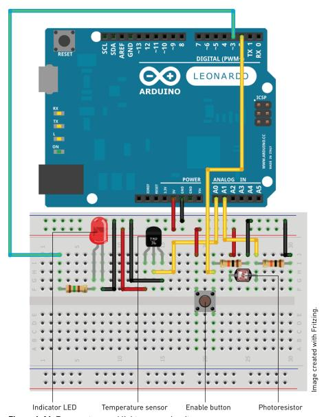
Figure 6-16: Temperature and light sensor circuit
