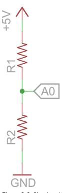
Figure 3-9: Simple voltage divider circuit
