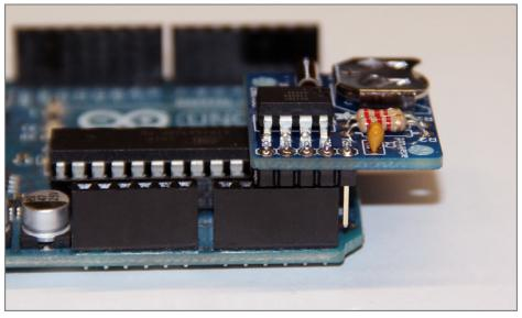
Figure 13-18: Real-time clock breakout mounted on an Arduino
