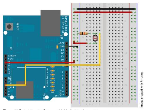
Figure 14-7: Arduino with Ethernet shield wired to photoresistor
