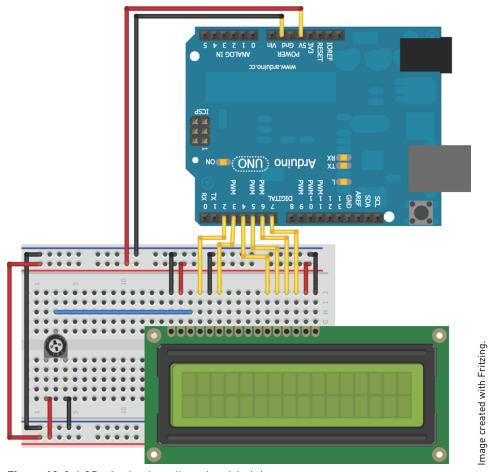
Figure 10-2: LCD wired to breadboard and Arduino
