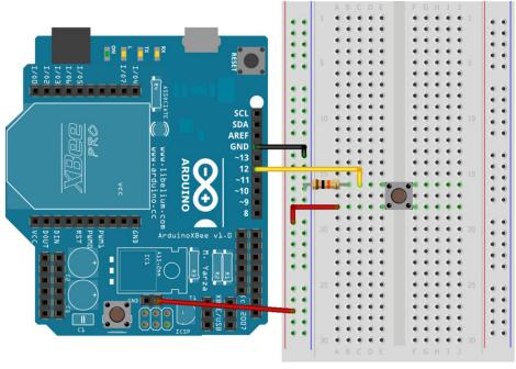
Figure 11-20: Wireless doorbell transmitter
