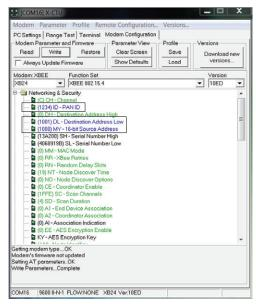
Figure 11-11: Settings written to XBee
