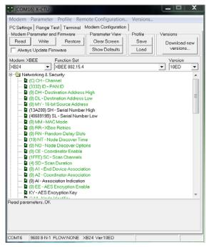
Figure 11-10: X-CTU modem configuration
