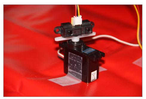
Figure 4-13: IR distance sensor mounted to the servo
