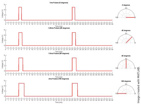
Figure 4-10: Servo motor timing diagram
