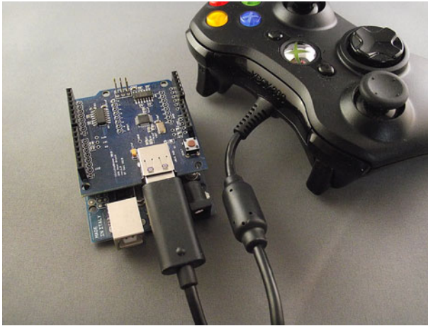
Figure 9.14 Xbox controller connected to USB Host Shield and Arduino
