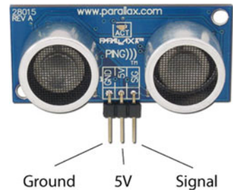
Figure 6.3 The Parallax Ping, an ultrasonic sensor
