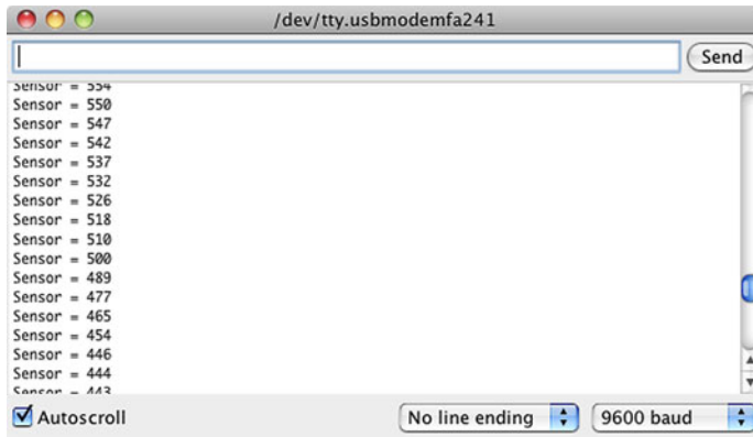
Figure 3.5 Output displayed as the potentiometer is rotated
