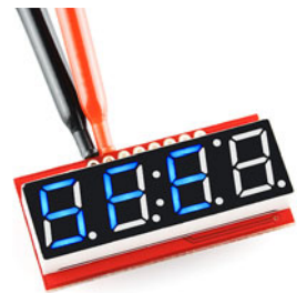
Figure 11.16 The SparkFun 7-segment serial display
