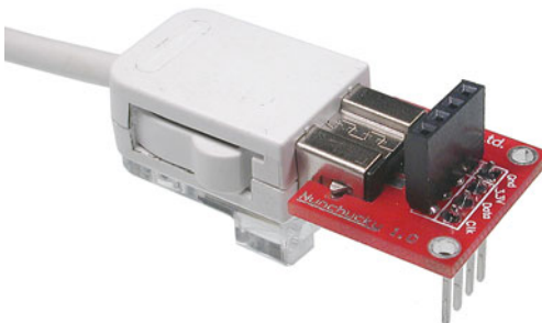
Figure 9.7 NunChucky breakout board from Solarbotics
