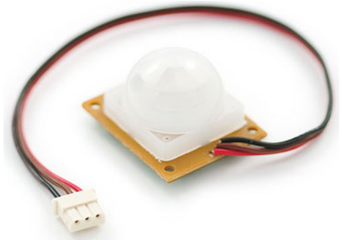
Figure 6.9 The Parallax PIR sensor
