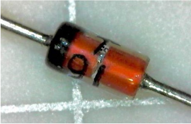
Figure 6-11. 1N914 diode to be tested
