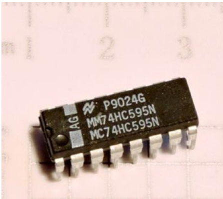
Figure 10-1. 74HC595 serial in, parallel out shift register
