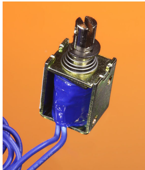
Figure 21-1. A small 12VDC solenoid.
