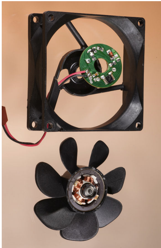
Figure 22-10. A typical brushless DC cooling fan uses stationary coils, with permanent magnets rotating around them.
